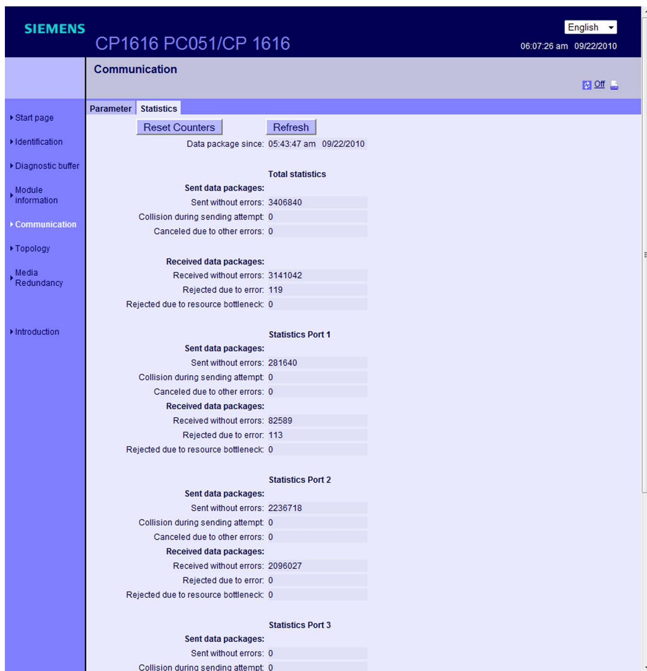
Figure 4-13 Characteristic data of data transfer
