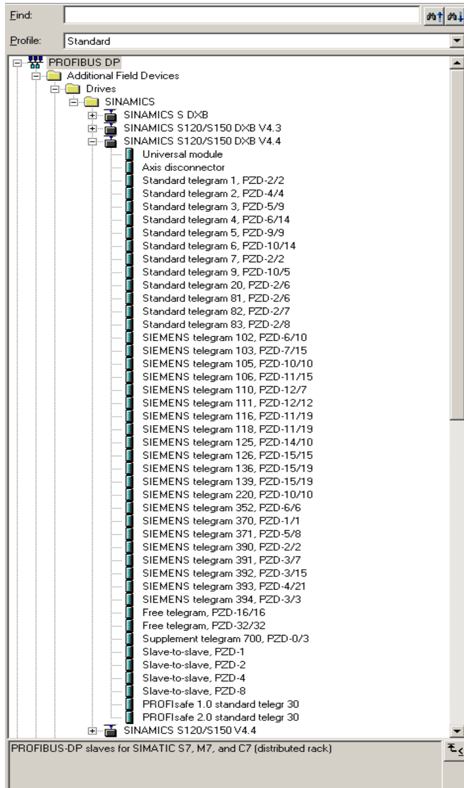
Figure 10-40 Hardware catalog of the generic station description file with slave-to-slave communication functionality
