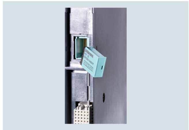
Plugging the C-plug into the rear of the CP 443-1 Advanced
