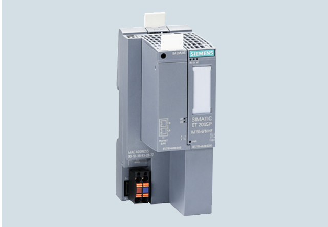
IM 155-6PN High Feature interface module, with reference ID label
