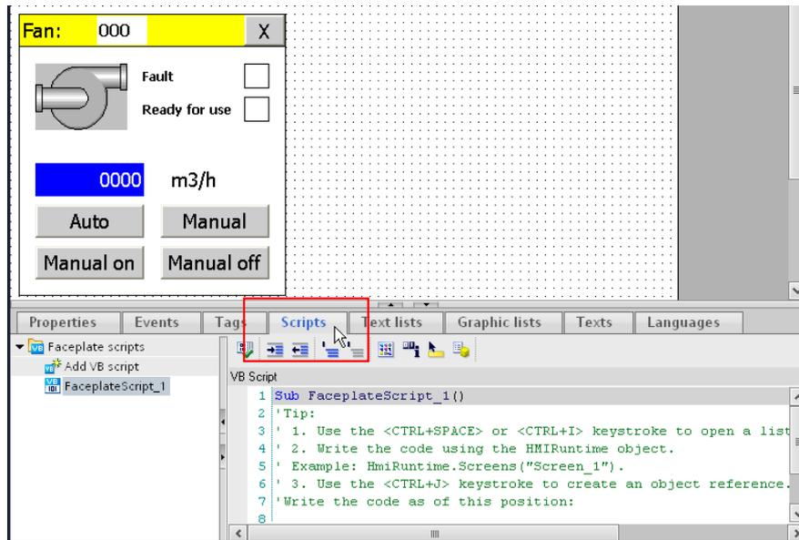
The "Scripts" tab contains scripts which are only available within the faceplate. In the script you call up the system functions or program new functions, e.g. for converting values. Programming is performed in VB script code.
