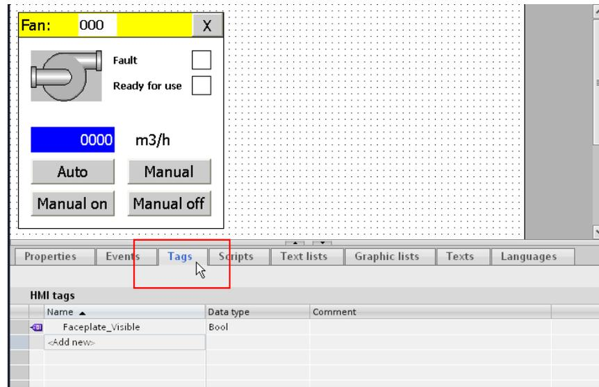
The "Tags" tab contains tags which are only available within the faceplate. The tags are connected directly to the objects contained in the faceplate.
