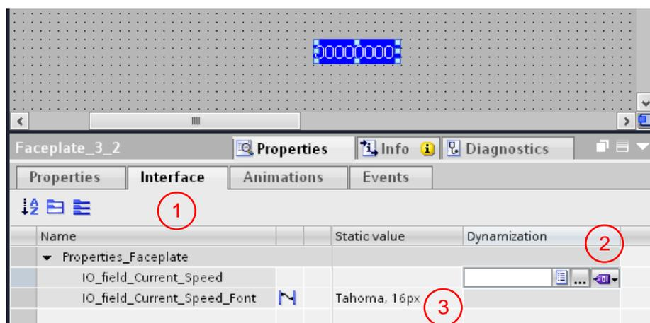
In the "Interface" tab (1) you see the two configured properties of the faceplate. A tag can be assigned to the "dynamic" interface (2). Only a fixed value can be assigned to the "static" interface (3).
