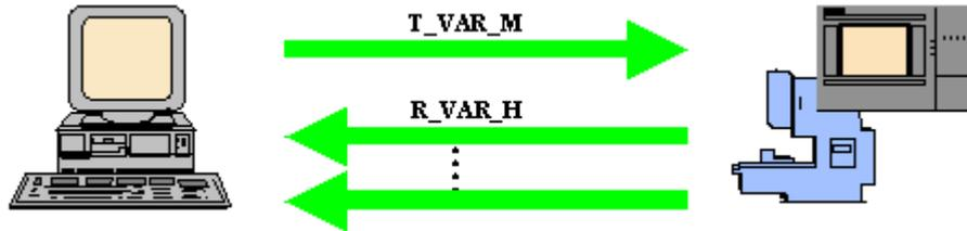
When the HTML page is loaded, the RPC **T\_VAR\_M()** is sent to RPC SINUMERIK via a VBScript function. With this RPC, the current values of the variables in the set: **"Set01"** are requested. This data is immediately supplied by RPC SINUMERIK with the RPC: **R\_VAR\_H()**.
