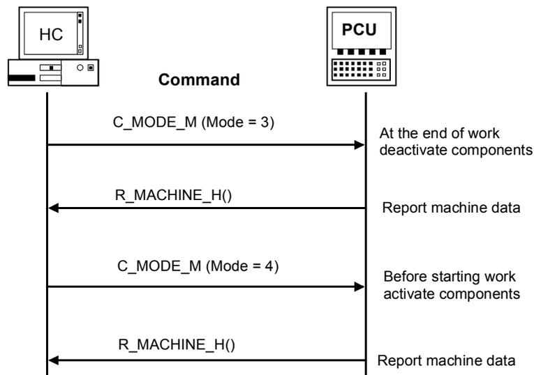
Fig. 5-23 End of work, initiated by the host computer
