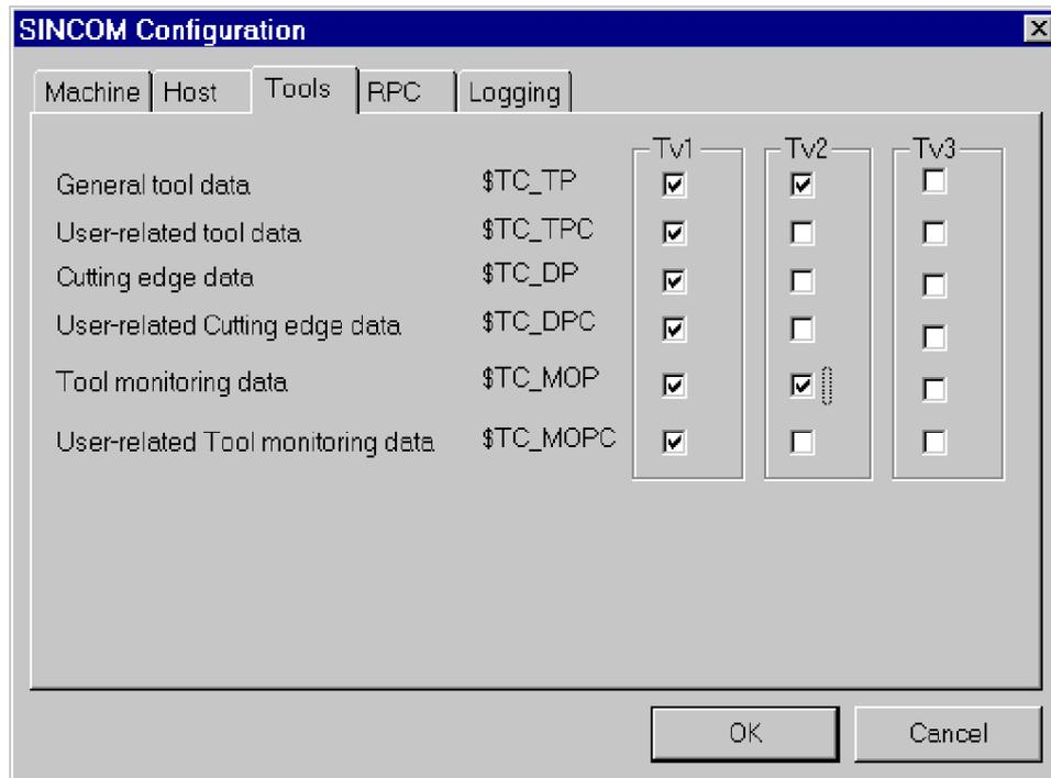
Fig. 5-3 Configuration program: Tools tab
