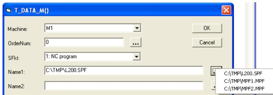
With the "OK" button you can send the RPC. All RPCs sent are traced. The traces are output to the screen in the main window of the RPC SINUMERIK Test application and to the logfile: RpcSinumerikTest.LOG. For every RPC sent, the return value is also logged and displayed in the status line (Ret=0). The meaning of the return value is described in Subsection: "10.3.6 Error handling".
