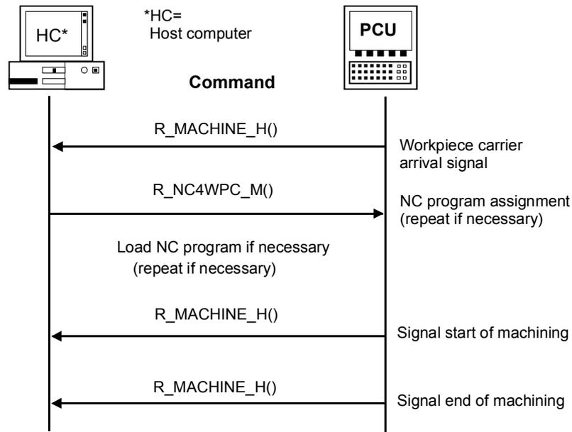
Fig. 5-1 Production dialog, normal execution, no errors
