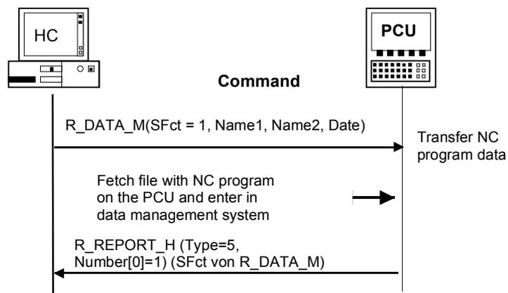
Fig. 5-6 Transfer NC program, initiated by host computer
