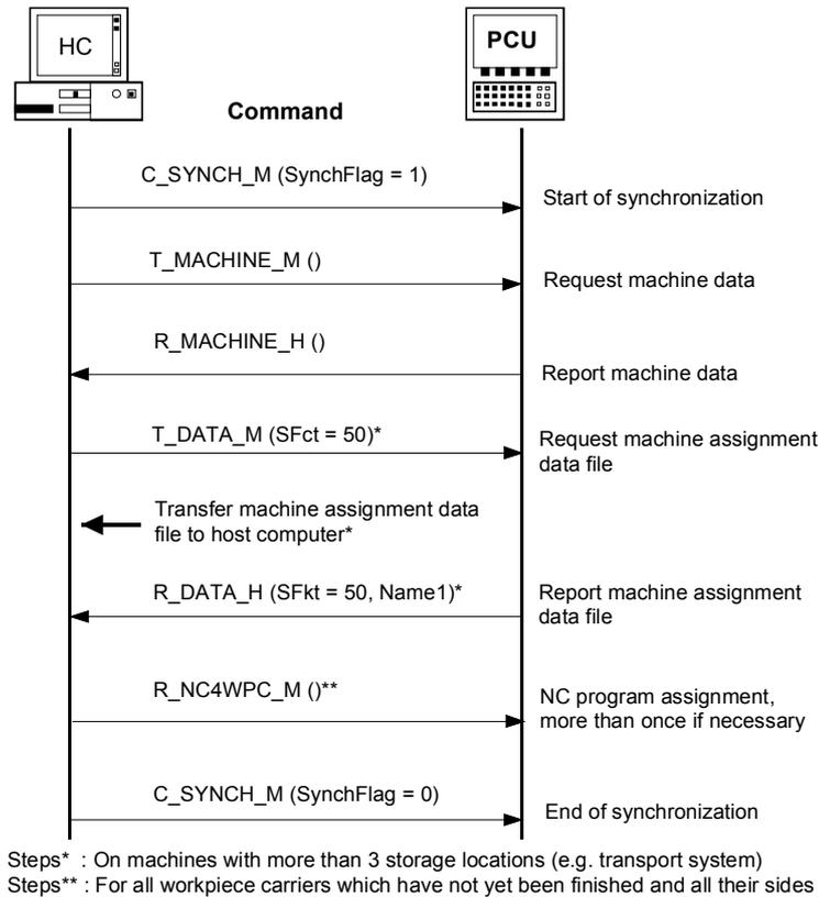
Fig. 5-24 Synchronization, initiated by host computer
