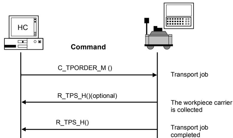
Fig. 8-1 Transport dialog, normal situation, no errors
