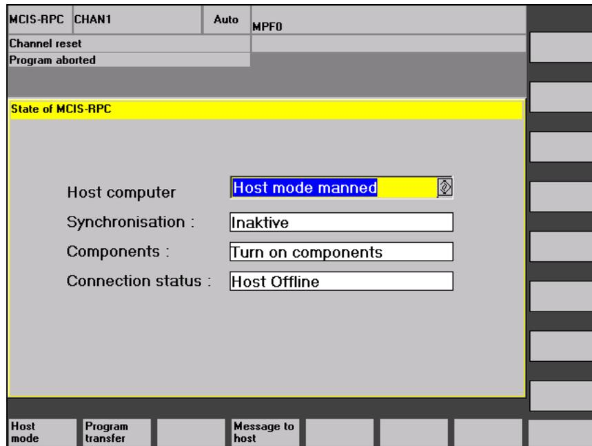
Fig. 3-1 The screen allows you to change the host computer mode
