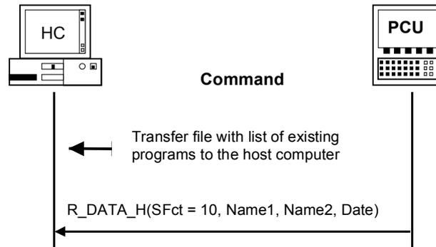
Fig. 5-12 Transfer NC program list to the host computer
