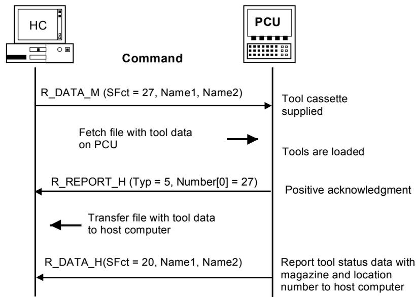
Fig. 5-18 Load tool pallet/cassette
