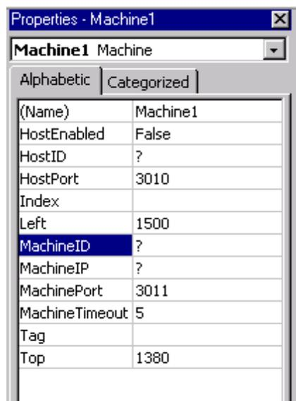
When you change the attribute: **MachineID**, the display of the OCX in the form also changes. Sending of the RPC **T\_MACHINE\_M** is triggered by clicking on the "DoRPC" button. The RPC SINUMERIK application responds with the RPC **R\_MACHINE\_H**. The response to this in the example application is a message box.
