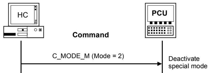
Fig. 5-22 Deactivate special mode, initiated by the host computer
