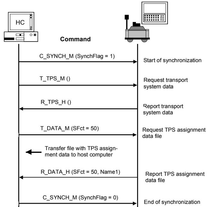
Fig. 8-2 TPS synchronization, initiated by host computer
