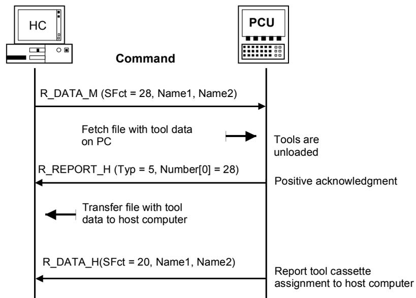
Fig. 5-19 Unload tool pallet/cassette
