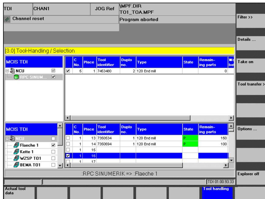
Fig. 3-8 Tool handling/selection
