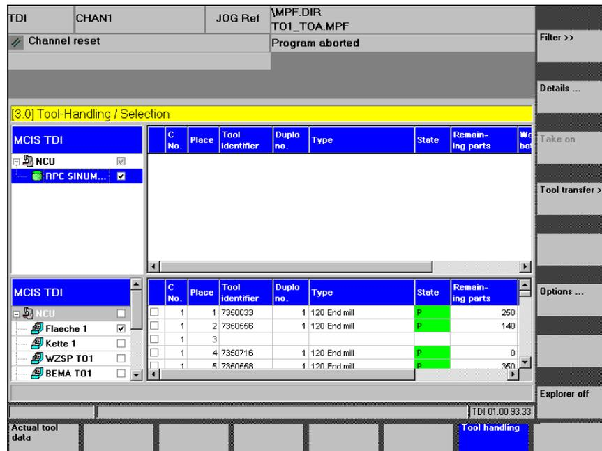
Fig. 3-11 Tool handling/filters
