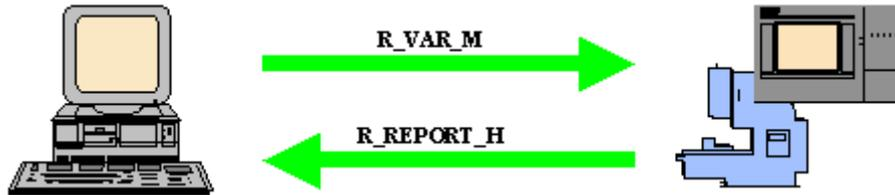
The VisualBasic application passes the data for an R parameter with the RPC: **R\_VAR\_M()** to RPC SINUMERIK. RPC SINUMERIK acknowledges the write operation with the RPC: **R\_REPORT\_H()**.
