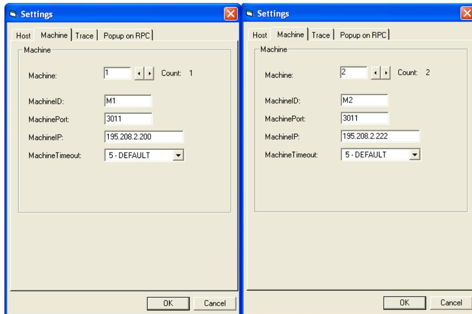
The meaning of the input fields HostEnabled and MachineTimeout corresponds to the attributes of the RPC SINUMERIK-OCX with the same names.
