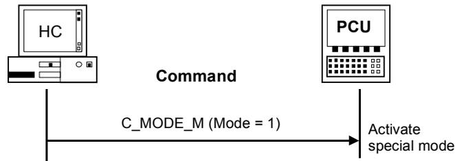
Fig. 5-21 Activate special mode, initiated by the host computer
