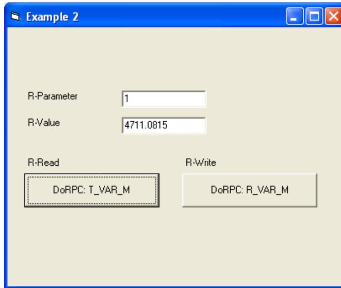
To activate the variable service of RPC SINUMERIK, at least one variable set must be defined in the file c:\add\_on\svarset.ini on the controller. Changes in this file only become effective after the next cold restart of the controller. If this is not the case, RPC SINUMERIK responds with the RPC: R\_REPRT\_H() and the error: -800.
