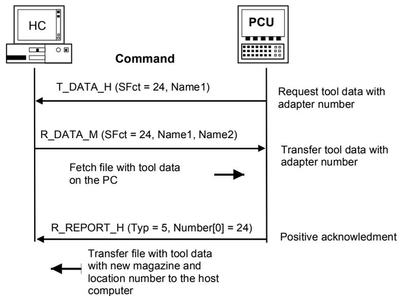
Figure 5-14 Tool data with tool adapter number (option)
