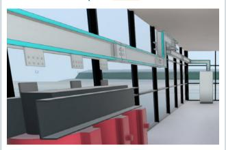
The new SIMARIS busbarplan planning tool supports simple configuration of SIVACON 8PS busbars.
