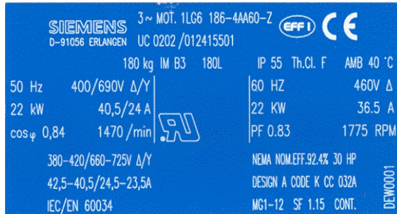
Figure 3-4: Name plate of a 22 kW motor
