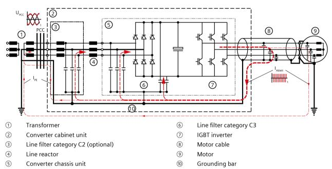
Figure 4-4 Reduction of high-frequency interference with line filters
