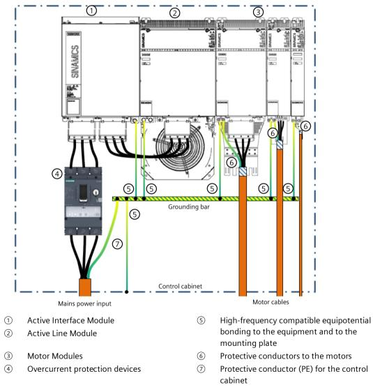
Figure 3-1 Protective connection concept, SINAMICS S120 Booksize (example)
