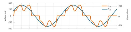
Figure 4-3 Typical progression of the input current of a three-phase converter
