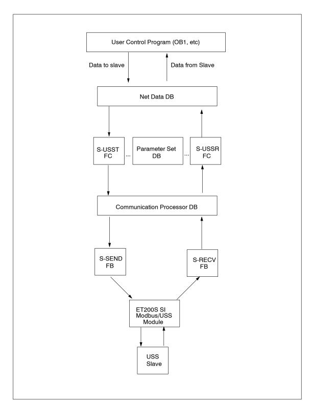
Figure 7-1 Data travel between user control program and USS slave
