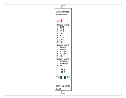
Figure 1-1 shows the ET 200S Serial Interface Modbus/USS module.
