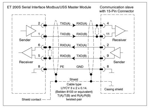
Figure 2-3 RS-422 Connecting Cable to 15-Pin Connector (1 master, 1 slave system)
