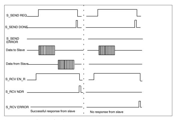
Figure 4-1 Time Sequence Chart for Modbus Request
