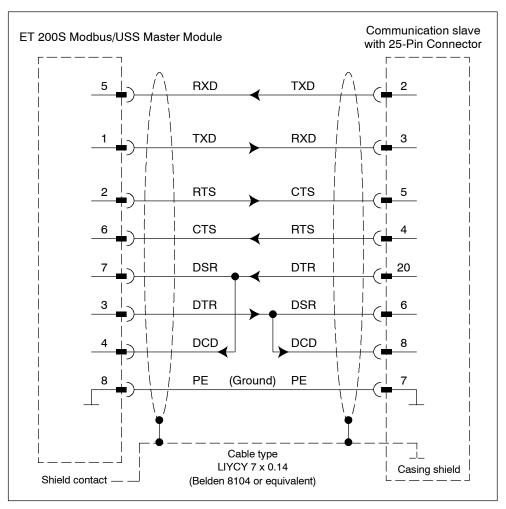
Figure 2-2 RS-232C Connecting Cable to 25-Pin Connector (1 master, 1 slave system)
