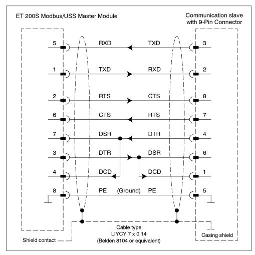
Figure 2-1 RS-232C Connecting Cable to 9-Pin Connector (1 master, 1 slave system)
