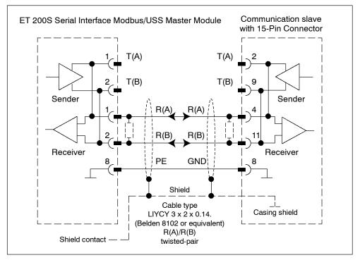
Figure 2-4 RS-485 Connecting Cable to 15-Pin Connector (1 master, 1 slave system)
