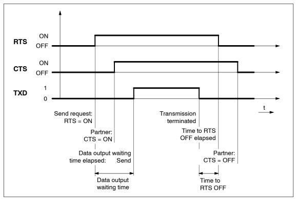
Figure 2-5 Time Diagram for Automatic Use of the RS-232C Secondary Signals
