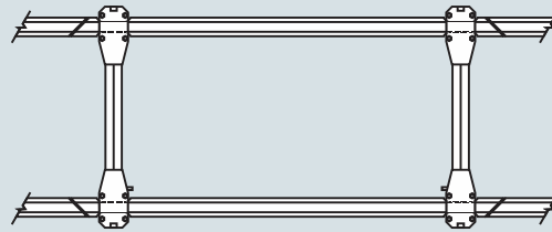
Top view of rails and cross ties to top of load cells (main scale assembly not shown)
