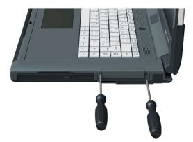
Open the cover and pull out the SSD unit.
