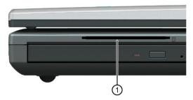
When inserting the card, pay attention to the correct positioning of the card. The chip must face upward.
