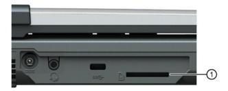
The contact areas of the card face downward. When inserting the card, pay attention to the correct positioning of the card.
