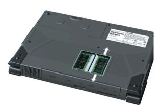
5. Pull the memory module out of the slot.
