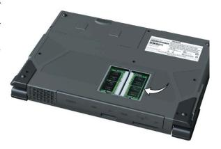
3. Put the cover back over the slot and fasten this with the screw.
