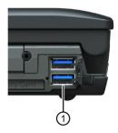
You can use the bottom USB socket under the cover on the side of the device ① to charge USB devices (e.g. smartphones) at a current of up to 1.5 A, even when the Field PG is switched off.
