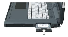
2. Close the cover, and secure it with the two screws.
