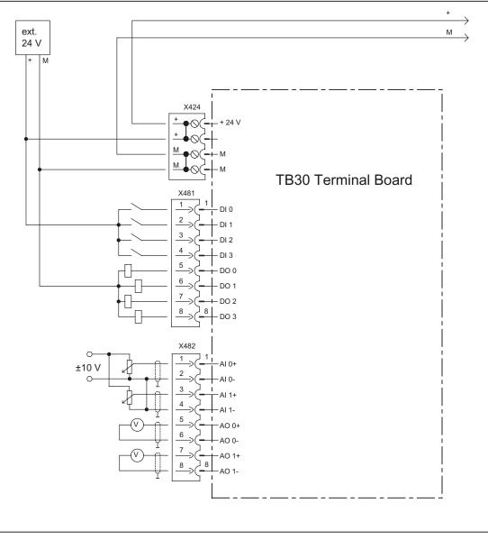
Figure 3-9 Example connection of TB30
