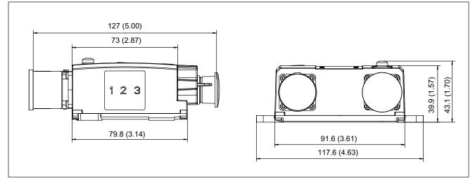
Figure 4-46 Dimension drawing SME125, Order number 6SL3055-0AA00-5KA3
