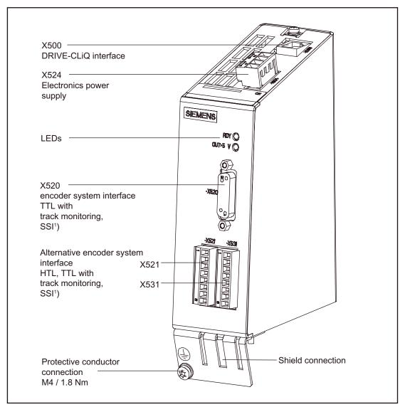
Figure 4-17 Interface description SMC30, 50 mm wide, order no. 6SL3055-0AA00-5CA0, 6SL3055-0AA00-5CA1
