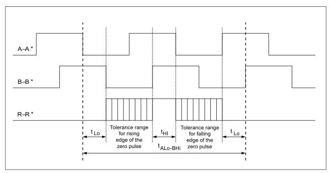
Figure 4-27 Position of the zero pulse to the track signals
