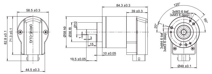
Figure 4-52 Dimension drawing: Clamping flange
