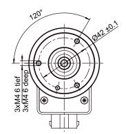
Figure 4-51 Dimension drawing: Synchronous flange
