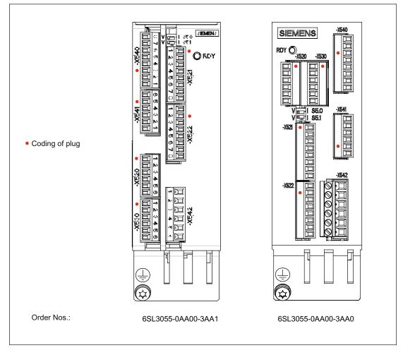
To ensure that identical connectors are assigned correctly on the TM31, the connecters are encoded as shown in the following diagram.
