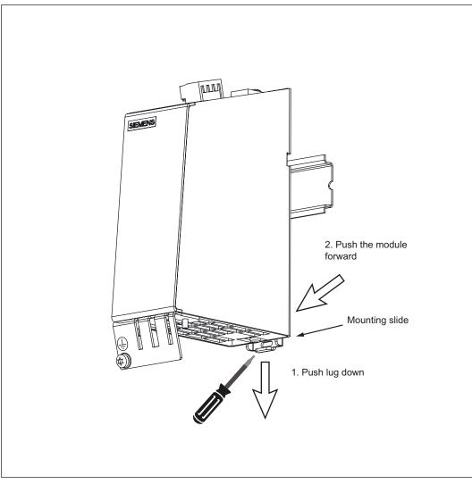
Figure 3-46 Releasing the component from a DIN rail
