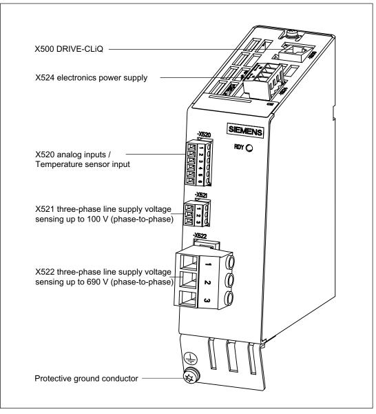
Figure 3-43 Voltage Sensing Module VSM10
