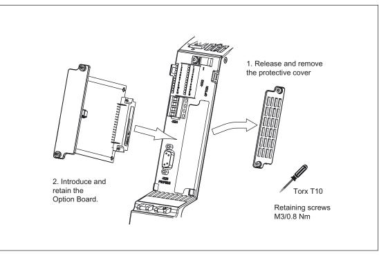
Figure 3-7 Installing the CBE20
