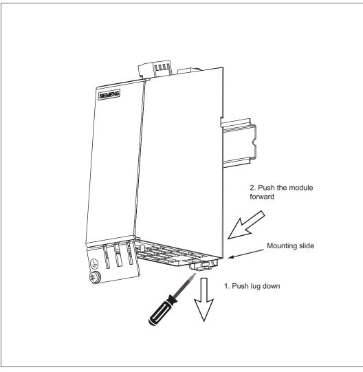
Figure 3-39 Releasing the component from a DIN rail
