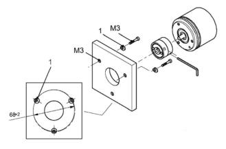
Figure 4-54 Installation: Synchronous flange, 1: Clamp straps
