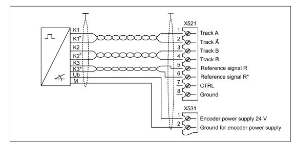
Connection example 1: HTL encoder, bipolar, with reference signal
