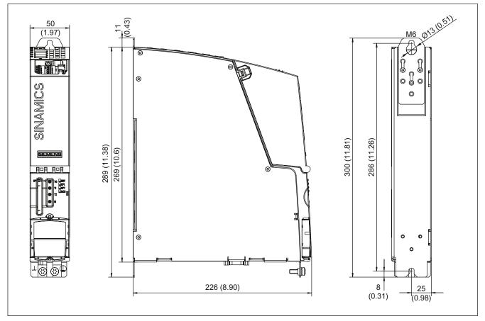
Figure 2-7 Dimension drawing: CU320
