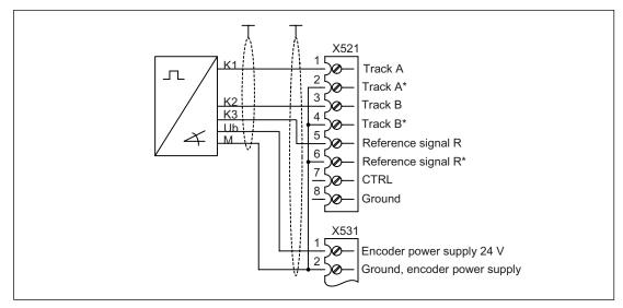
Figure 4-19 Connection example 2: HTL encoder, unipolar, with reference signal<sup>1)</sup>
