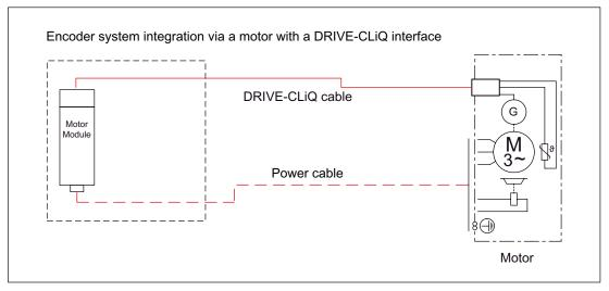
Figure 4-4 Encoder system integration via a motor with a DRIVE-CLiQ interface
