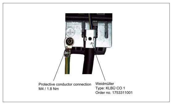
Figure 4-24 Shield contacts for the SMC30
