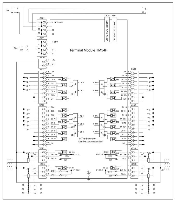
Figure 3-34 Connection example: TM54F
