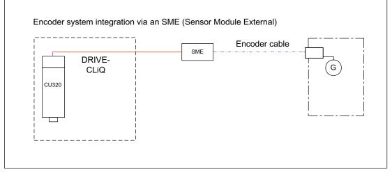
Figure 4-5 Encoder system integration via an SME (Sensor Module External)
