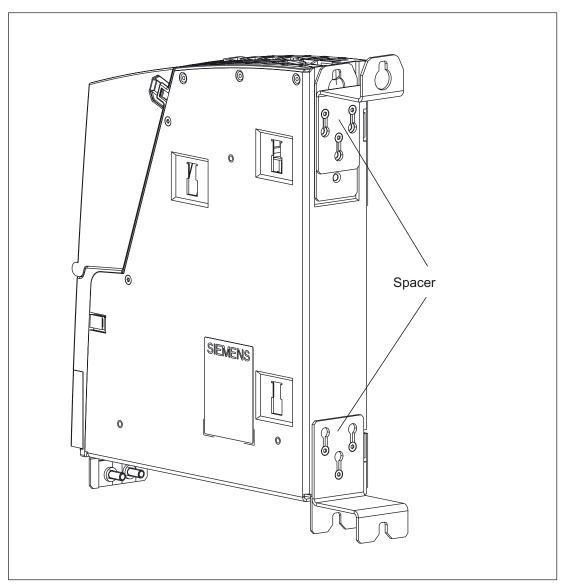
Figure 2-10 Installing the CU320 on a mounting surface using spacer elements
