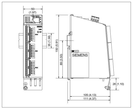
Figure 3-14 Dimension drawing of the TM15
