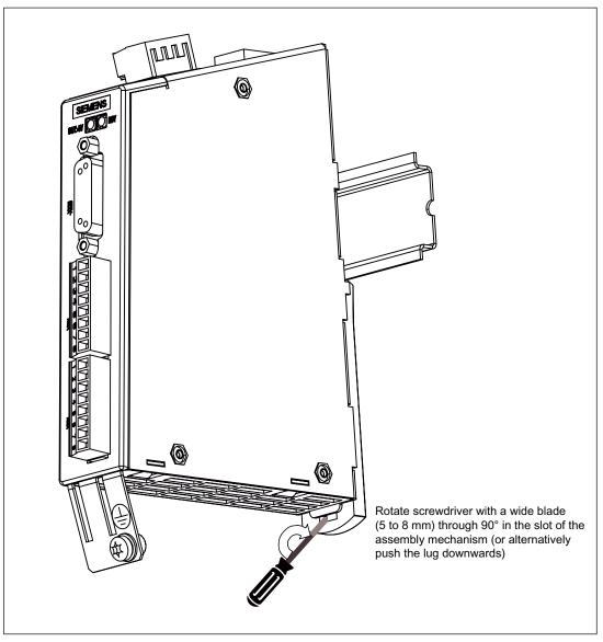
Figure 4-23 Removing: SMC30: 30 mm wide
