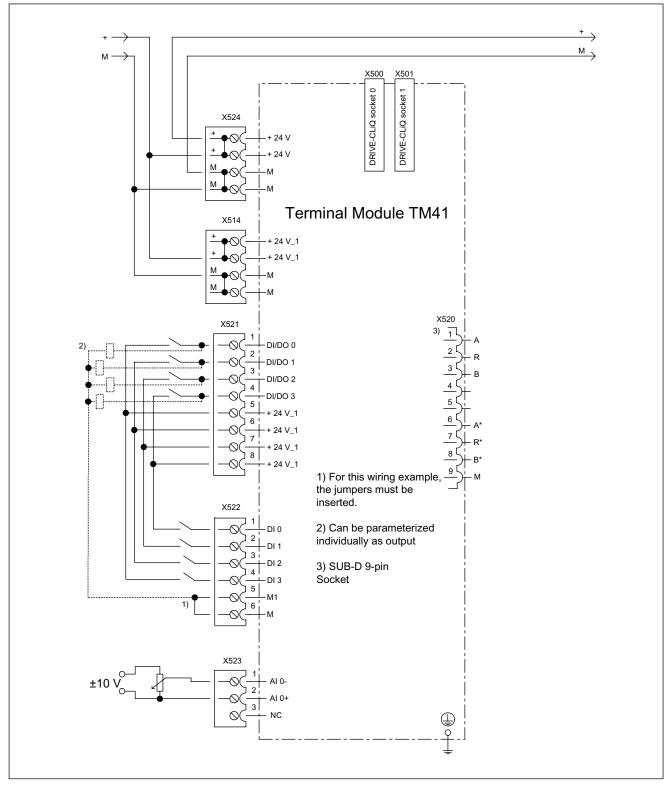
Figure 3-28 Sample connection of TM41
