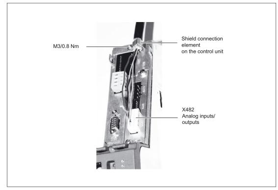
Shield connection of the TB30 on the Control Unit
