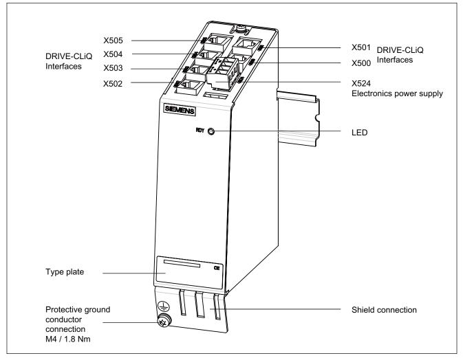
Figure 3-37 Interface description of the DMC20
