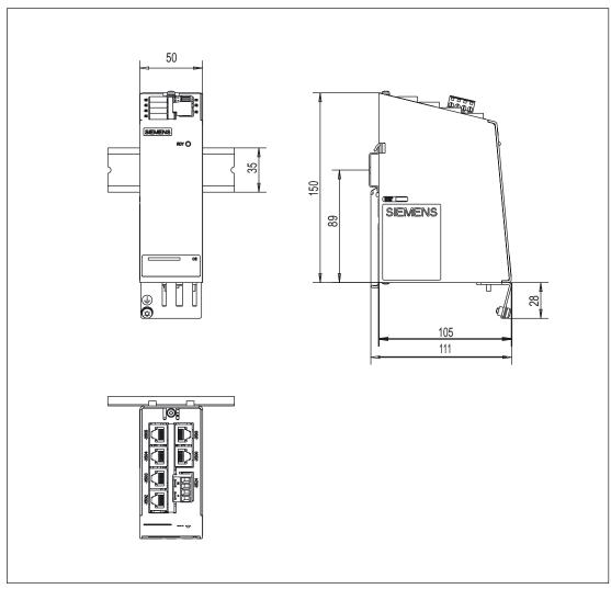
Figure 3-38 Dimension drawing of the DMC20
