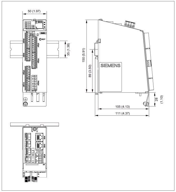
Figure 3-21 Dimension drawing TM31, order number: 6SL3055-0AA00-3AA1
