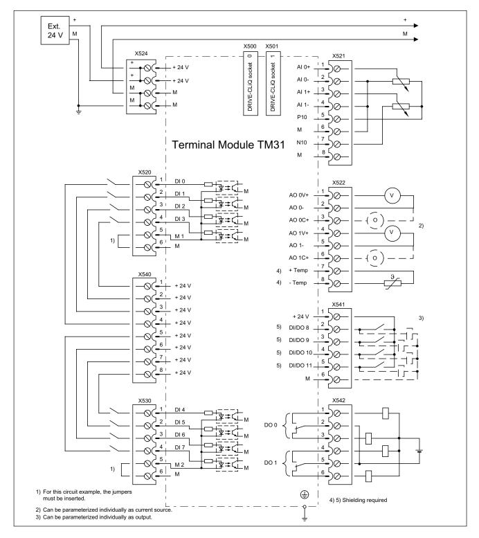
Figure 3-20 Example connection of TM31
