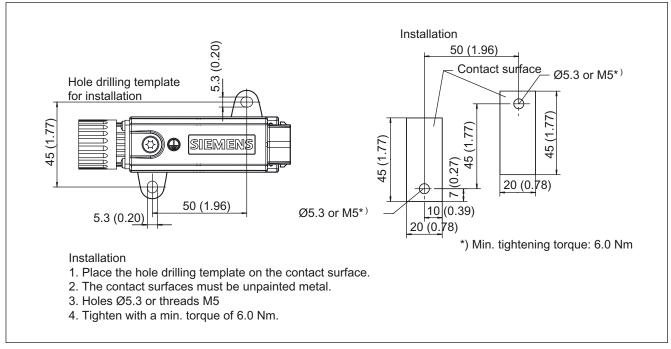
Figure 4-36 Installing the SME20/SME25
