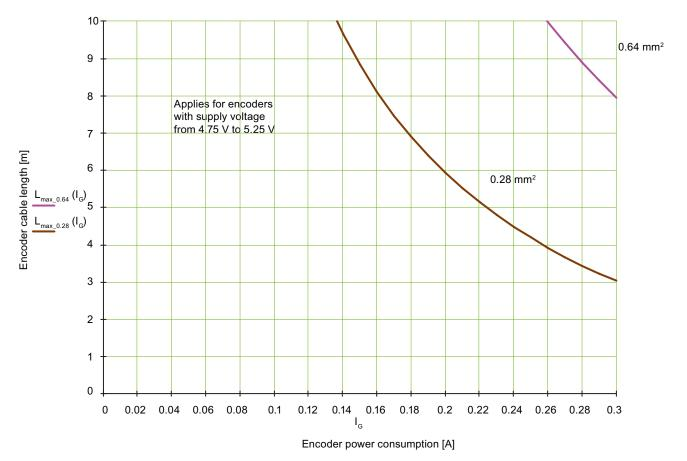
Figure 4-43 Max. cable length as a function of the current drawn by the encoder system
