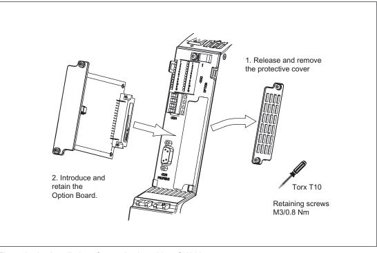
Figure 3-10 Installation of an option board in a CU320
