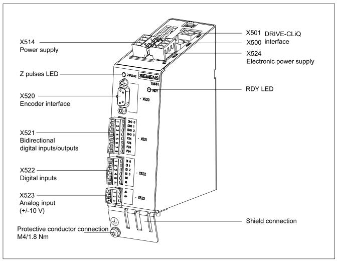
Figure 3-27 TM41 interface description, Order number 6SL3055-0AA00-3PA0
