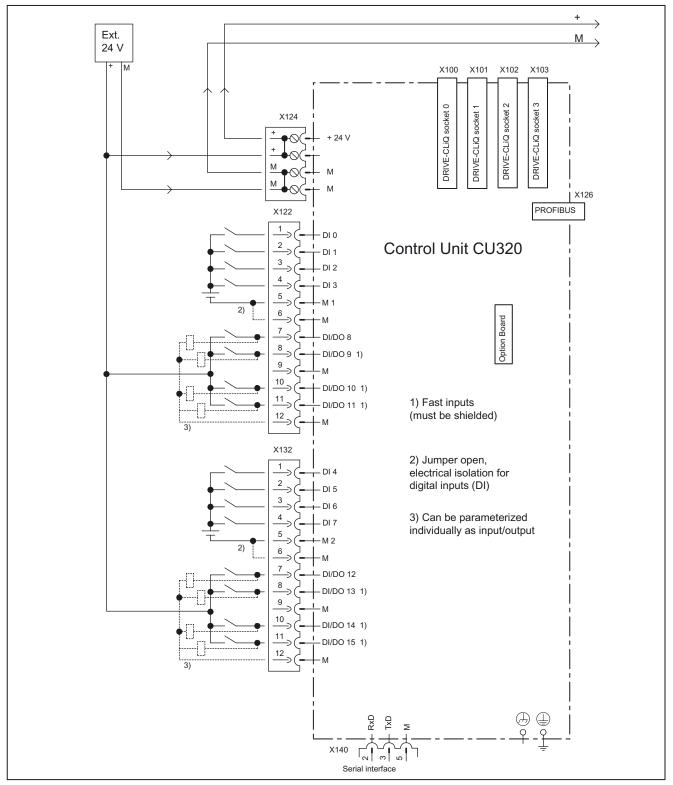
Figure 2-4 Example connection of CU320
