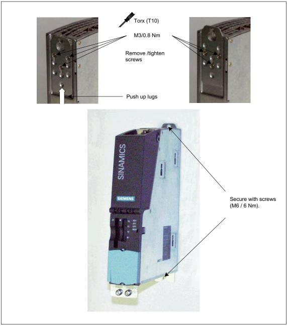
Figure 2-9 Installing the CU320 directly on a mounting surface
