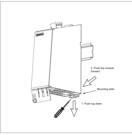
Figure 4-9 Releasing the component from a DIN rail
