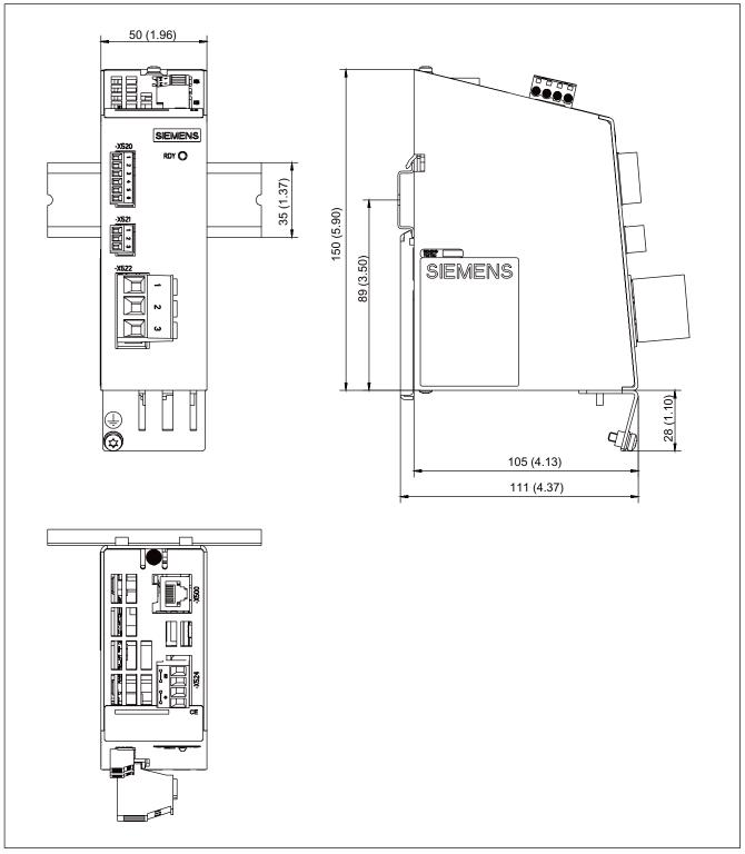
Figure 3-45 Dimension drawing: Voltage Sensing Module
