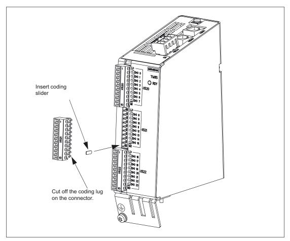
Figure 3-17 Procedure for encoding a connector
