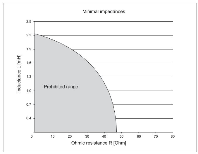
Figure 4-10 Connectable impedances with an excitation frequency f = 5000 Hz
