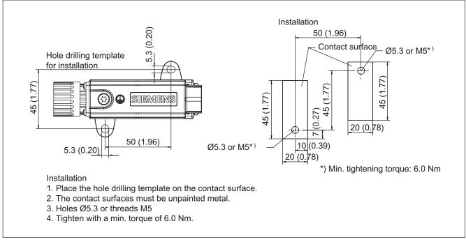
Figure 4-31 Installing the SME20/SME25
