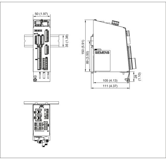
Figure 3-22 Dimension drawing TM31, order number: 6SL3055-0AA00-3AA0
