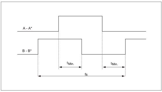
Figure 4-26 Signal characteristic of track A and track B between two edges: Time between two edges with pulse encoders
