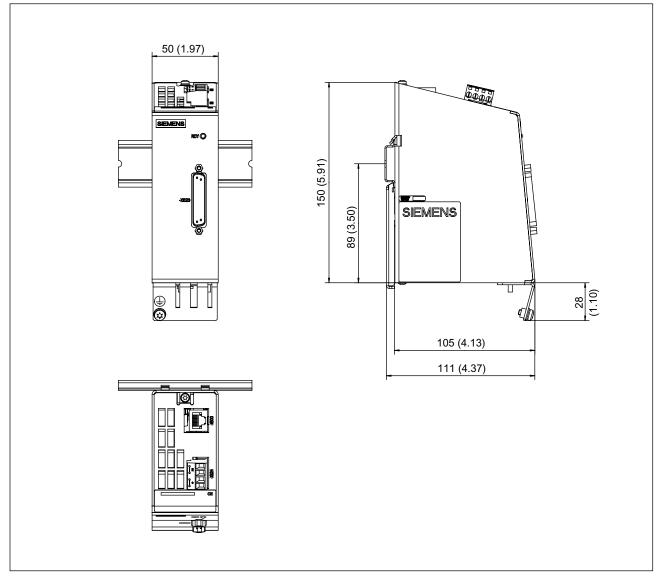
Figure 4-8 Dimension drawing of the SMC10
