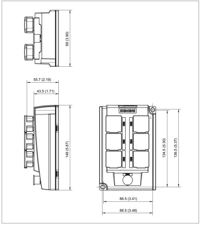
Figure 3-41 Dimension drawing: DME20
