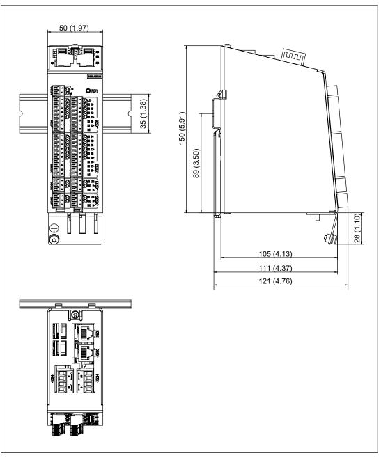
Figure 3-35 Dimension drawing of TM54F
