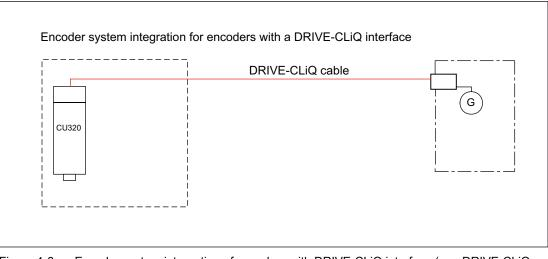
Figure 4-6 Encoder system integration of encoders with DRIVE-CLiQ interface (e.g. DRIVE-CLiQ encoder)
