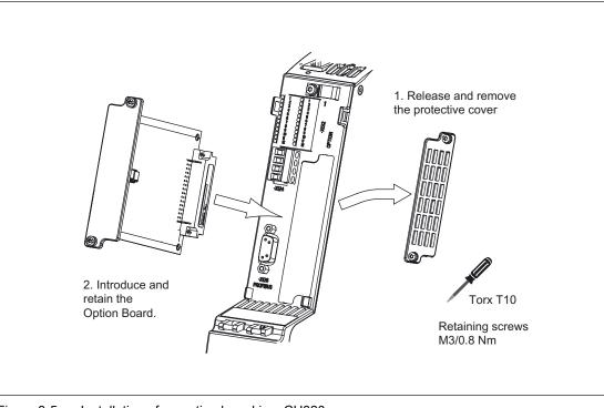
Figure 3-5 Installation of an option board in a CU320
