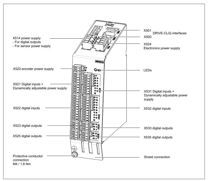
Figure 3-33 Interface description of the TM54F
