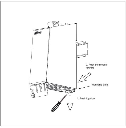
Figure 3-31 Releasing the component from a DIN rail
