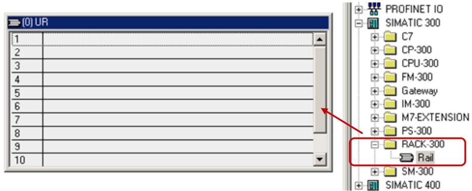
In the hardware catalog, select the CPU used and drag-and-drop this to slot 2 in the rack. A CPU 319-3PN/DP is used in this example.
