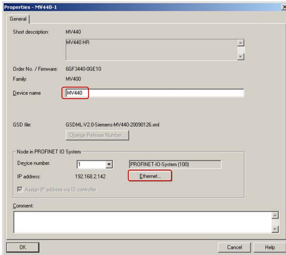
Enter the IP address of the SIMATIC MV440 code reading system.
