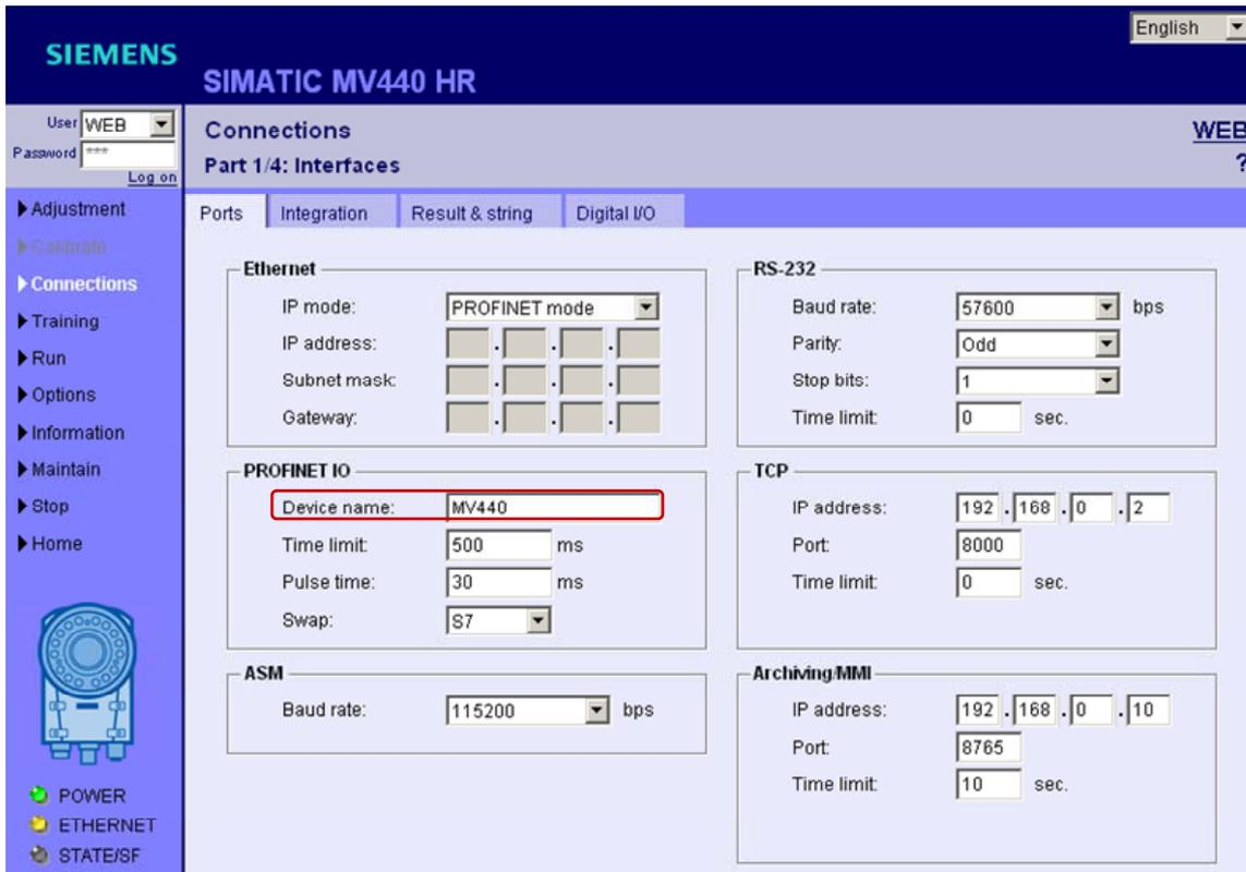
Select the "Integration" tab and then select "PROFINET IO" as source for the Trigger under Connection.
