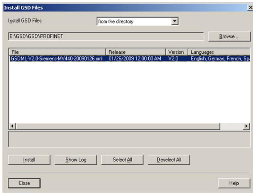
**Note** The GSD file is in the "VS130-2 Mode" directory on the CD included in the delivery package of the SIMATIC MV440 code reading system.
