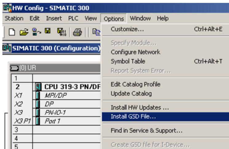
In the "Install GSD Files" dialog, click on the "Browse..." button. Select the directory in which the GSD file of the SIMATIC MV440 code reading system is stored.
