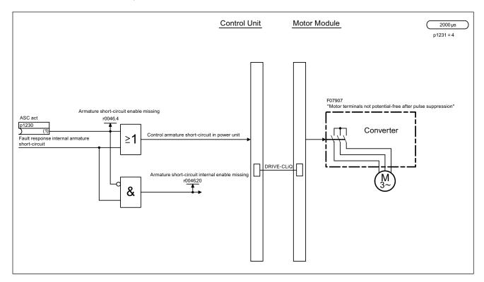
Figure 6-4 Internal armature short-circuit
