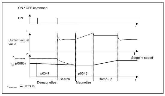
Figure 4-27 Flying restart, example of induction motor without encoder
