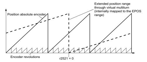
Figure 7-12 Position tracking (p2721 = 24), setting p2504 = p2505 =1 (gear factor = 1)
