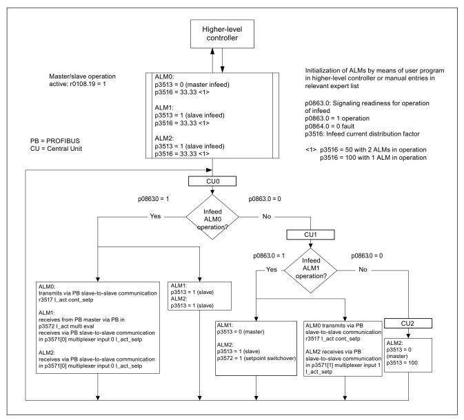
Figure 7-26 Structogram of master/slave operation, 3 identical Active Line Modules (ALMs) of identical output rating, PROFIBUS communication system
