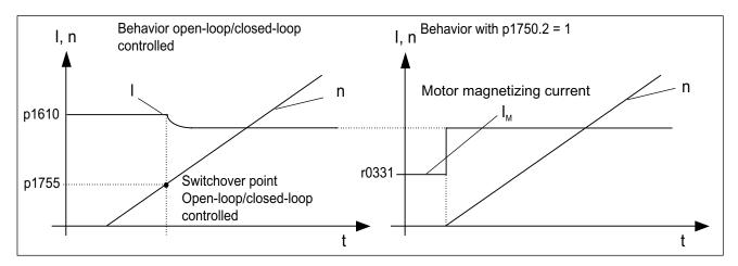
Figure 4-3 Vector control without an encoder
