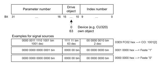
Figure 12-6 Internal encoding of the binector/connector output parameters
