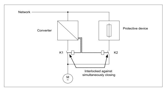
Figure 4-32 Circuit example, bypass without synchronization
