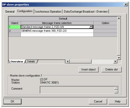
Figure 10-29 Telegram selection for drive object
