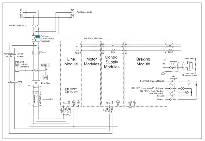
Figure 11-14 Example: interconnection of quick stop due to power failure or emergency off
