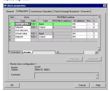
Figure 10-30 Detail view of slave configuration
