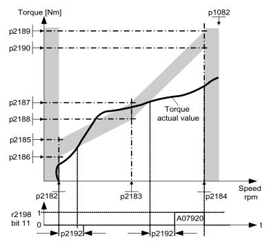
Figure 7-3 Load monitoring
