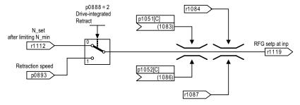
Figure 7-41 Connecting the setpoint channel to the ramp-function generator
