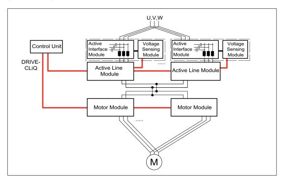
Figure 7-37 Example 2 parallel connection of Active Line Modules (chassis format) and Motor Modules
