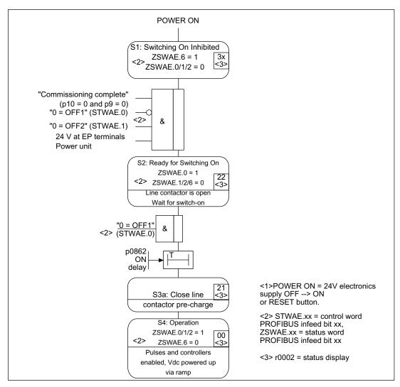
Figure 1-9 Basic Infeed power-up
