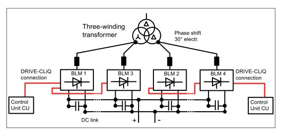
Figure 7-32 Parallel connection BLM 12-pulse redundant
