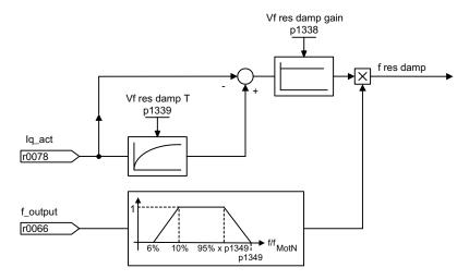
Figure 5-6 Resonance damping
