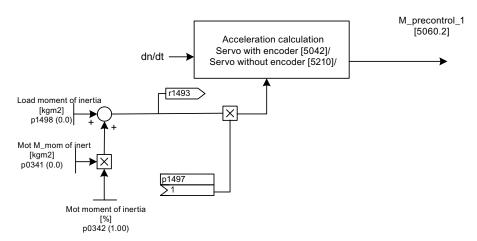
Figure 11-9 Torque pre-control for SERVO control
