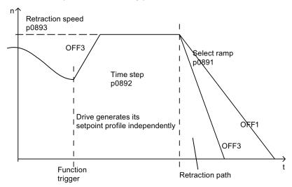
Figure 7-40 OFF ramp with "extended retract"
