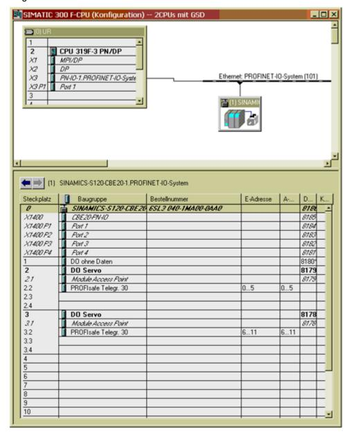
Figure 10-50 Two projects: Configuring the F-CPU
