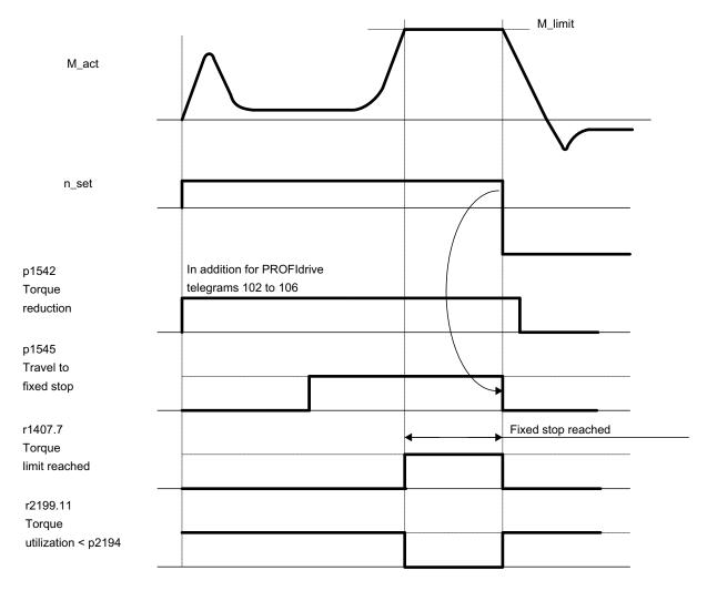
Figure 3-26 Signal chart for "Travel to fixed stop"
