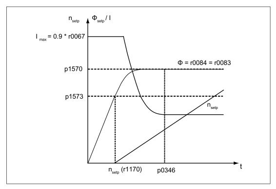
Figure 4-23 Quick magnetization characteristics
