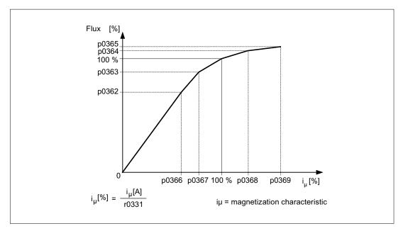
Figure 4-21 Magnetization characteristic
