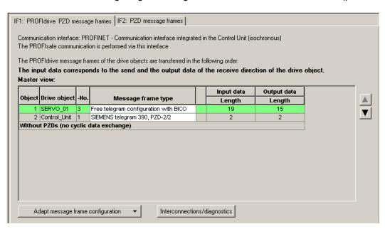
Figure 10-36 Configuring the slave-to-slave communication links in STARTER
