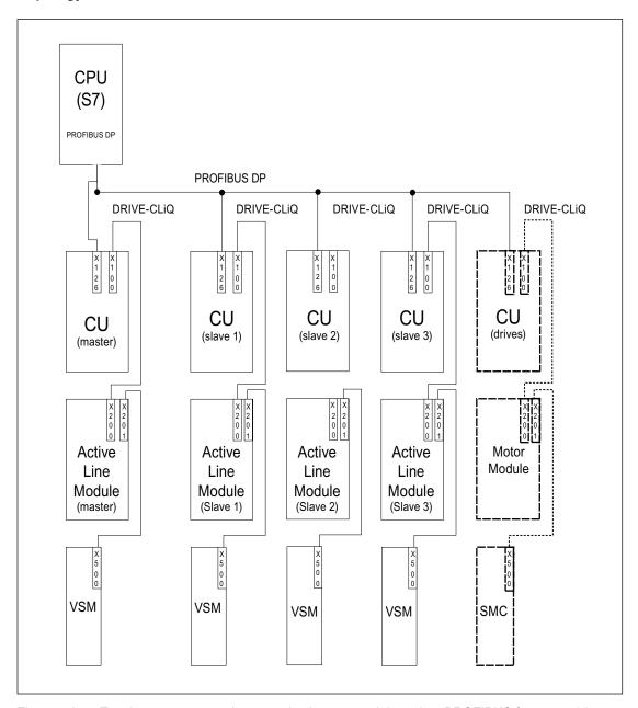
Figure 7-25 Topology structure and communications network based on PROFIBUS for master/slave operation with redundant infeeds (4 infeed trains)
