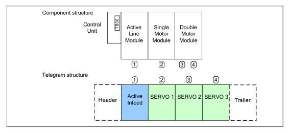
Figure 10-18 Component and telegram structure
