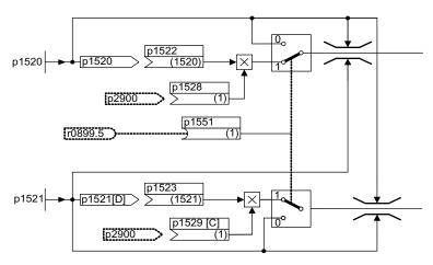
Figure 6-7 Torque limits OFF3
