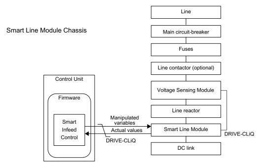
Figure 1-5 Schematic structure of Smart Infeed chassis
