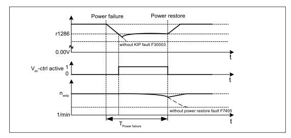
Figure 5-8 Switching Vdc\_min control on/off (kinetic buffering)
