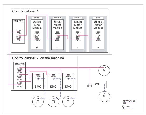
Figure 11-4 Example, distributed topology using DMC20
