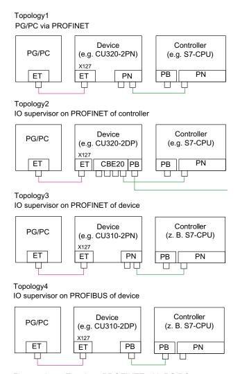
Figure 10-41 Topology PROFINET with PG/PC,
