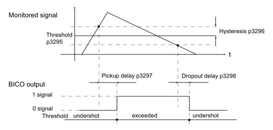
Figure 3-27 Variable signaling function
