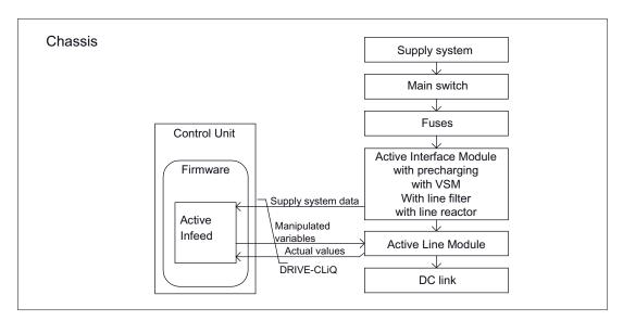
Figure 1-2 Schematic structure of Active Infeed chassis
