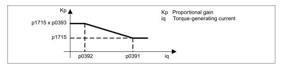
Figure 4-19 Current controller adaptation with swapped iq interpolation points for p0393 > 1, with p0392 < p0391
