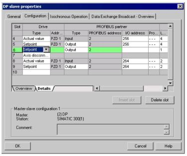
Figure 10-31 Insert new slot
