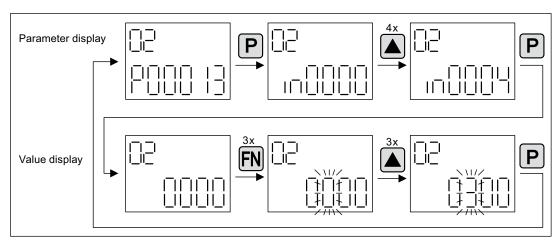
Figure 12-17 Example: Changing p0013[4] from 0 to 300
