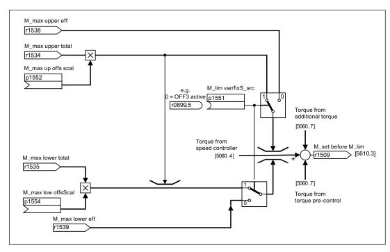
Figure 11-11 Limitation of the speed controller output with dynamic speed limits (example of SERVO) See 6060 for VECTOR application.
