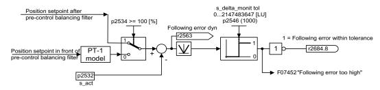
Figure 7-14 Following error monitoring
