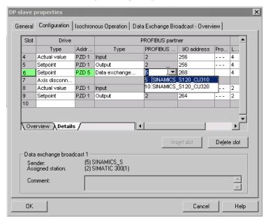
Figure 10-32 Configuring the slave-to-slave communication nodes
