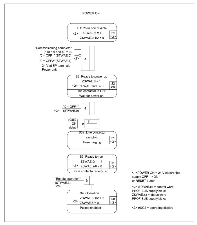
Figure 1-6 Smart Infeed power-up
