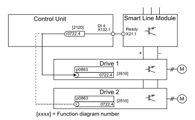
Figure 11-12 Example: interconnecting a Smart Line Module without DRIVE-CLiQ
