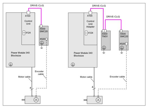
Figure 12-28 Wiring example for Power Modules Blocksize
