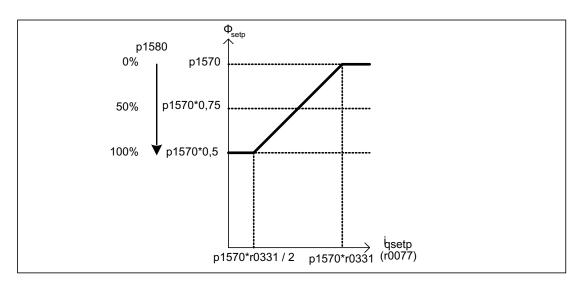
Figure 4-22 Efficiency optimization
