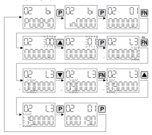
Figure 12-18 Example: Changing indexed binector parameters
