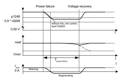
Figure 3-23 Switching Vdc\_min control on/off (kinetic buffering)
