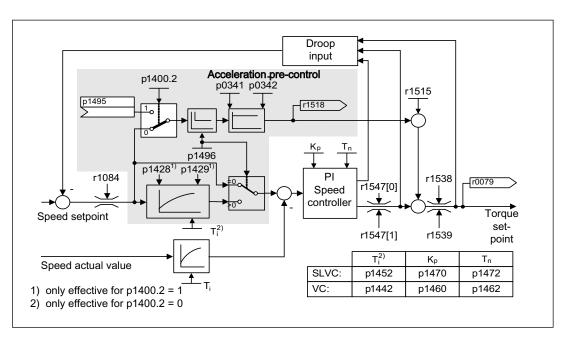
Figure 4-10 Speed controller with pre-control
