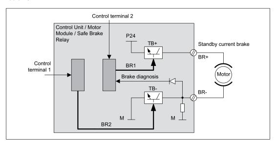
Figure 9-1 Two-channel brake control, blocksize (example)
