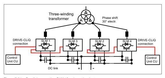
Figure 7-34 Parallel connection SLM 12-pulse redundant
