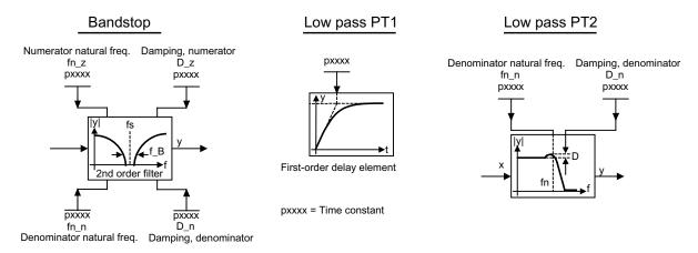
Figure 3-2 Filter overview for speed setpoint filters
