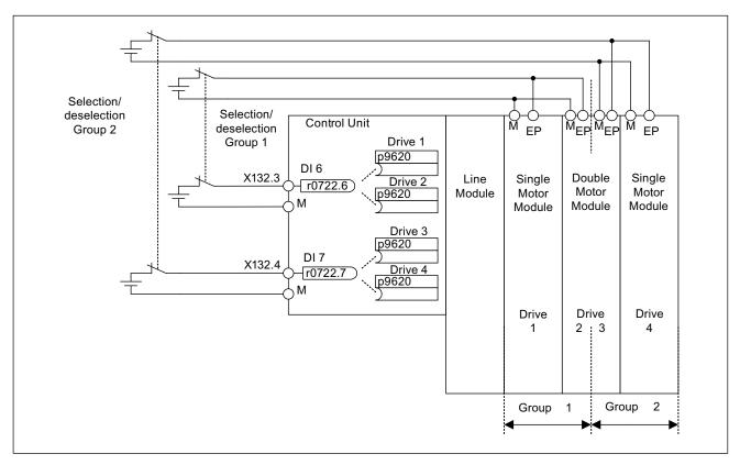
Figure 9-3 Example: Grouping terminals with Motor Modules Booksize and CU320-2
