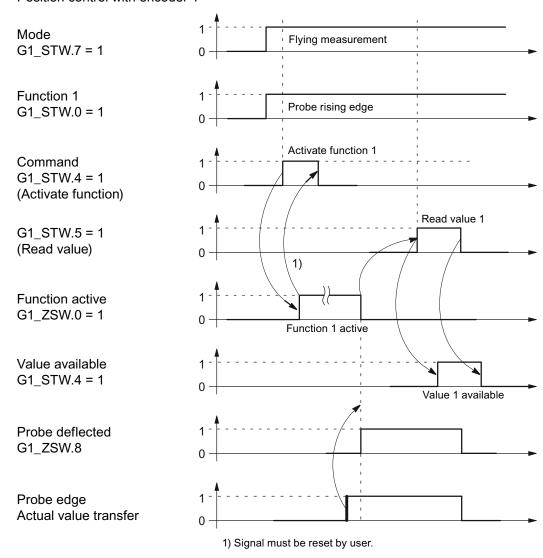
Figure 10-9 Sequence chart for "Flying measurement"
