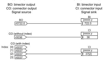
Figure 12-5 Interconnecting signals using BICO technology
