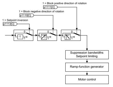
Figure 2-8 Direction of rotation limiting and direction reversal
