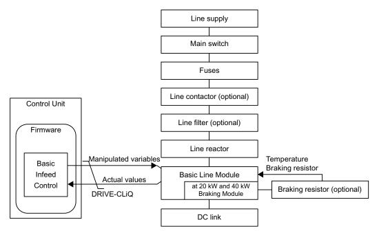
Figure 1-7 Schematic structure of Basic Infeed booksize
