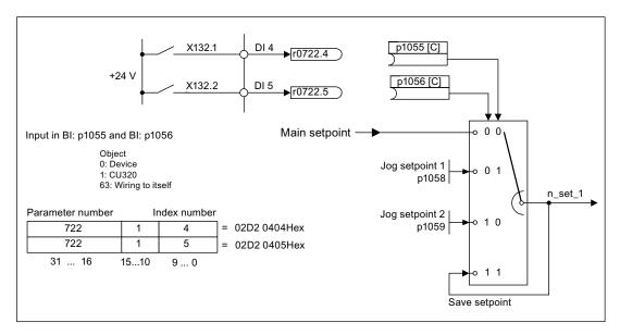
Figure 10-17 Task description for multi-parameter request (example)
