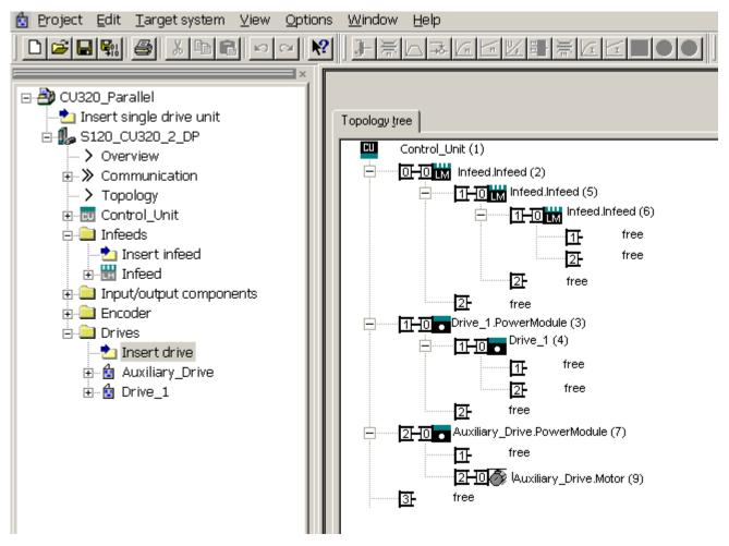
Figure 7-38 Topology with 3 Basic Line Modules, 2 Motor Modules and 1 auxiliary drive with SMI motor
