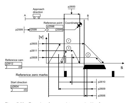
Figure 7-20 Example: reference point approach with reference cam
