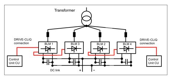
Figure 7-30 Parallel connection BLM 6-pulse redundant
