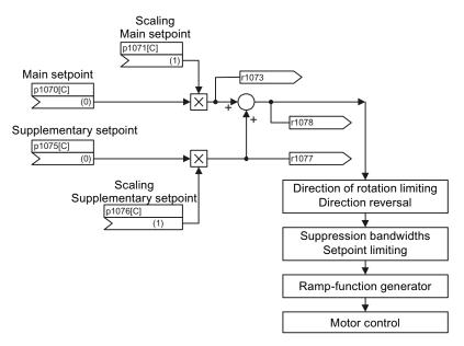
Figure 2-6 Setpoint addition, setpoint scaling
