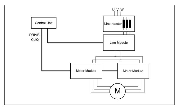
Figure 7-36 Example 1: parallel connection
