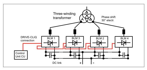
Figure 7-31 Parallel connection BLM 12-pulse single
