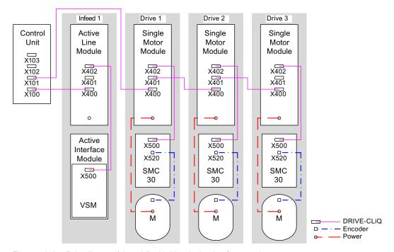
Figure 12-25 Drive line-up (chassis) with identical pulse frequencies
