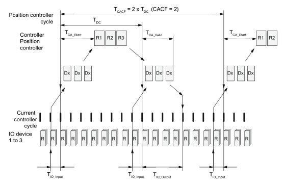
Figure 10-43 Motion Control/Isochronous drive link with PROFINET, optimized cycle with CACF = 2
