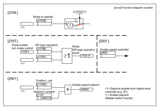
Figure 7-4 Example, operating brake for a crane drive
