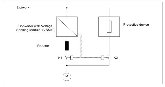
Figure 4-29 Circuit example: Bypass with synchronization with overlap
