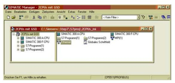
Figure 10-46 Both CPUs in one STEP7 project
