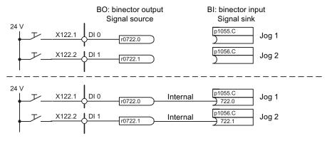
Figure 12-7 Interconnection of digital signals (example)
