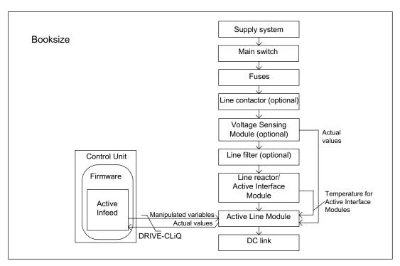
Figure 1-1 Schematic structure of Active Infeed booksize
