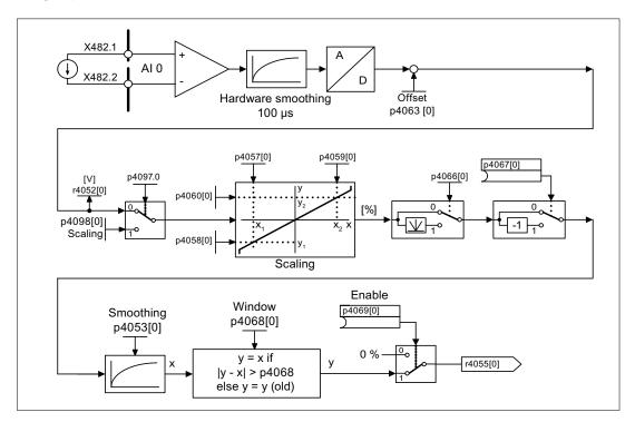
Figure 12-12 Analog inputs: Signal processing using Al0 of the TB30
