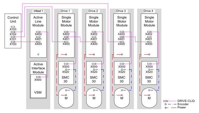
Figure 12-26 Drive line-up in chassis format with different pulse frequencies
