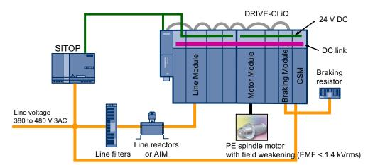
Figure 6-6 Example of a configuration recommended for application of internal voltage protection
