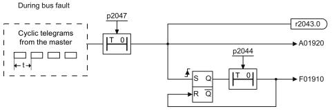
Figure 10-23 Monitoring telegram failure with a bus fault
