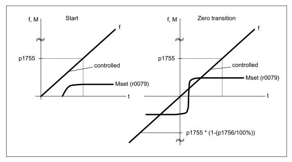
Figure 4-4 Zero point and starting in open-loop operation at low speeds
