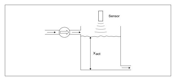
Figure 7-1 Fill level control: Application
