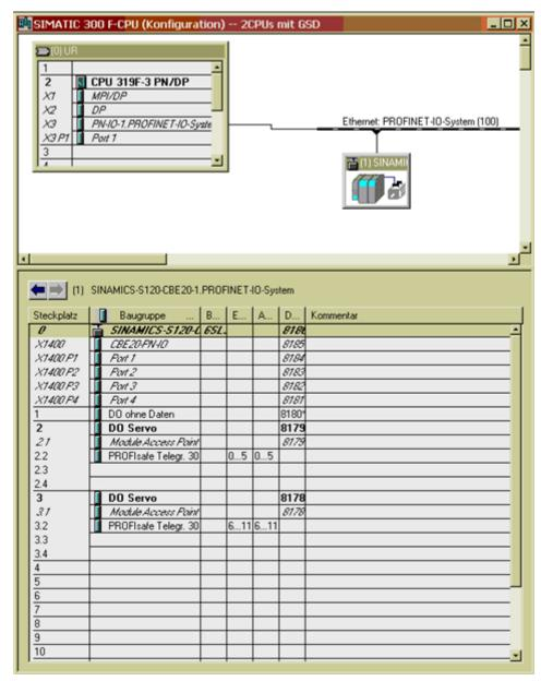
Figure 10-48 One project: Configuring the F-CPU
