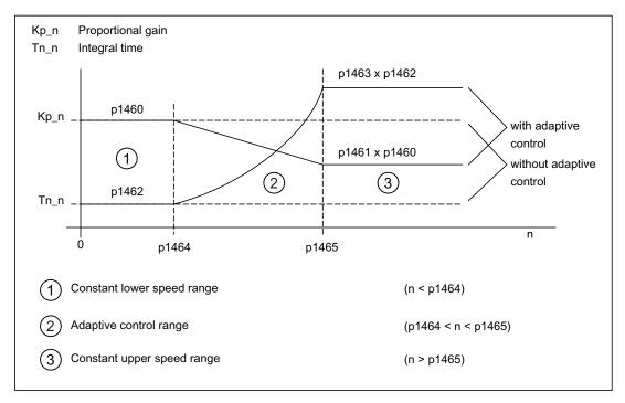
Figure 4-8 Speed controller Kp\_n/Tn\_n adaptation
