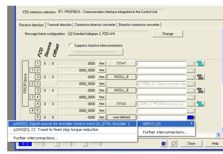
Figure 10-39 Combinding the PZDs for slave-to-slave communication with external signals
