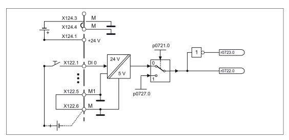
Figure 12-9 Digital inputs: Signal processing using DI 0 as an example
