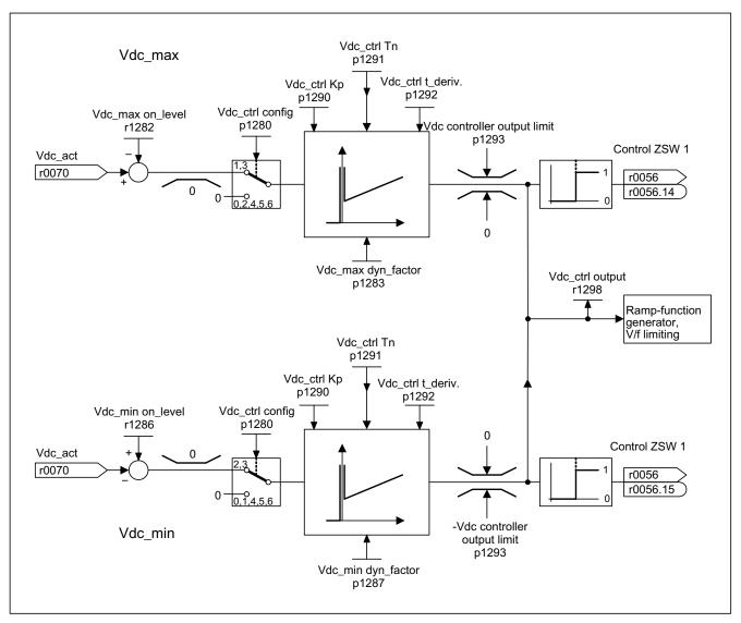
Figure 5-7 Vdc control V/f
