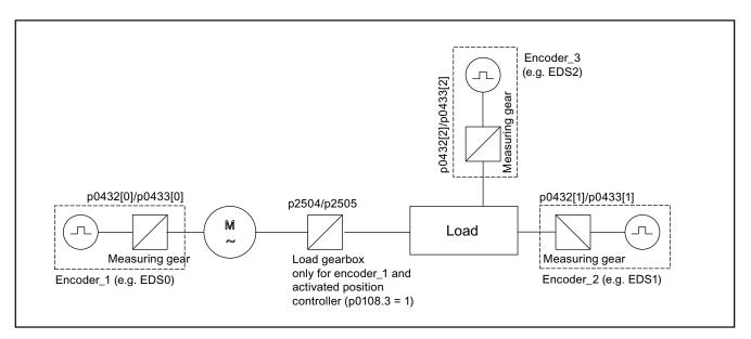
Figure 6-12 Overview of gears and encoders
