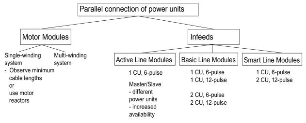
Figure 7-28 Parallel connection of power units - overview
