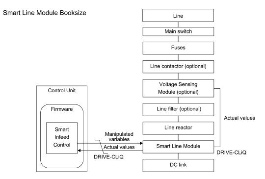
Figure 1-4 Schematic structure of Smart Infeed booksize
