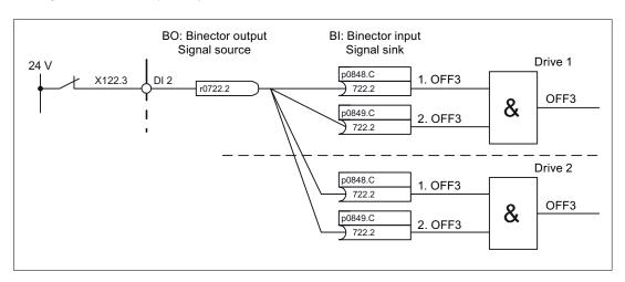
Figure 12-8 Connection of OFF3 to several drives (example)
