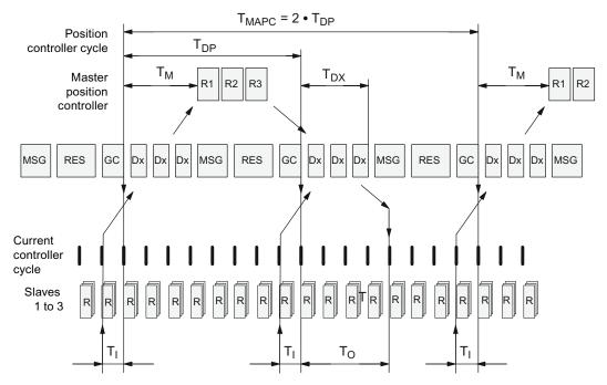
Figure 10-25 Motion Control/Isochronous drive link with PROFIBUS, optimized cycle with  $T_{MAPC}$  = 2 •  $T_{DP}$
