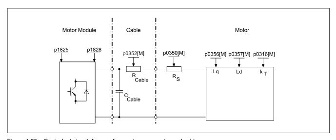
Figure 4-25 Equivalent circuit diagram for synchronous motor and cable
