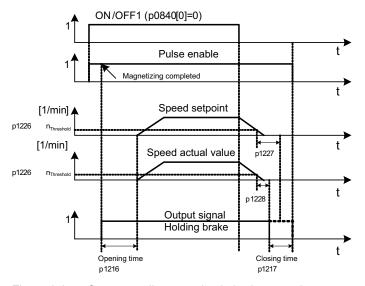
Figure 6-8 Sequence diagram, simple brake control
