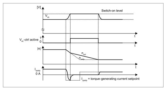
Figure 4-17 Switching Vdc\_max control on/off
