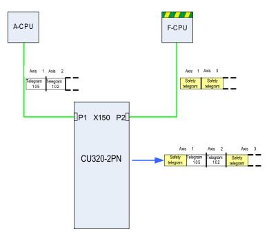
Figure 10-45 Example, communication sequence
