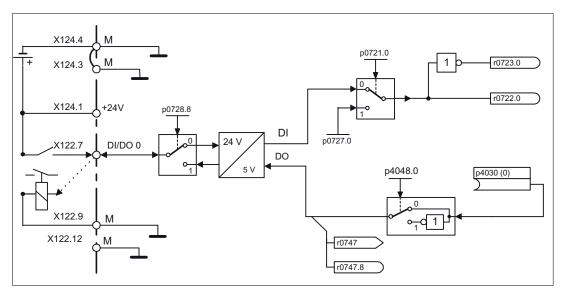
Figure 12-11 Bidirectional inputs/outputs: Signal processing using DI/DO 0 as an example
