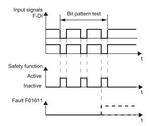
Figure 9-4 Inverter response to a bit pattern test
