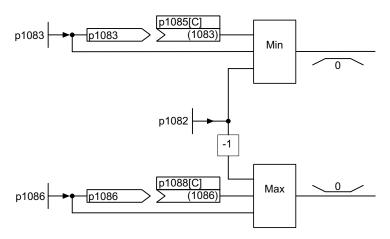
Figure 3-1 Speed controller limitations
