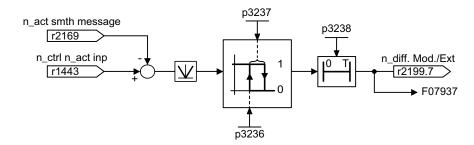
Figure 4-13 Monitoring "Speed deviation model / external in tolerance"
