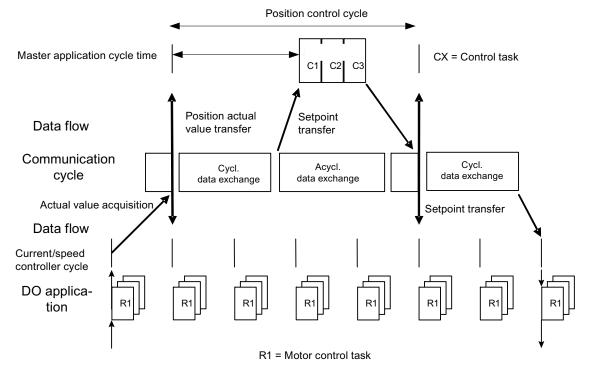
Figure 10-15 Isochronous drive link/Motion Control with PROFIdrive
