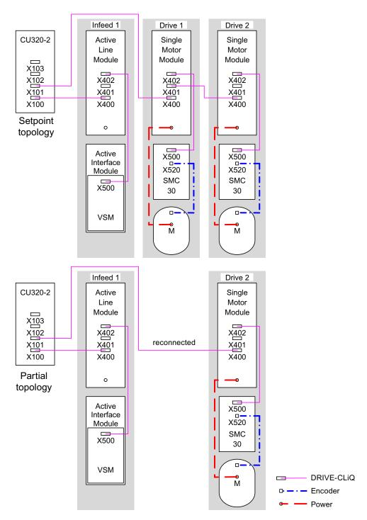
Figure 6-2 Example of a sub-topology
