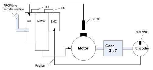
Figure 7-22 Measuring gear between the motor and encoder
