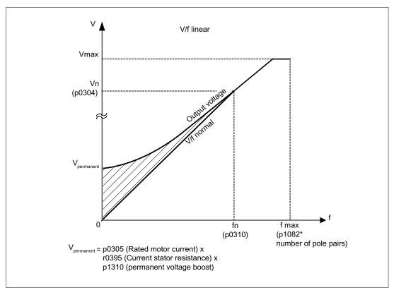
Figure 5-3 Permanent voltage boost (example: p1300 = 0 and p1310 > 0)
