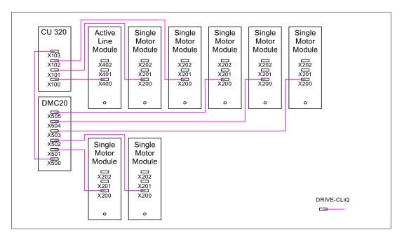
Figure 11-5 Example topology for hot plugging in vector V/f\_control mode
