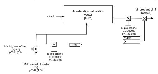
Figure 11-10 Torque pre-control for VECTOR control
