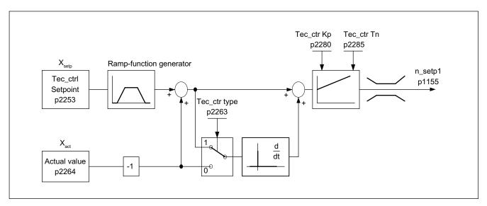
Figure 7-2 Fill level control: Controller structure
