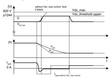
Figure 3-24 Switching-in/switching-out the Vdc\_max control
