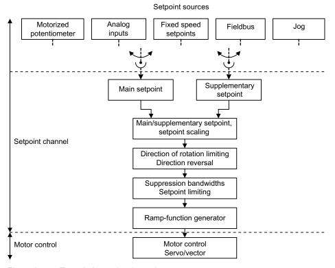
Figure 2-1 Extended setpoint channel
