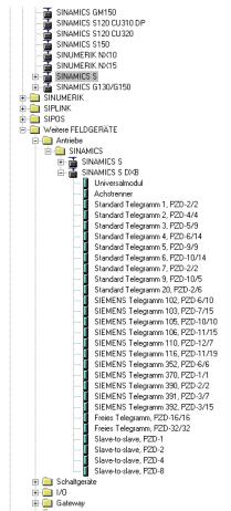
Figure 10-22 Hardware catalog of the generic station description file with slave-to-slave communication functionality
