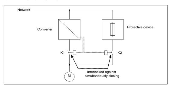
Figure 4-31 Circuit example, bypass with synchronization without overlap
