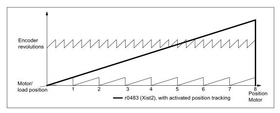
Figure 6-15 Odd-numbered gears with position tracking (p0412 = 8)
