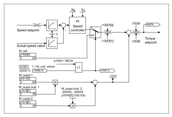
Figure 4-14 Closed-loop speed/torque control
