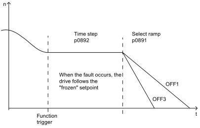
Figure 7-39 OFF ramp with timer
