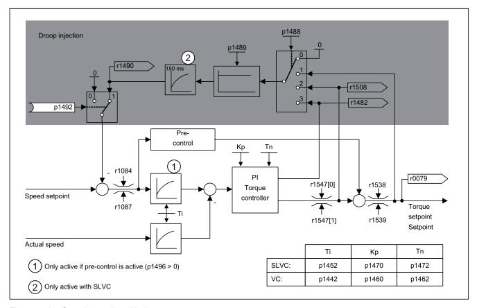
Figure 4-12 Speed controller with droop
