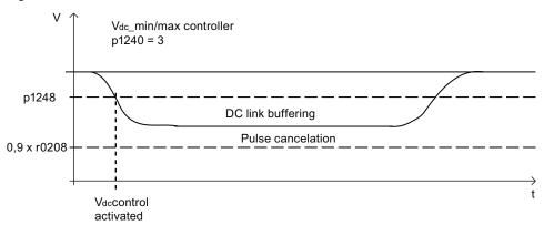
Figure 7-42 DC link voltage setpoint
