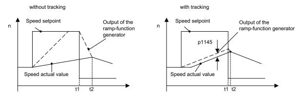
Figure 2-14 Ramp-function generator tracking
