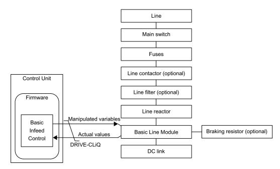
Figure 1-8 Schematic structure of Basic Infeed chassis
