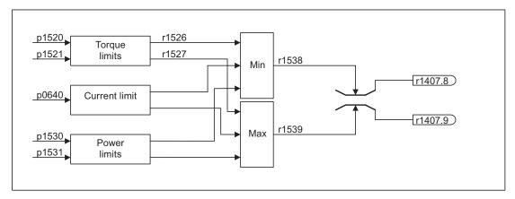
Figure 4-15 Torque limiting
