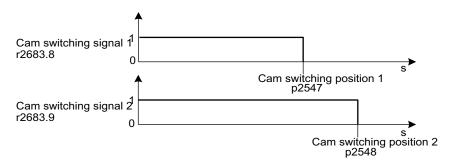
Figure 7-15 Cam controllers
