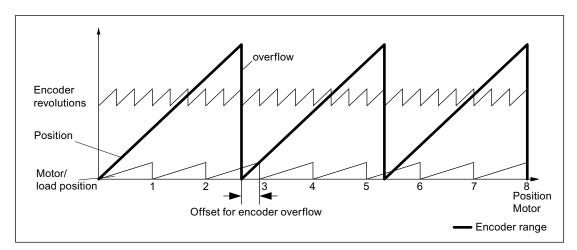
Figure 6-14 Drive with odd-numbered gears without position tracking
