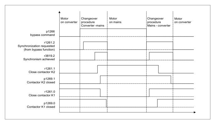
Figure 4-30 Signal diagram, bypass with synchronization with overlap
