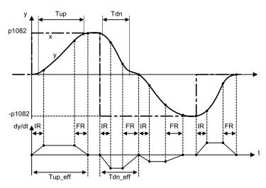
Figure 2-13 Extended ramp-function generator
