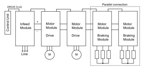
Figure 7-7 Parallel connection of Motor Modules as Braking Modules
