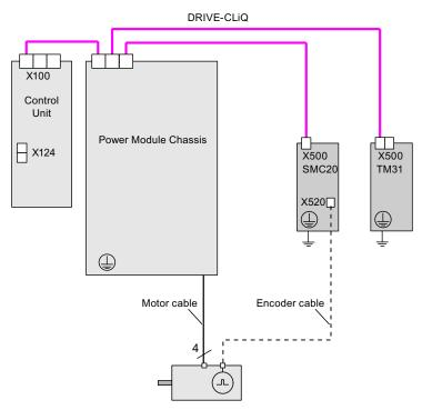
Figure 12-29 Wiring example for Power Modules Chassis
