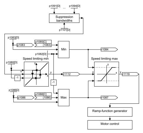
Figure 2-10 Suppression bandwidths, setpoint limitation
