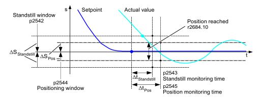
Figure 7-13 Zero-speed monitoring, positioning window
