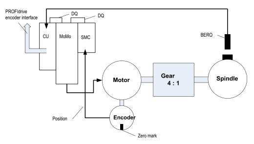
Figure 7-21 Design with a gear between the motor and spindle
