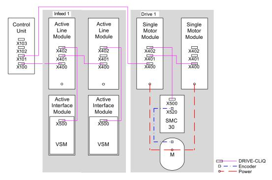
Figure 12-27 Drive line-up with parallel-connected power units in chassis format
