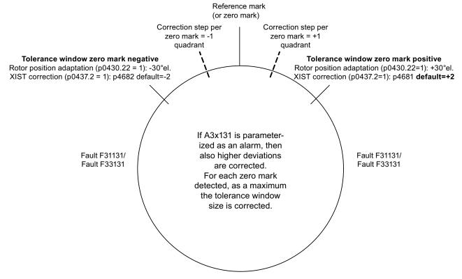
Figure 11-7 Tolerance window and correction
