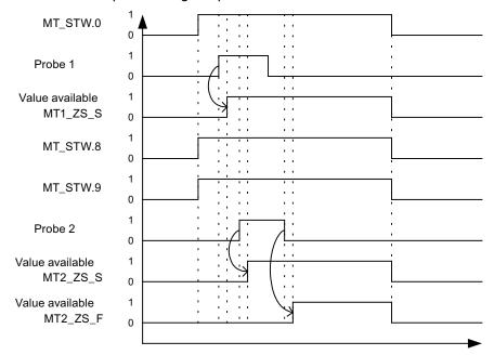
Figure 10-13 Sequence chart for central probe example
