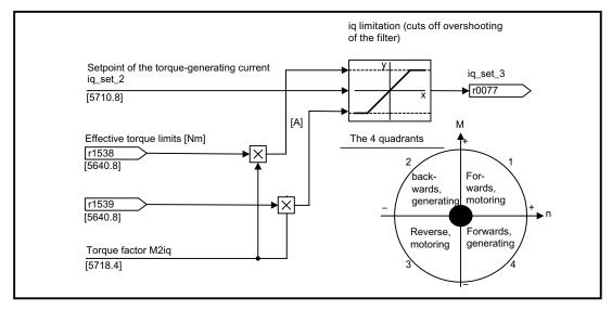
Figure 3-9 Current/torque setpoint limiting
