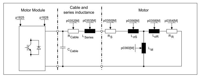
Figure 4-20 Equivalent circuit diagram for induction motor and cable
