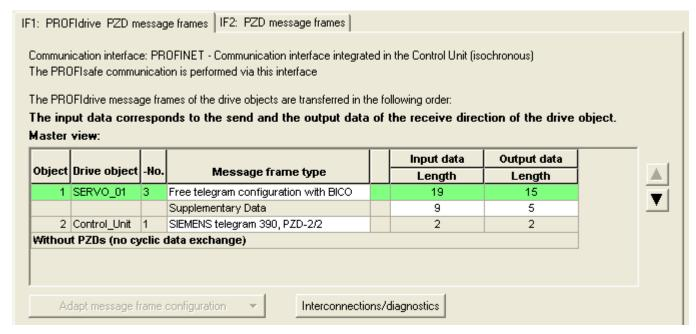
Figure 10-37 Display of the telegram extension
