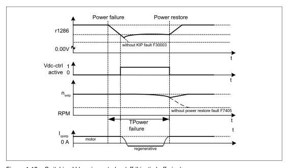
Figure 4-16 Switching Vdc\_min control on/off (kinetic buffering)
