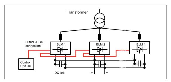
Figure 7-29 Parallel connection BLM 6-pulse single
