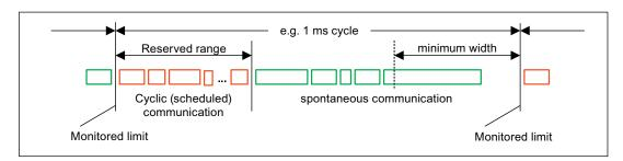
Figure 10-40 Bandwidth distribution/reservation, PROFINET IO
