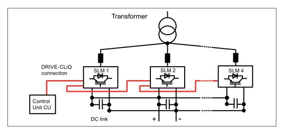
Figure 7-33 Parallel connection SLM 6-pulse single
