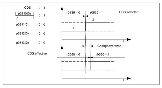
Figure 12-3 Switching the command data set (example)
