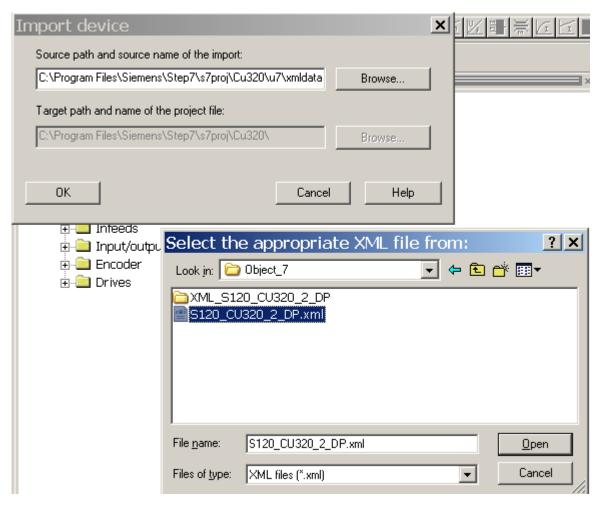
Figure 6-23 Select the xml file of the drive object
