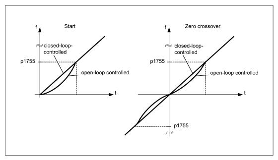
Figure 4-2 Zero crossover and when induction motors start in closed-loop or open-loop controlled operation
