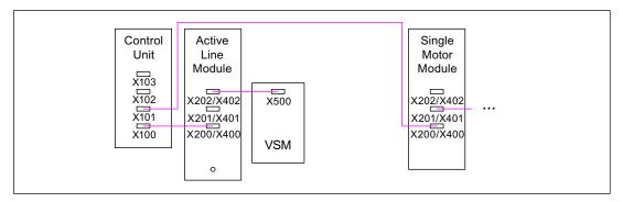
Figure 12-24 Example of a topology with VSM for booksize and chassis components
