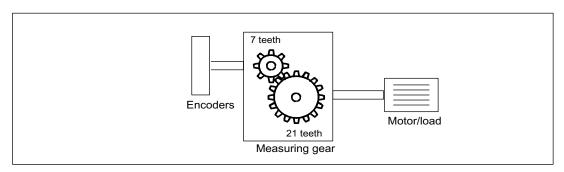
Figure 6-13 Measuring gear
