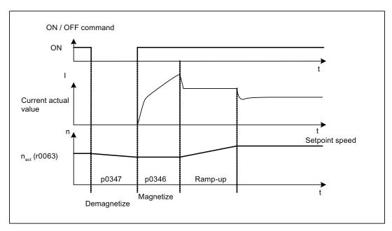
Figure 4-28 Flying restart, example of induction motor with encoder
