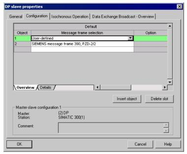
Figure 10-34 Telegram assignment for slave-to-slave communication
