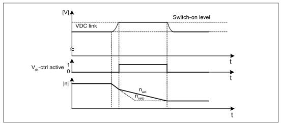
Figure 5-9 Switching Vdc\_max control on/off
