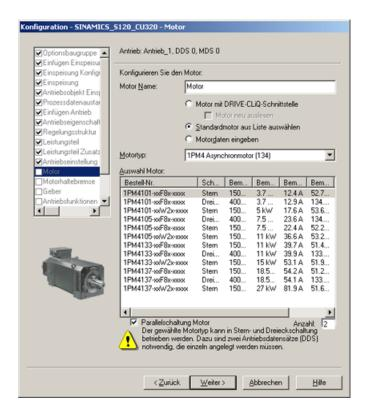
Figure 7-27 Selection of motors for parallel connection
