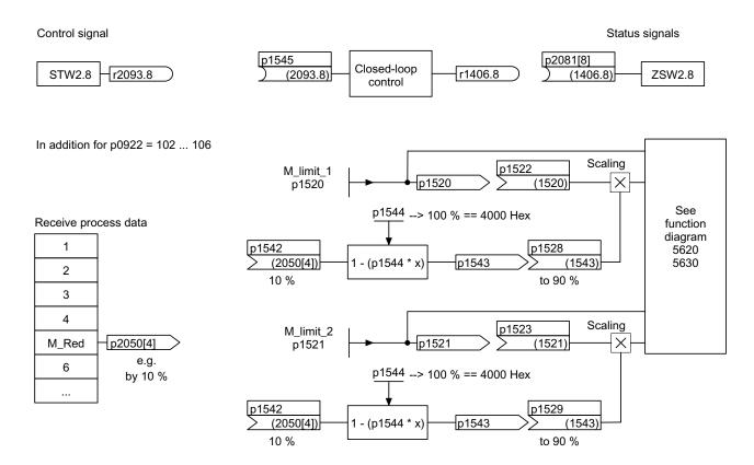
Figure 3-25 Signals for "Travel to fixed stop"
