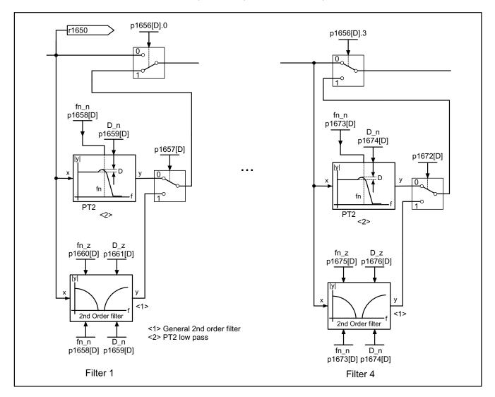
Figure 3-14 Current setpoint filter
