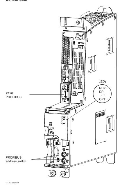
Figure 10-21 Interfaces and diagnostic LED
