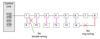
Figure 12-22 Example: DRIVE-CLiQ line connected to the X103 DRIVE-CLiQ connection of a Control Unit
