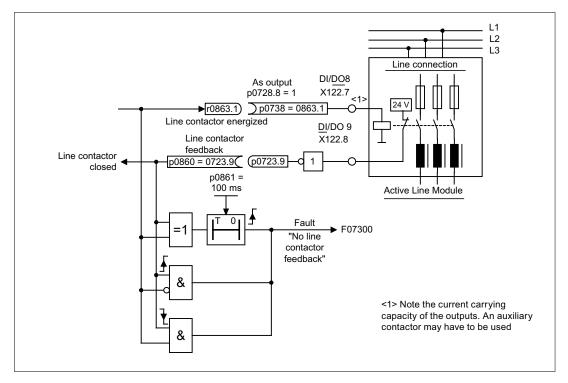
Figure 1-10 Line contactor control
