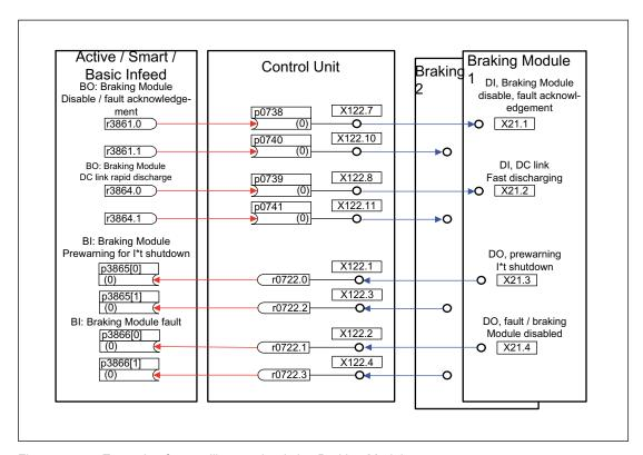
Figure 7-5 Example of controlling two booksize Braking Modules
