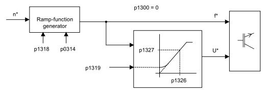
Figure 3-16 Structure of V/f control
