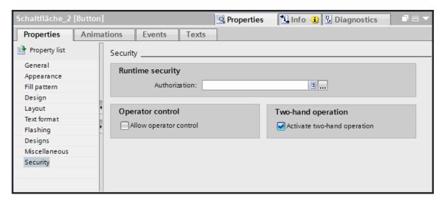
4. To unlock the operator controls, disable the option "Activate two-hand operation" under "Properties > Properties > Security".
