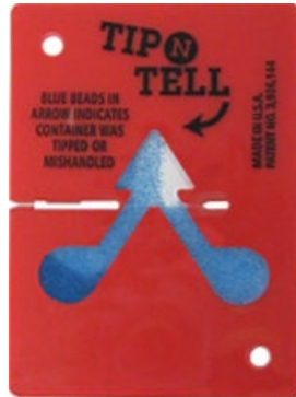
Figure 3-5 Tilt indicator tripped
