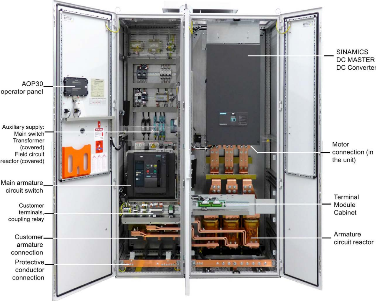
Figure 2-8 Main components - overview, frame size EC
