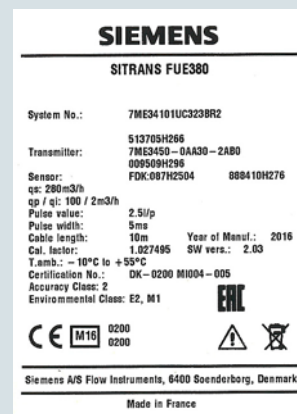
FUE380 transmitter label (with MID first verification)
