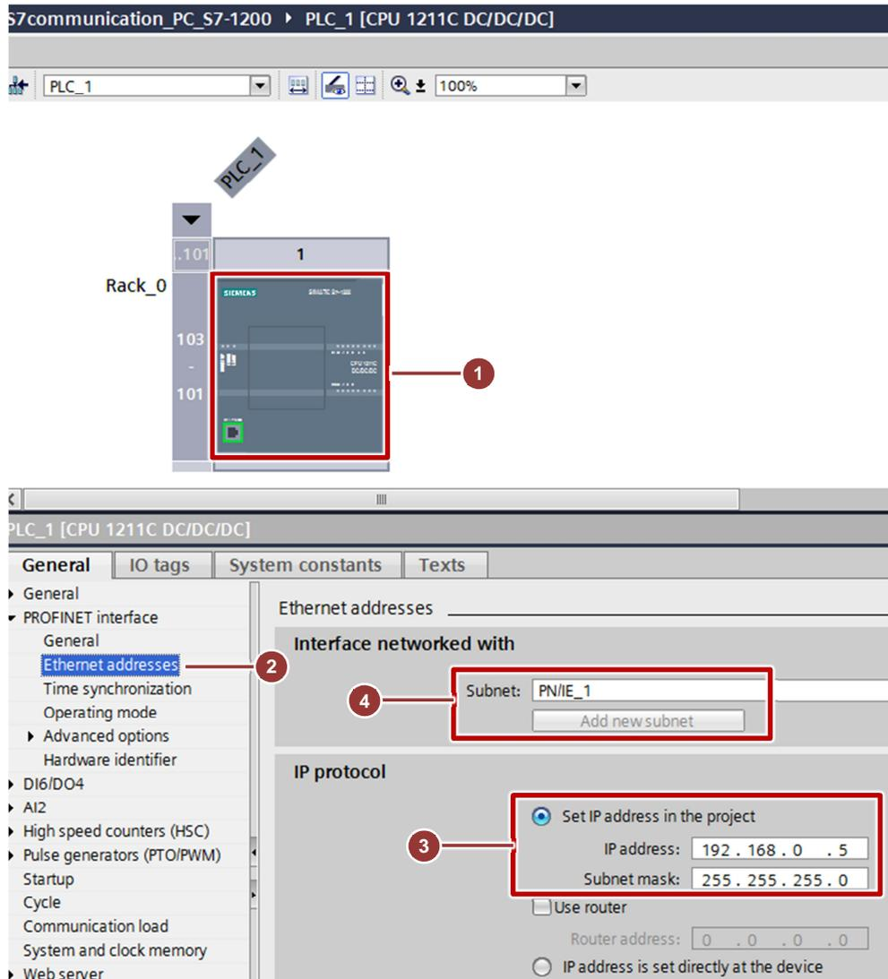
The connection between the subnet, PN/IE\_1, for example, and the S7-1200 is now displayed in the "Network View" of the Devices and Networks editor.
