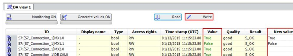
Enter the values below in the "New value" column (see [Table 2-4](#)). Click the "Write" button. The marker bit M2.0 and Bit 0 in DB1 are reset to the value "False".
