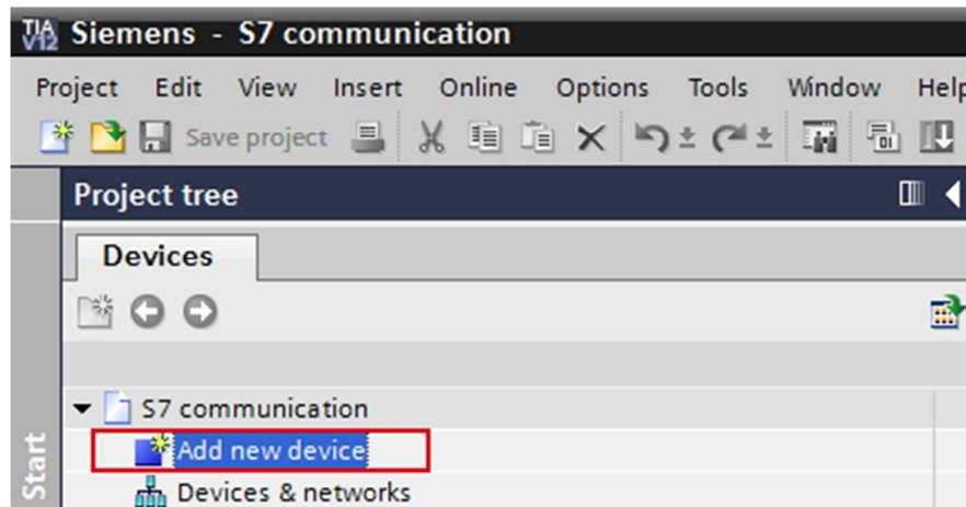
Click the "Controllers" button in the working area. Go to "Controllers > SIMATIC S7-1200 > CPU" and select the required controller. Click the "OK" button to add the selected S7-1200 CPU to your project.
