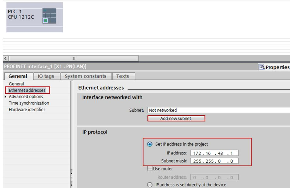
The connection between the subnet, PN/IE\_1, for example, and the S7-1200 is now displayed in the "Network View" of the devices and networks editor.
