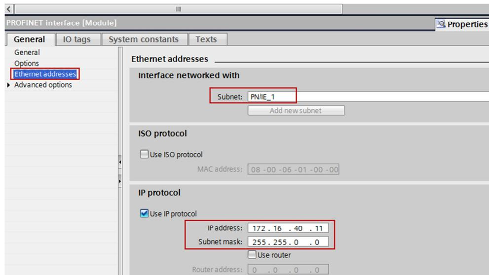
**Note** The IP address configured for the PC station in the TIA Portal must match the IP address set in Windows. If you are not using a router, the IP addresses of the PC station and the S7-1200 CPU must be in the same subnet.
