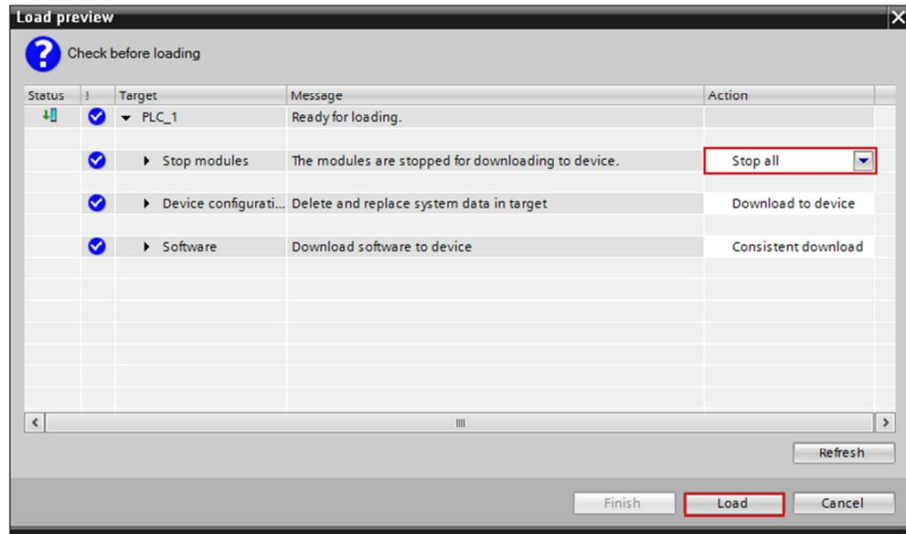
The dialog box containing the results of the download procedure opens. If the S7-1200 is in "STOP" mode for the download procedure, check the "Start all" check box. Click the "Finish" button. The status LED of the S7-1200 CPU indicates the "RUN" mode after downloading.
