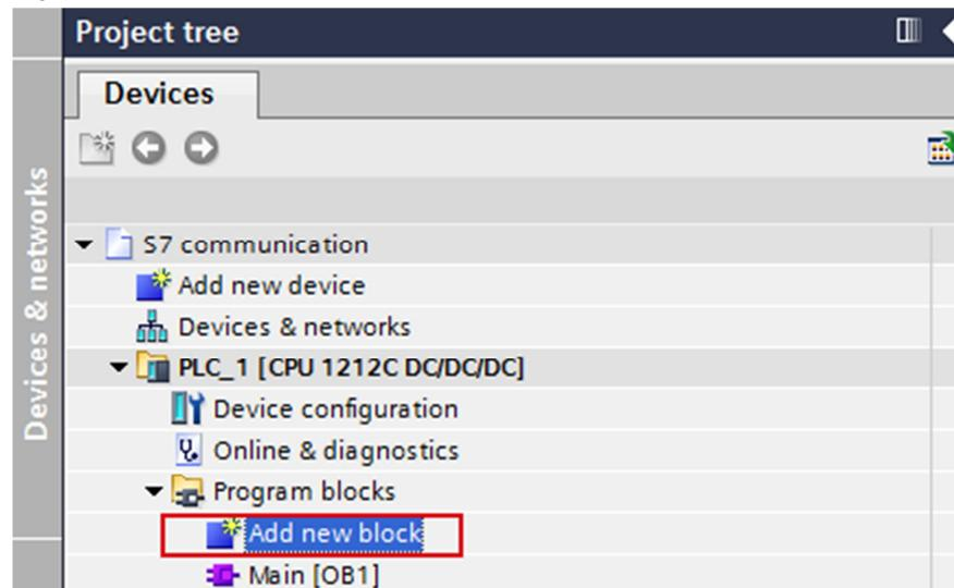
Click the "DB Data block" button. Enter the name of the data block and enable the "Manual" option to assign the number of the data block manually. If you enable the "Automatic" option, the number of the data block is assigned automatically.
