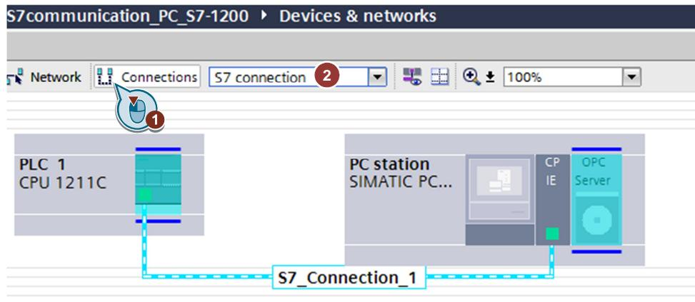
1. In the graphical area of the Network View, click the OPC server in the PC station and connect it to the S7-1200 CPU.
