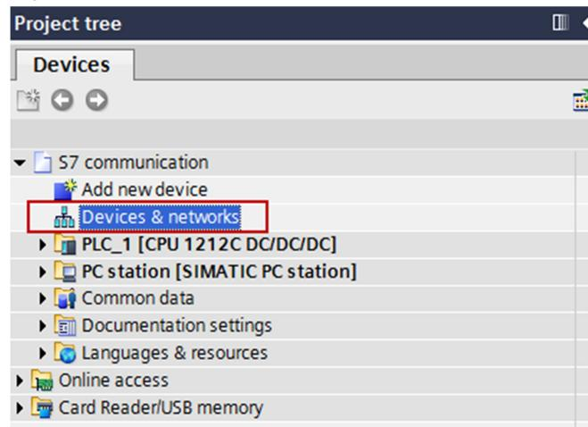
In the Network View or Device View of the Devices and Networks editor you click the PROFINET interface of the network card in the PC station.
