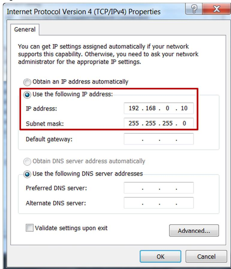
**NOTE** The IP address configured for the PC station in the TIA Portal must match the IP address set in Windows.
