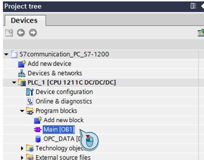
Create the program as shown in [Figure 3-14](#). The bit links are in the "Instructions" task card under "Basic instructions > Bit links".
