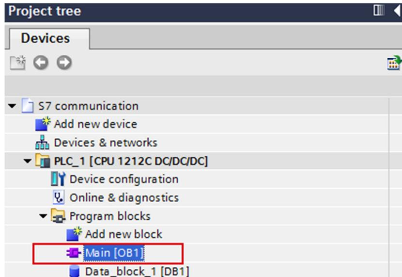
Create the program as shown in [Figure 2-14](#). The bit links are in the "Instructions" task card under "Basic instructions > Bit links".
