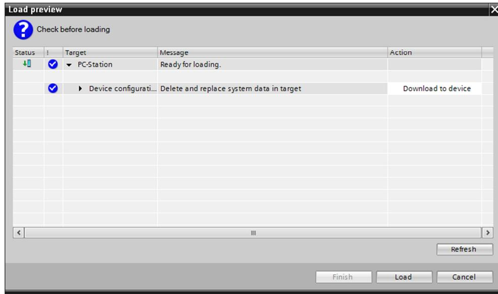
Commissioning of the PC station is completed after downloading of the configuration.
