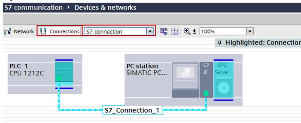
In the graphical area of the Network View, click the OPC server in the PC station and connect it to the S7-1200 CPU.
