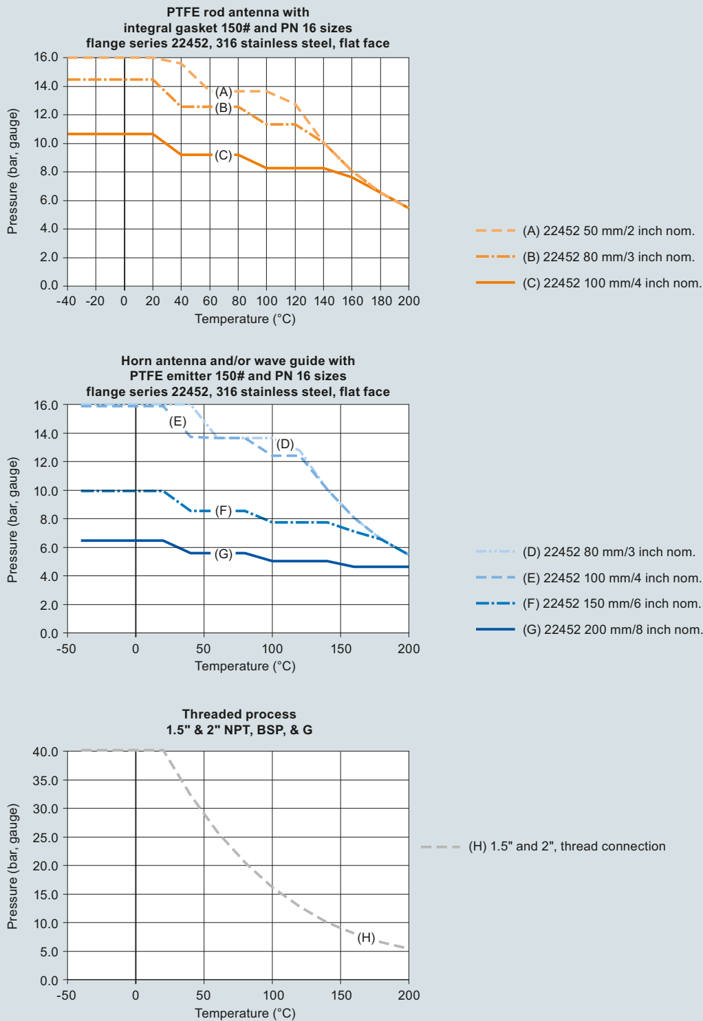
SITRANS LR200 process pressure/temperature derating curves
