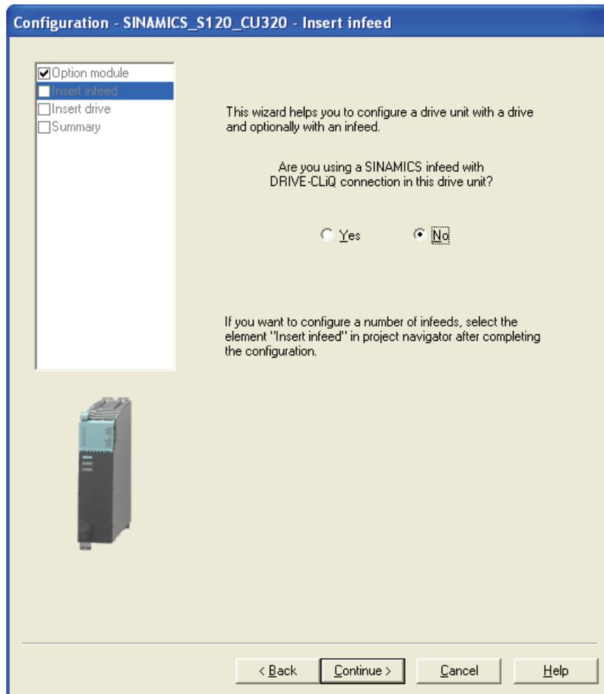
For modules with DRIVE-CLiQ infeed, proceed as for the configuration with Active Line Modules (ALM).
