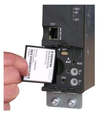
Figure 2-11 Slot for memory card
