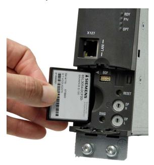
Figure 2-6 Slot for memory card
