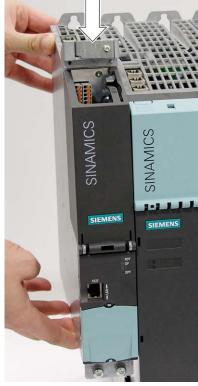
Push the Control Unit downwards until it latches into place
