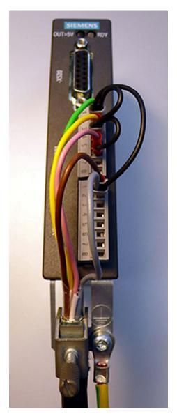
Figure 4-15 Photo of connection example 2: SMC30, 30 mm wide
