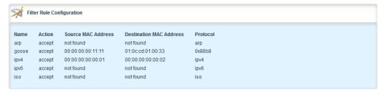
Figure 11.16 Filter Rule Configuration Table
