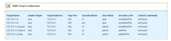
Figure 14.15 SNMPv3 Target Configuration Table
