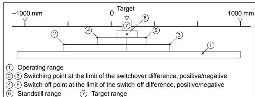
Figure 2-2 Ranges and Switching Points Around the Target
