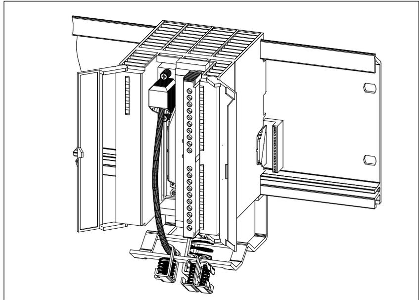
Figure 4-5 Connection of an Encoder to the FM 351 Positioning Function Module
