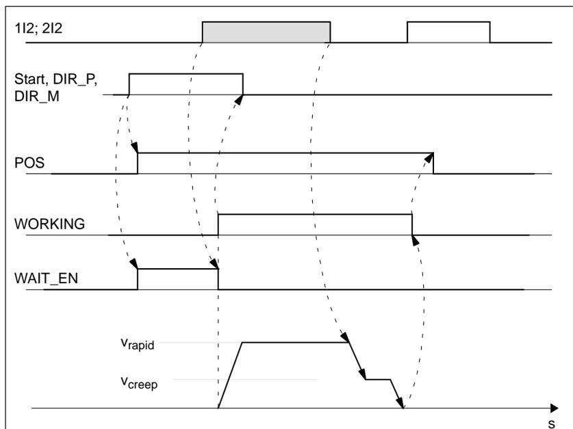
Figure 9-3 Starting the Incremental Mode
