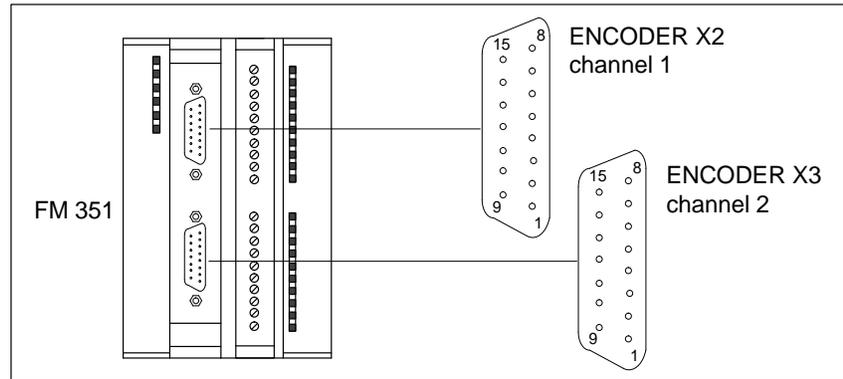
Figure 4-4 Position of the Subminiature Cannon Sockets X2 and X3
