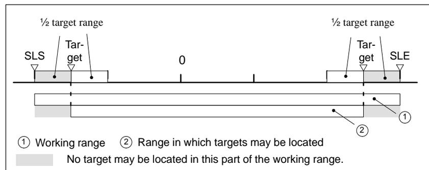
Figure 8-1 Limits for Entry of Incremental Dimensions
