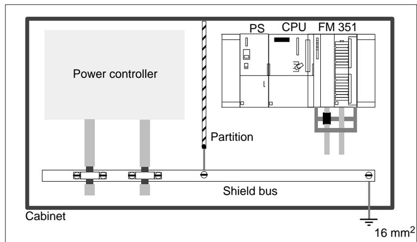
Figure 4-2 Installation in a Cabinet
