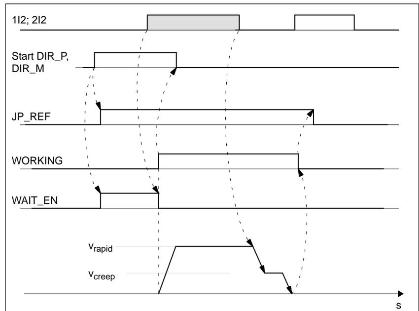
Figure 9-2 Starting a Seek-Reference-Point Traverse
