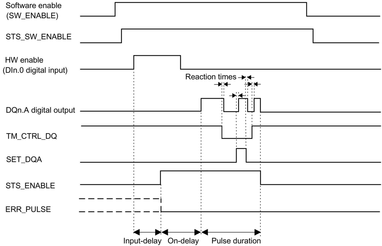
Figure 3-15 Direct control of DQ timing during Pulse output mode
