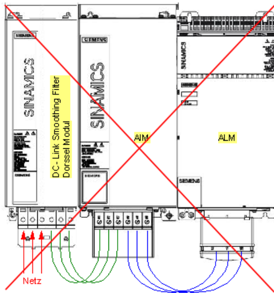
Figure 9-19 Impermissible connection of the line filter with the ALM without intermediate connection of the SF Choke Module
