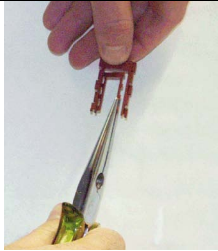
Adjust the shock-hazard protection using a suitable tool.
