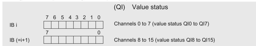
Figure 4-1 Address space for configuration as 16-channel DQ 16x24VDC/0.5A HF with value status
