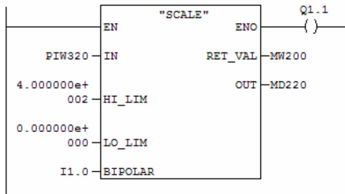
Because there is no contact in the rung, the controller executes FC105 on every scan cycle:
