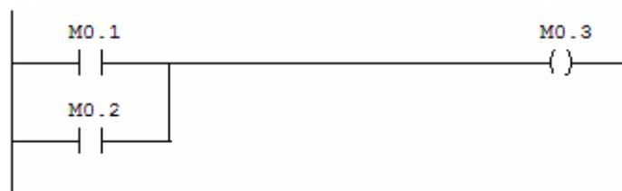
By setting M0.3 to 1 (on), FC41 reports that an out-of range condition has been detected:
