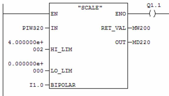
Because there is no contact in the rung, the controller executes FC105 on every scan cycle:
