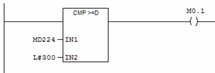
The Compare instruction ( $CMP \leq D$ ) checks to see whether the scaled value is above the higher limit of the operating range.
