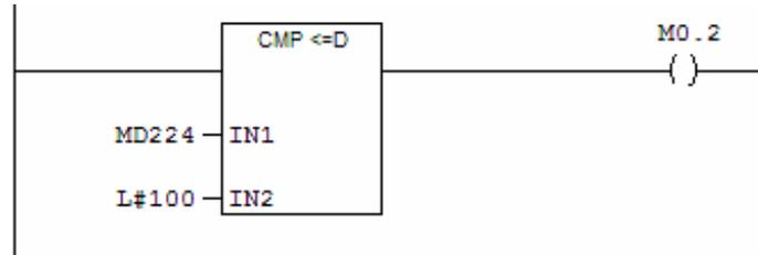
The Compare instruction (CMP <=D) checks whether the scaled value is below the lower limit of the operating range.
