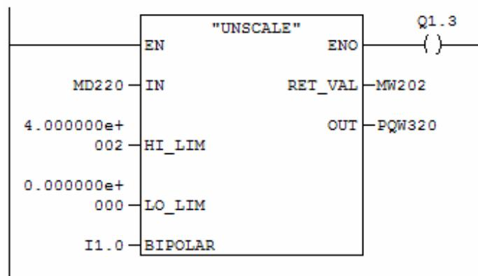
Because there is no contact in the rung, the controller executes FC106 on every scan cycle:
