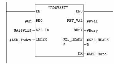
If SFC51 fails with SSL 0119, it returns -32638 (W#16#8082) in the RET\_VAL parameter. Network 3 checks the RET\_VAL. If W#16#0119 failed to get the LED status, FC112 calls SFC51 with SSL W#16#0174.
