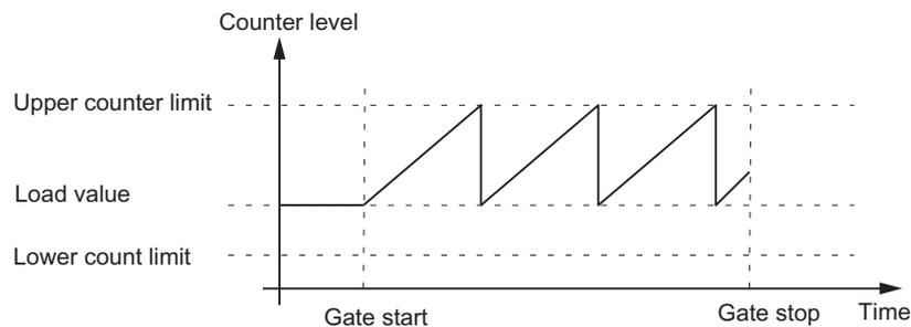
Figure 7-9 Periodic Counting with Load Value and Gate Control
