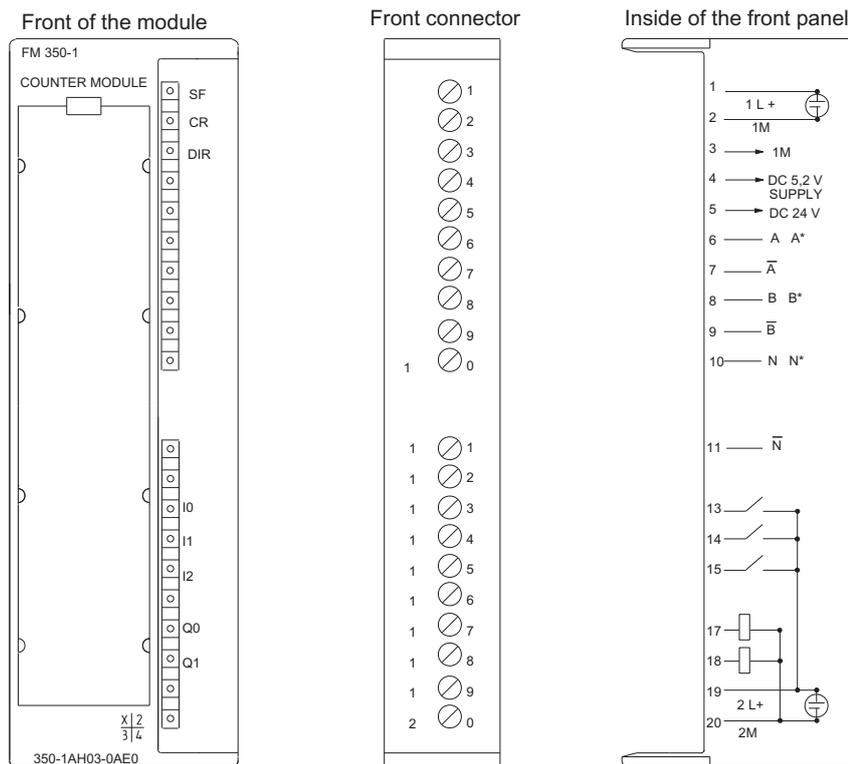
Figure 3-1 Front connector of the FM 350-1
