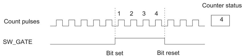
Figure 7-12 Opening and closing the software gate
