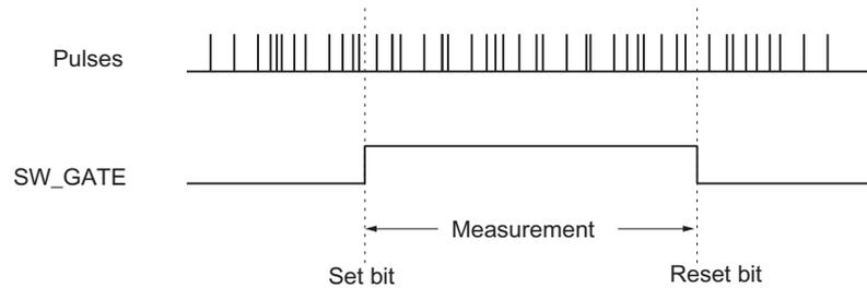
Figure 7-37 Opening and closing the SW gate
