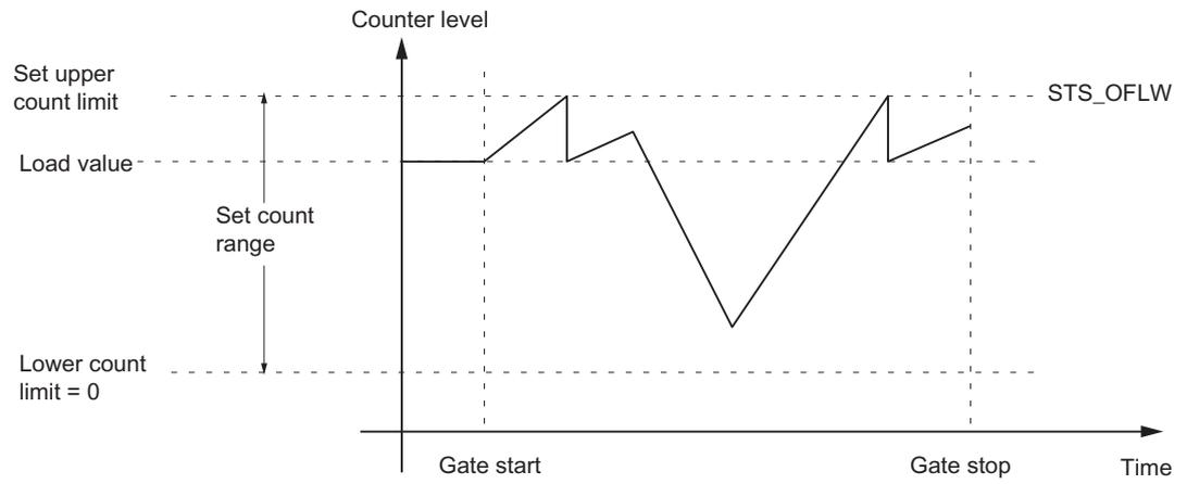
Figure 7-7 Periodic Counting With Main Count Direction Up
