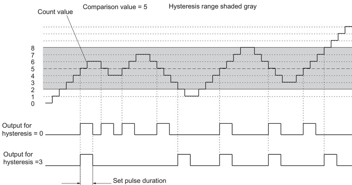
Figure 7-22 Example showing the effect of the hysteresis
