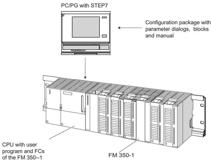
Figure 1-3 SIMATIC S7-300 configuration with an FM 350-1
