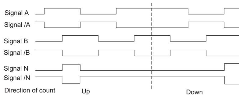
Figure 8-1 Signals of the 5-V incremental encoder
