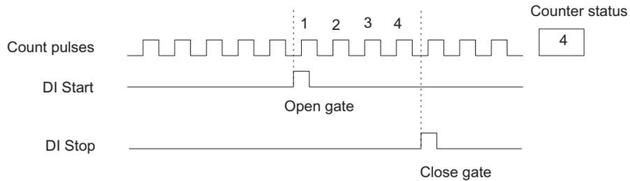
Figure 7-11 Edge-triggered opening and closing of the HW gate
