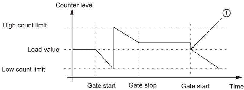
Figure 7-13 Continuous down count, canceling gate function
