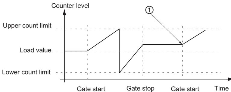
Figure 7-14 Continuous up count, interrupting gate function
