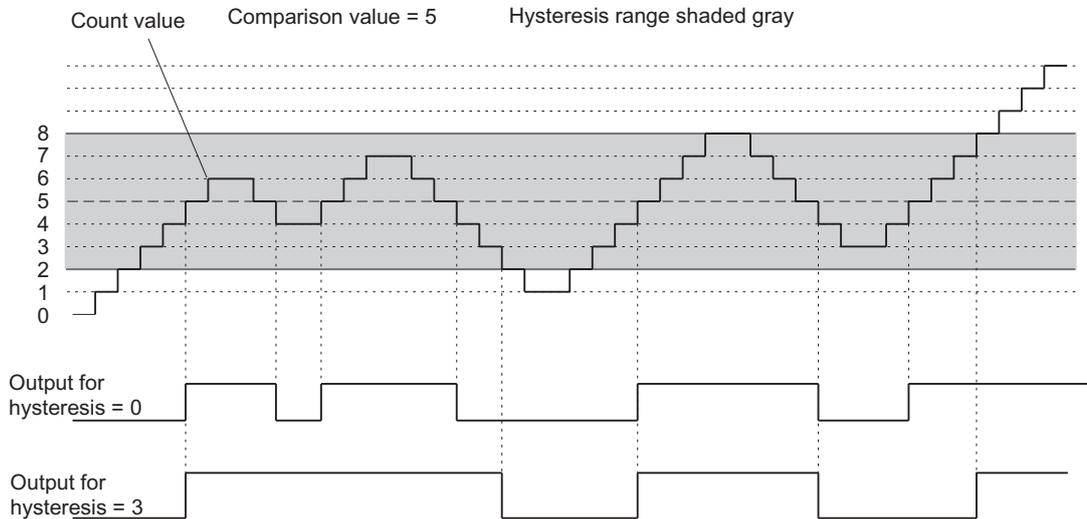
Figure 7-20 Example showing the effect of the hysteresis
