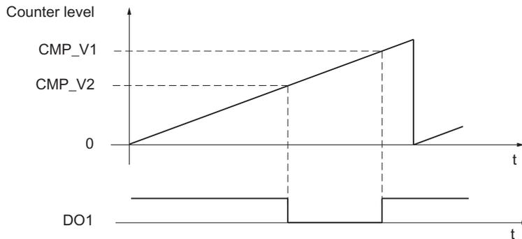
Figure 7-18 At the start of the counting process,  $V2 < V1$
