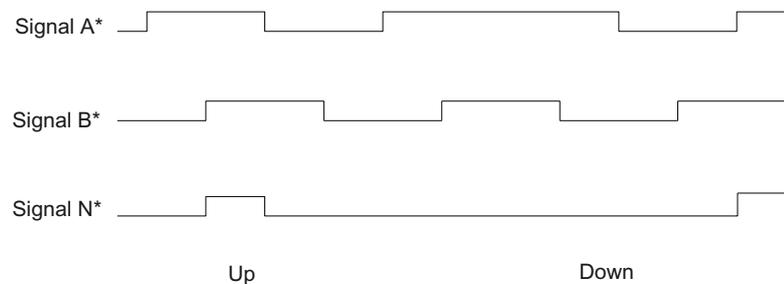
Figure 8-2 Signals of the 24-V incremental encoder
