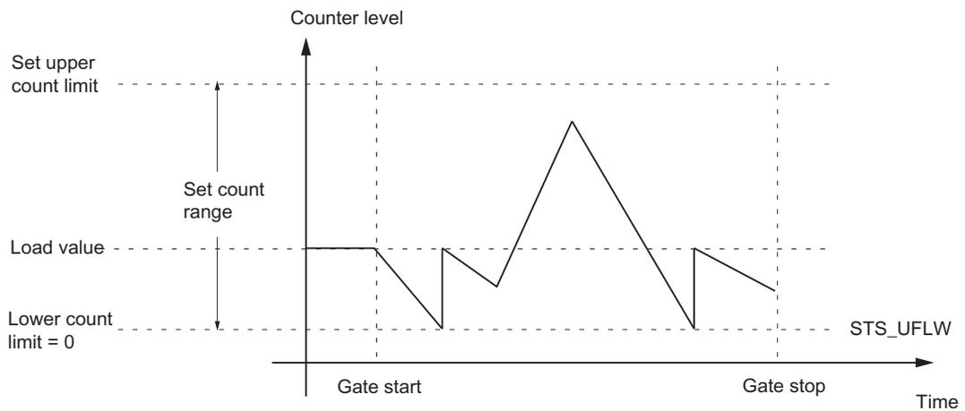
Figure 7-8 Periodic Counting With Main Count Direction Down
