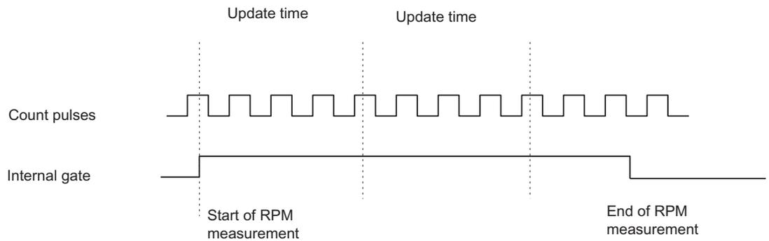
Figure 7-33 RPM Measurement with Gate Function
