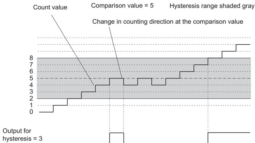
Figure 7-21 Example of a hysteresis for a change of direction at the comparison value
