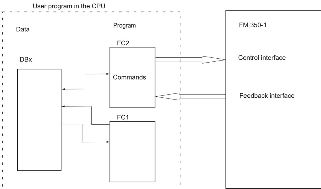
Figure 5-1 Exchange of Data between the User Program and FM 350-1 with FC`s (Example)
