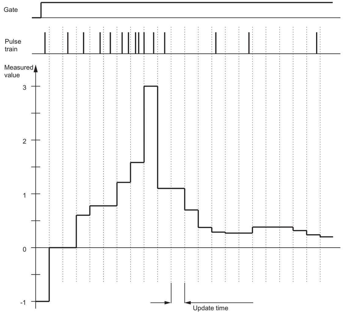
Figure 7-30 Principle of continuous measurement (example frequency measurement)
