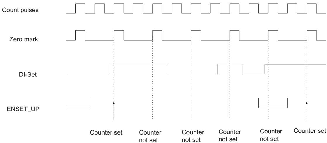
Figure 7-25 Single Setting of the Counter with the Zero Mark
