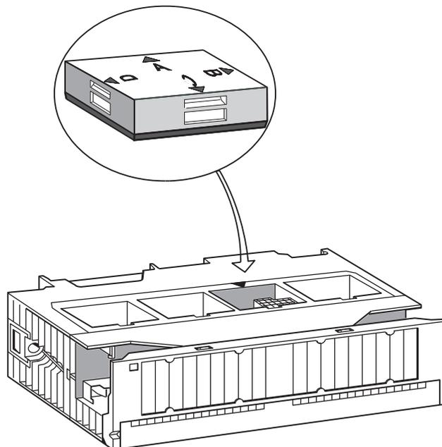
Figure 2-1 Installing the coding plug
