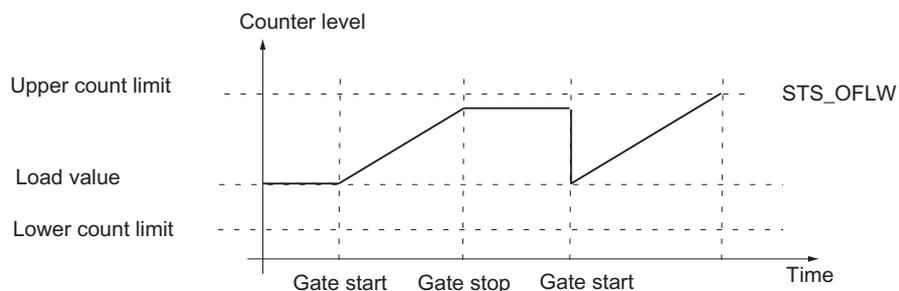
Figure 7-5 Single Counting with Load Value and gate control
