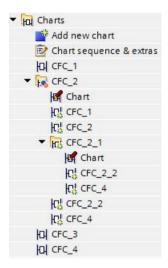
The chart "CFC\_2" is a basic chart that contains the subcharts "CFC\_1", "CFC\_2\_1", "CFC\_2\_1", "CFC\_2\_2" and "CFC\_4".
