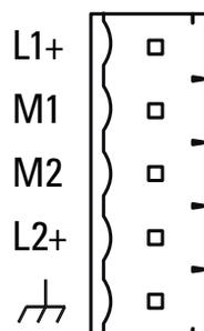
Figure 4-1 Socket of the external power supply
