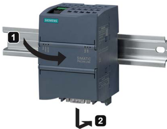
Figure 8-1 PN/CAN LINK DIN rail mounting
