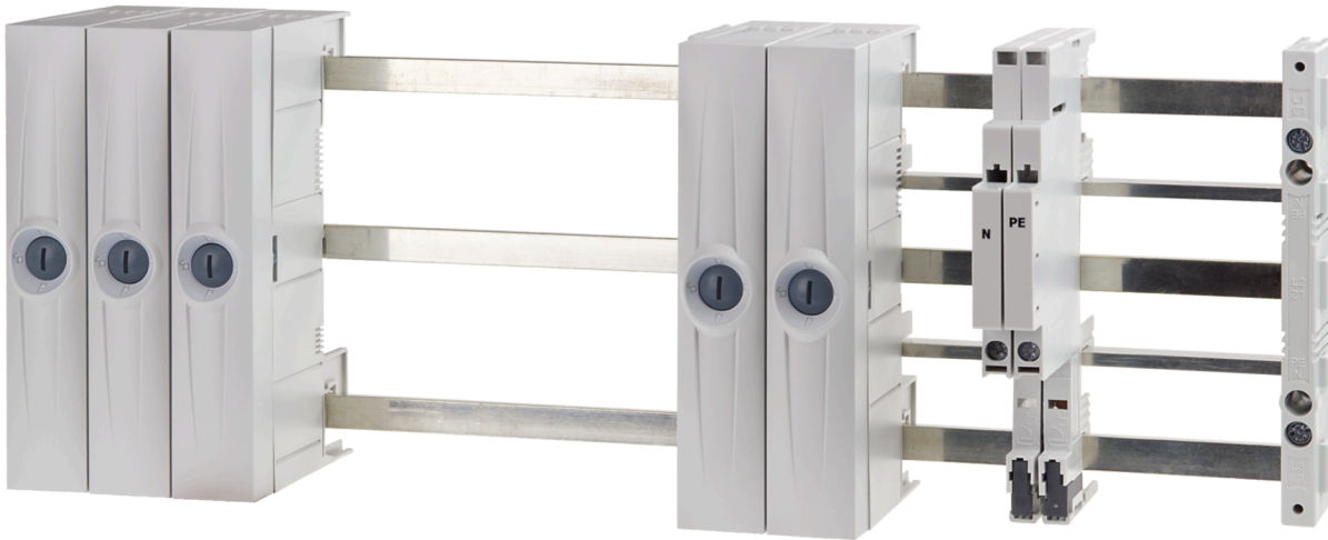
Figure 3-2 The 3-/5-pole 60 mm compact busbar system for the lower performance range up to 360 A; the 5-pole element is only designed for up to 200 A
