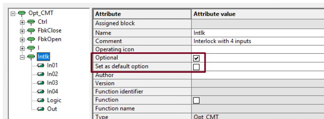
The alternative is a continuation of the variant. This allows you to configure "either/or variants". This is necessary if a block input will be configured with different connections depending on the variation. The instance must decide on an alternative.
