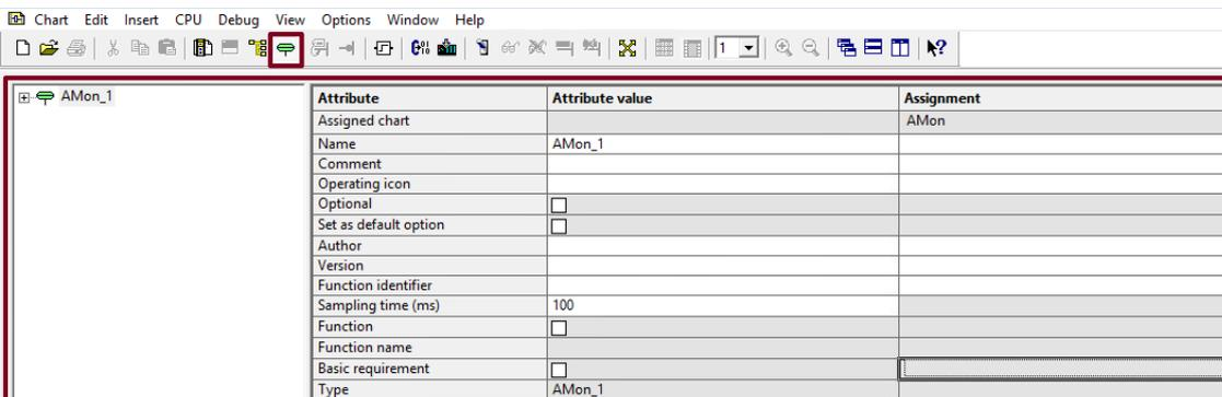
2. Enter the corresponding plan name in the "Assignment" column in the "Name" area.
