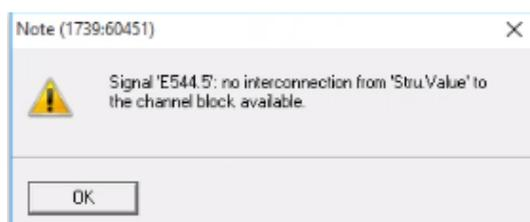
To make additional blocks known to the system as driver blocks, these must be entered in the XML "SignalBlocksAPL\_90" (\Siemens\STEP7\S7data\SignalProcessing).
