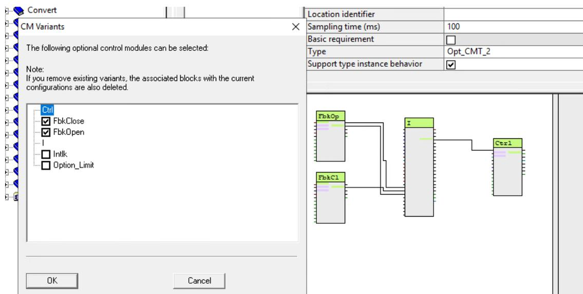
If an option is used with almost all instances, it can also be enabled by default. If an instance is created with "Set as default option" enabled, each new created instance will be activated with the option.
