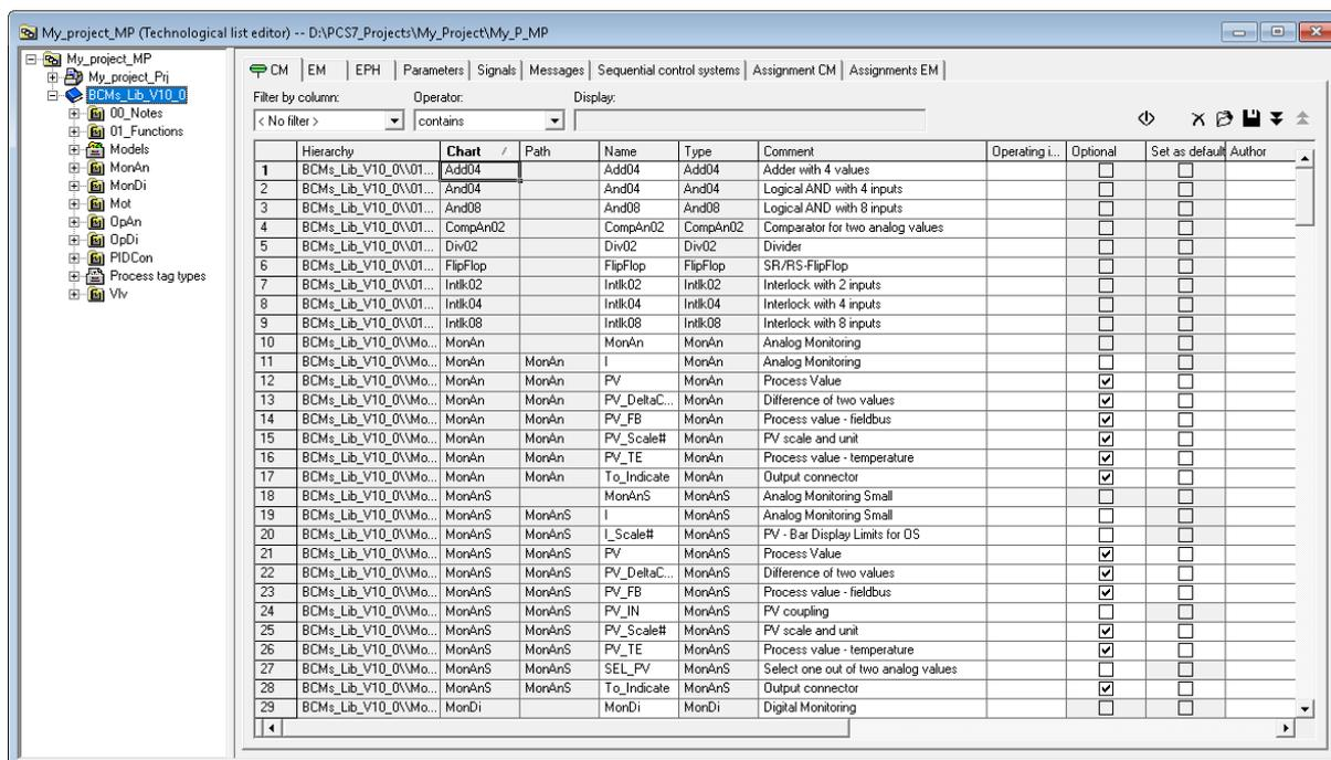
In the "Technological List Editor", the signals, parameters, and messages of CMs can be parameterized and CMs can be interconnected via the technological I/Os. In addition to parameterization and interconnection, CMTs can also declare blocks as optional.
