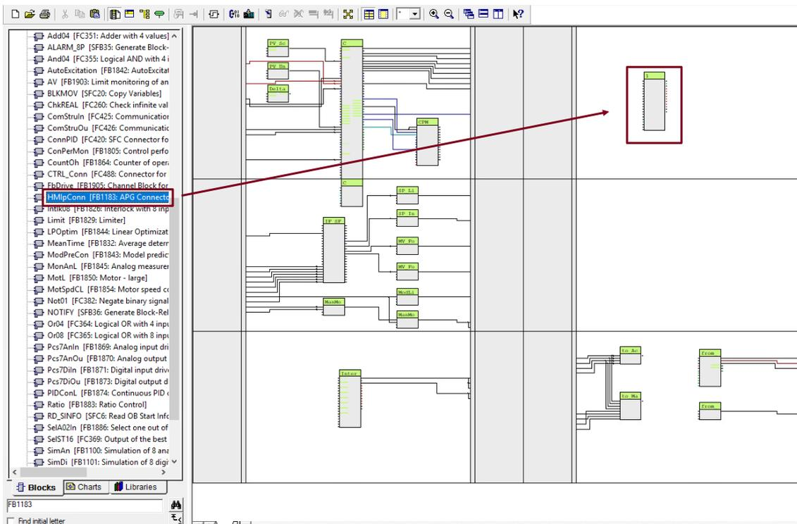
4. Connect the "ReadPointer" input of the "HMIPConn" block to an output of the "PIDConL" block.
