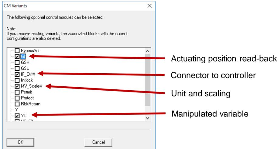
If you cannot imagine an exact function under the individual selection points, then you receive a complete overview of the interconnected blocks and configured technological I/Os in the CMT. You can find the assigned CMT in the object properties of the CFC.
