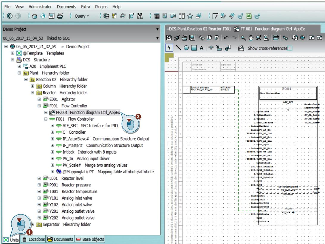
13. Drag the function from the folder "<Project name> > Templates > Template container > Functions" into the "Function diagram".
