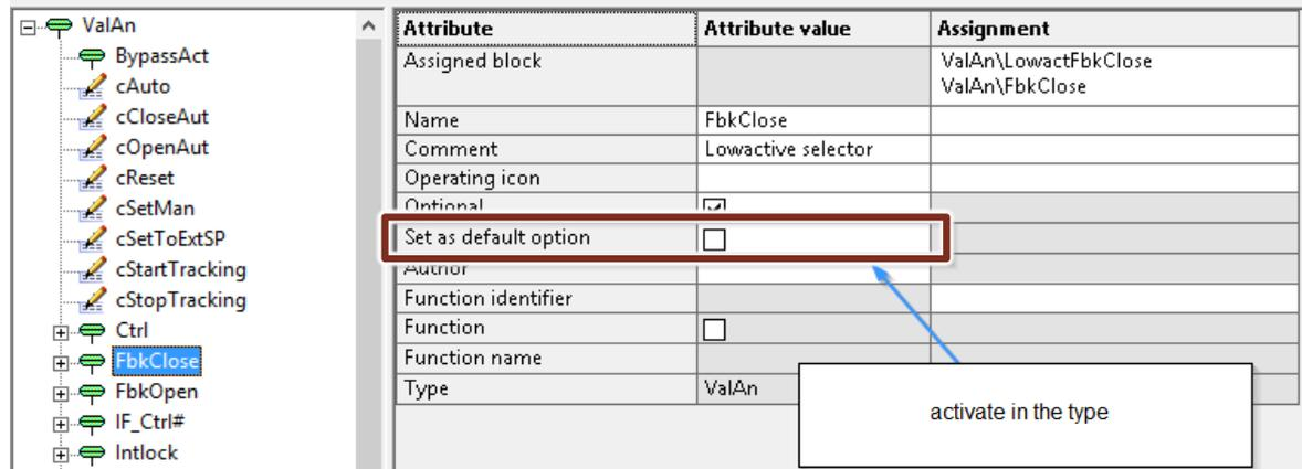
2. To create variants, activate the optional attribute for the CM "DeltaCalc", "PV\_FB\_In", "PV\_In" and "PV\_TE\_In".
