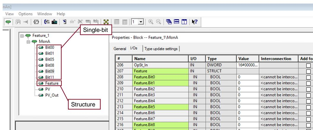
In order to keep the function plans (FBD) in COMOS/PAA clear, the bits can be switched to being invisible.
