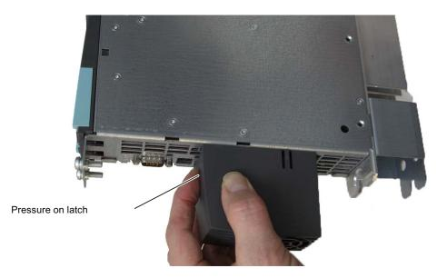
Figure 6-3 Unlatch the double fan/battery module
