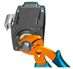
Figure 5-1 Mounting the feather key
