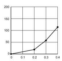
This calculation creates a piece-wise linear approximation of the level/flow curve, providing best results if the curve is non-linear and there are no sharp angles.
