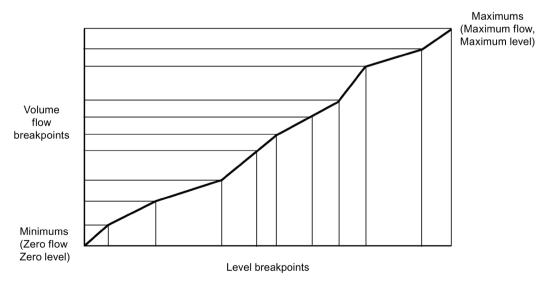
Characterization is achieved by entering the level and corresponding volume flow breakpoints, either from empirical measurement or from the manufacturer's specification.
