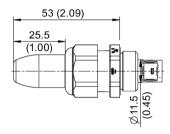
Figure C-1 Dimension drawing SITRANS AW050 Bluetooth adapter, dimensions in mm (inch)
