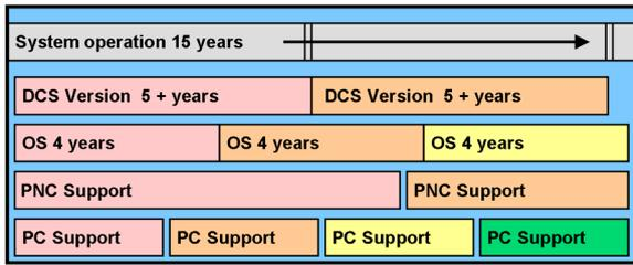
Example of typical replacement intervals for key process components during the operating time<sup>5</sup>
