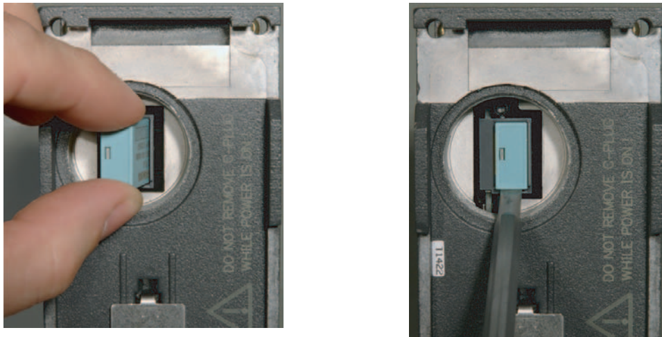
Figure 2-7 Inserting the C-PLUG in the device and removing the C-PLUG from the device with a screwdriver
