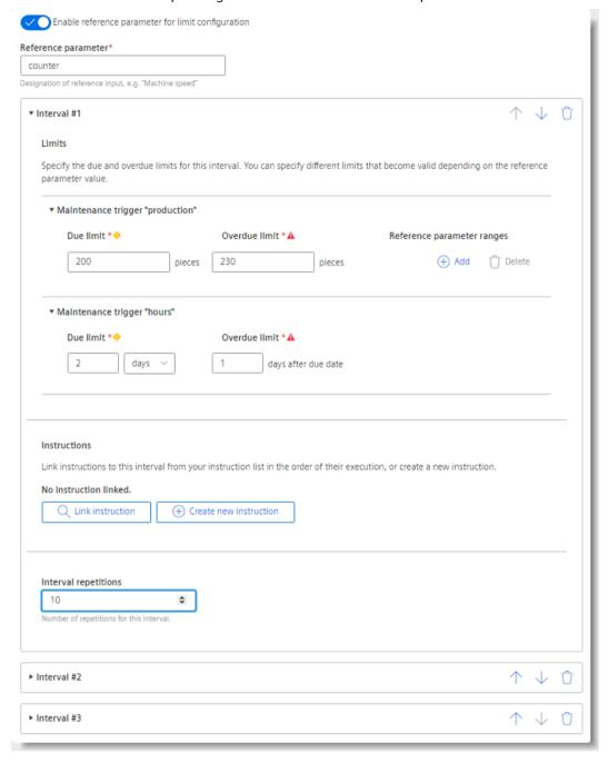
Example: Define "Machine speed" as reference parameter. Now you can define shorter maintenance intervals, for example, if your machine is operated at higher speeds.
