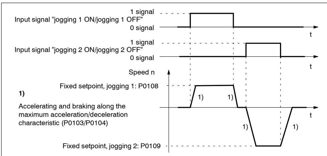
Fig. 6-25 Accelerating and braking when jogging
