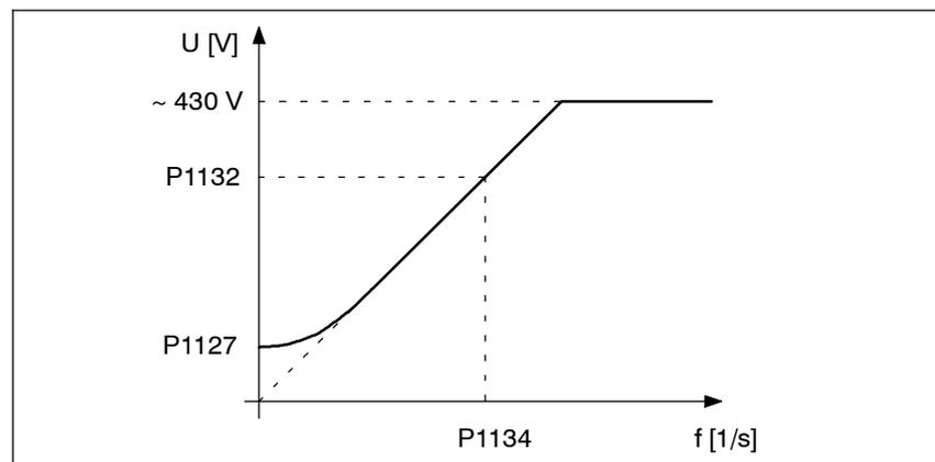
Fig. 7-12 V/Hz characteristic ARM
