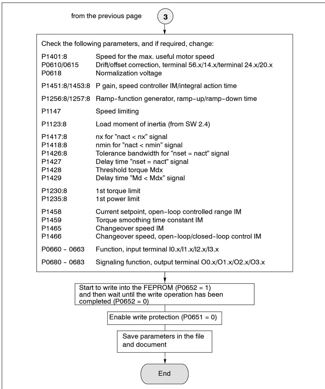
Fig. 4-9 Commissioning induction motors without encoder (Part 3)
