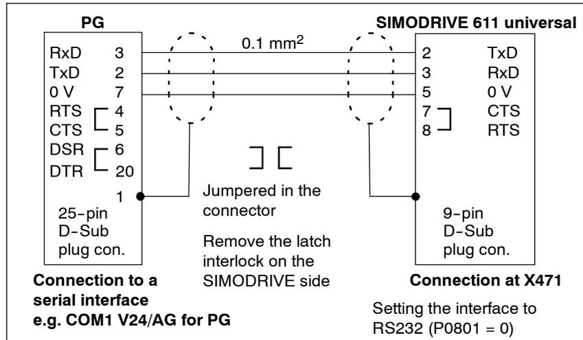
Fig. 2-13 RS232 connecting cable: PG <-> SIMODRIVE 611 universal
