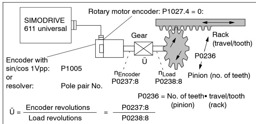
Fig. 6-11 Linear axis with rotary motor encoder (rack/pinion)
