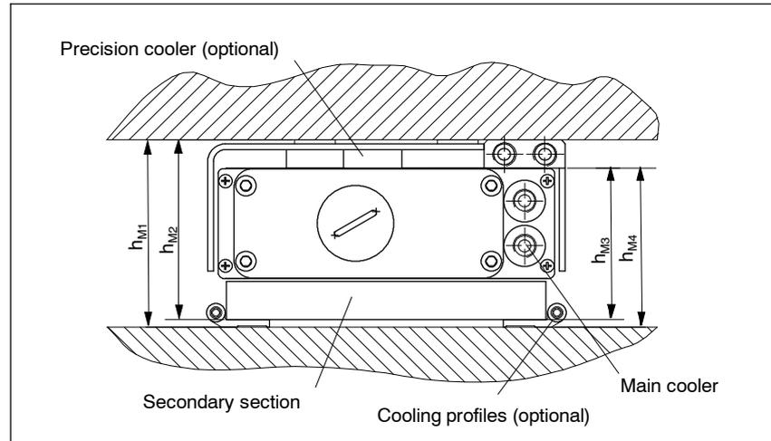
Fig. 4-16 Important dimensions when mounting the motor
