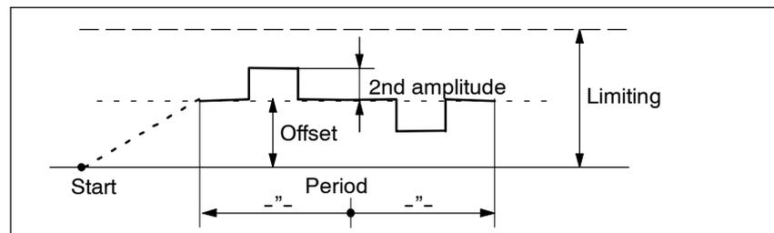
Fig. 7-6 "Staircase" waveform with amplitude = 0 and offset > amplitude 2
