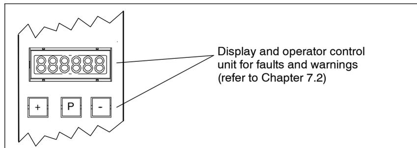
Fig. 5-23 Fault display on the control board
