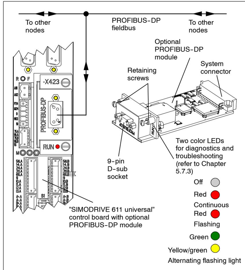
Fig. 5-3 "SIMODRIVE 611 universal" with optional PROFIBUS-DP module
