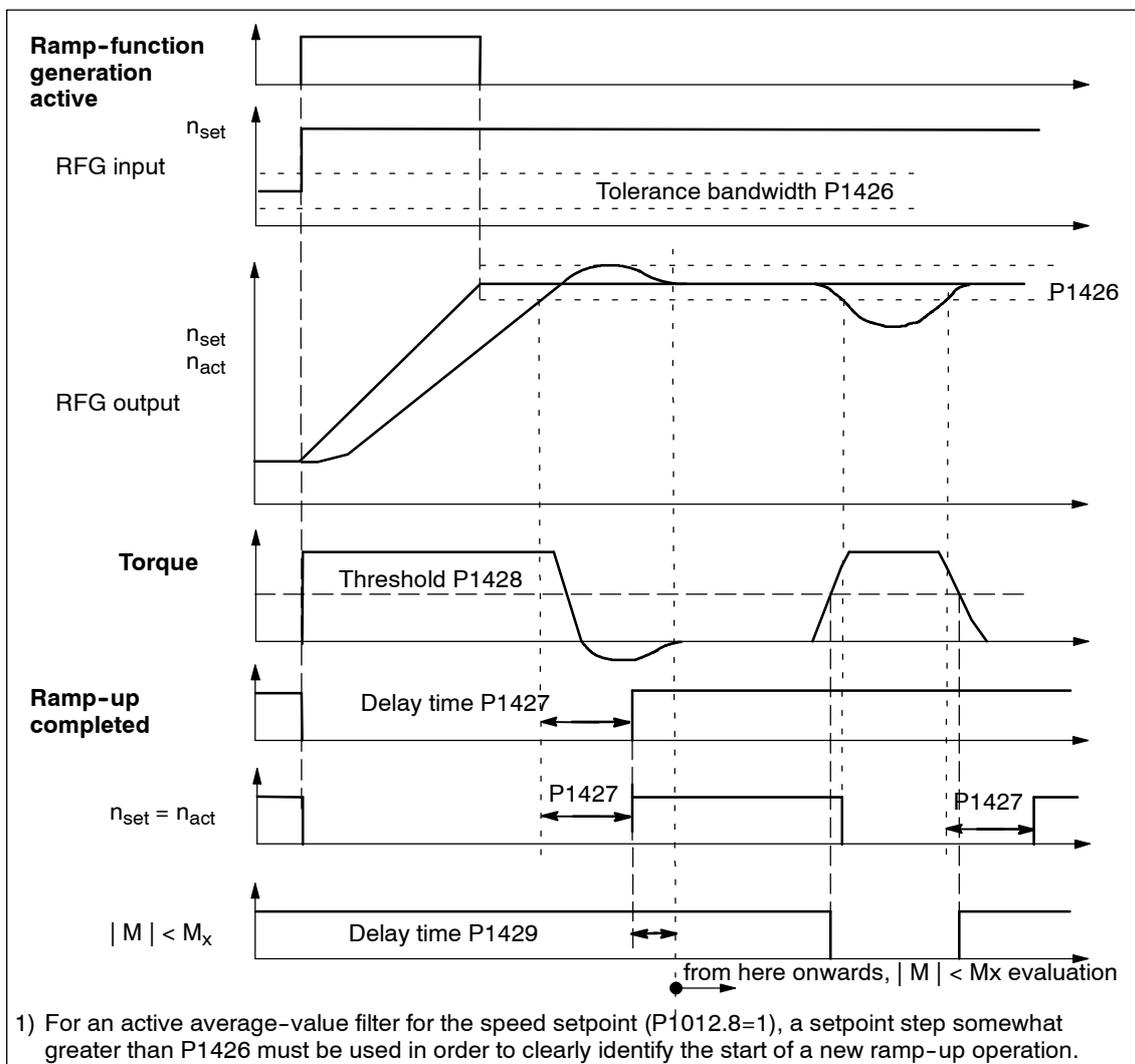
Fig. 6-5 Signal characteristics for the ramp-function generator
