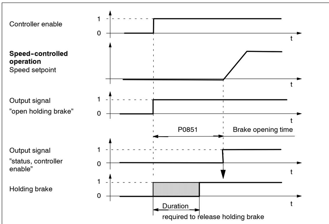
Fig. 6-82 Release brake: Characteristics when issuing "controller enable"
