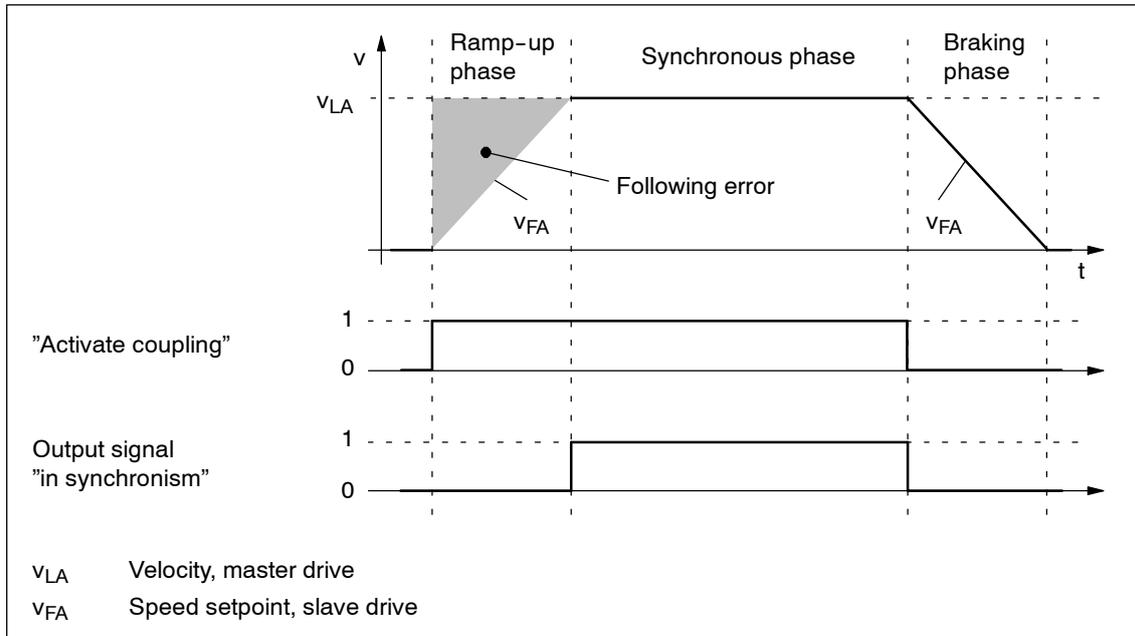
Fig. 6-35 Speed synchronism (P0410 = 1 or 3)
