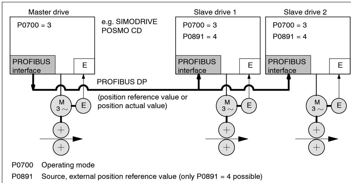
Fig. 6-34 Synchronous coupling between several DP slaves
