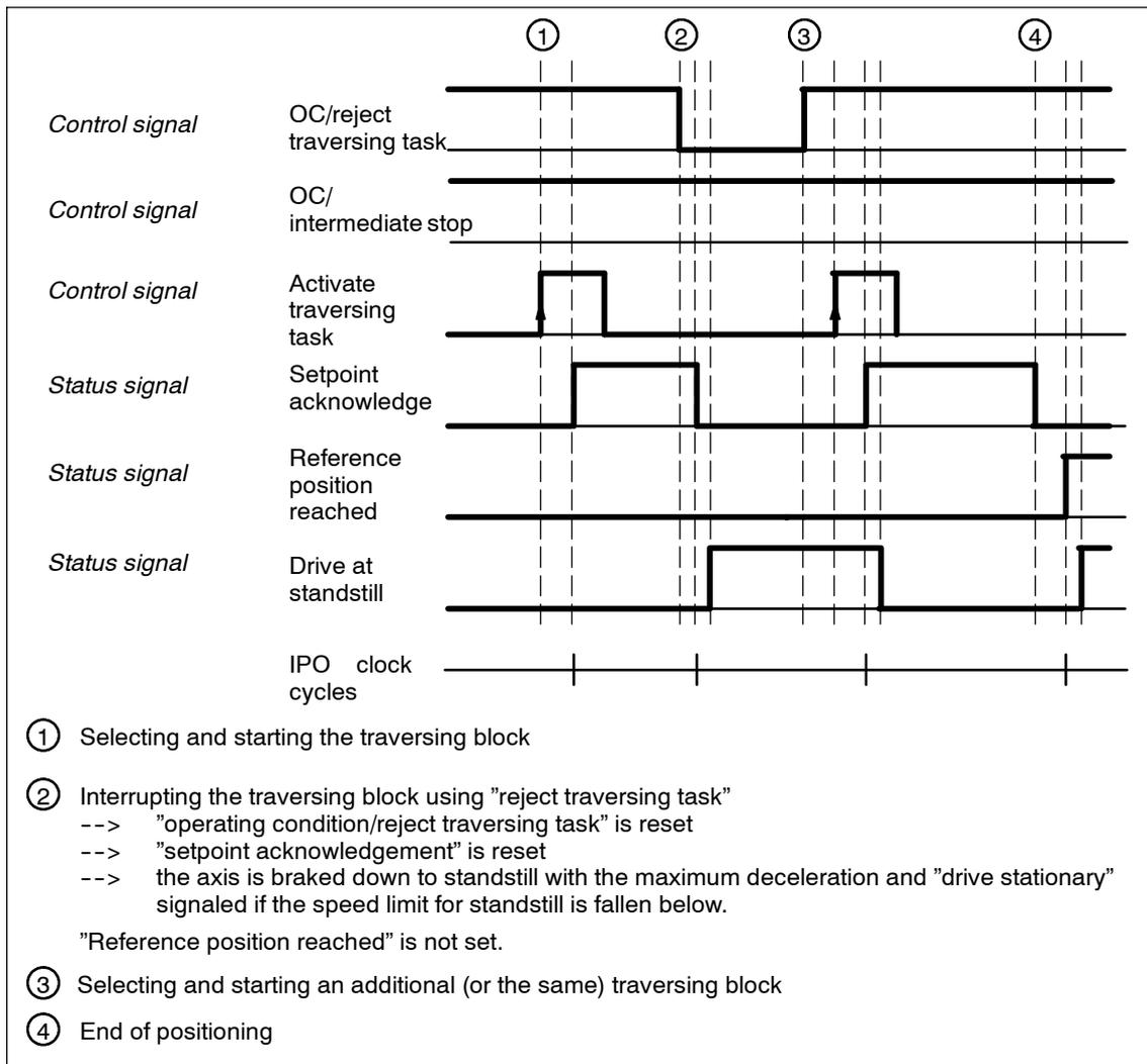
Fig. 6-29 Characteristics when aborting a traversing block
