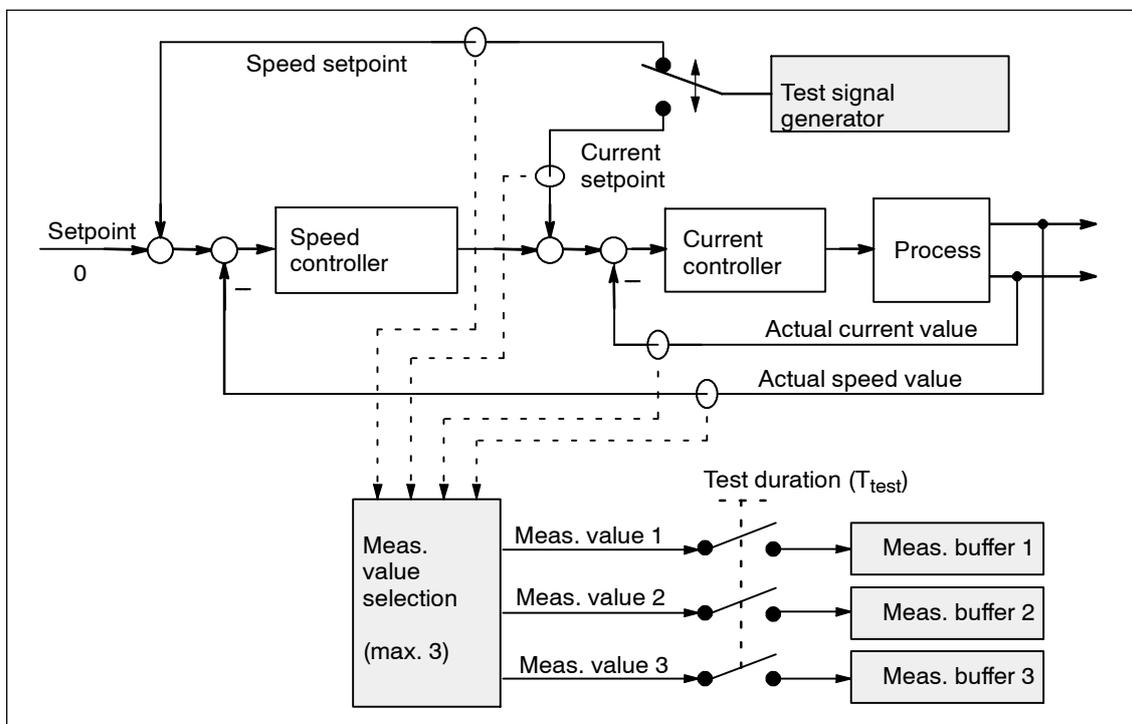
Fig. 7-11 Block diagram of the drive optimization (schematic)
