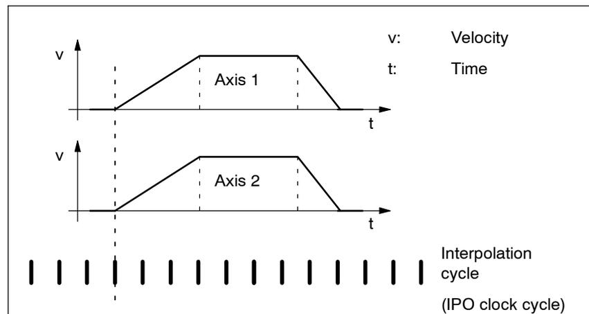
Fig. 5-27 Example: Simultaneously starting the traversing motion
