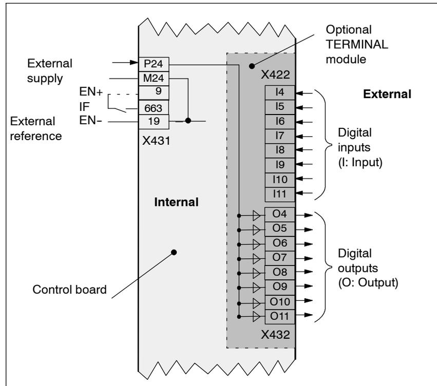
Fig. 2-8 Connection diagram for the optional TERMINAL module
