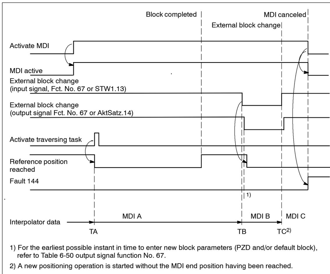
Fig. 6-30 Control and status signals for MDI
