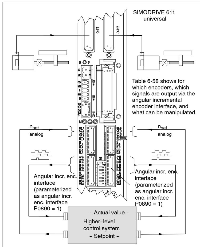
Fig. 6-74 Angular incremental encoder interface parameterized as output
