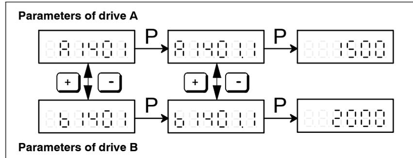
Fig. 3-6 Parameter display for drive A and B
