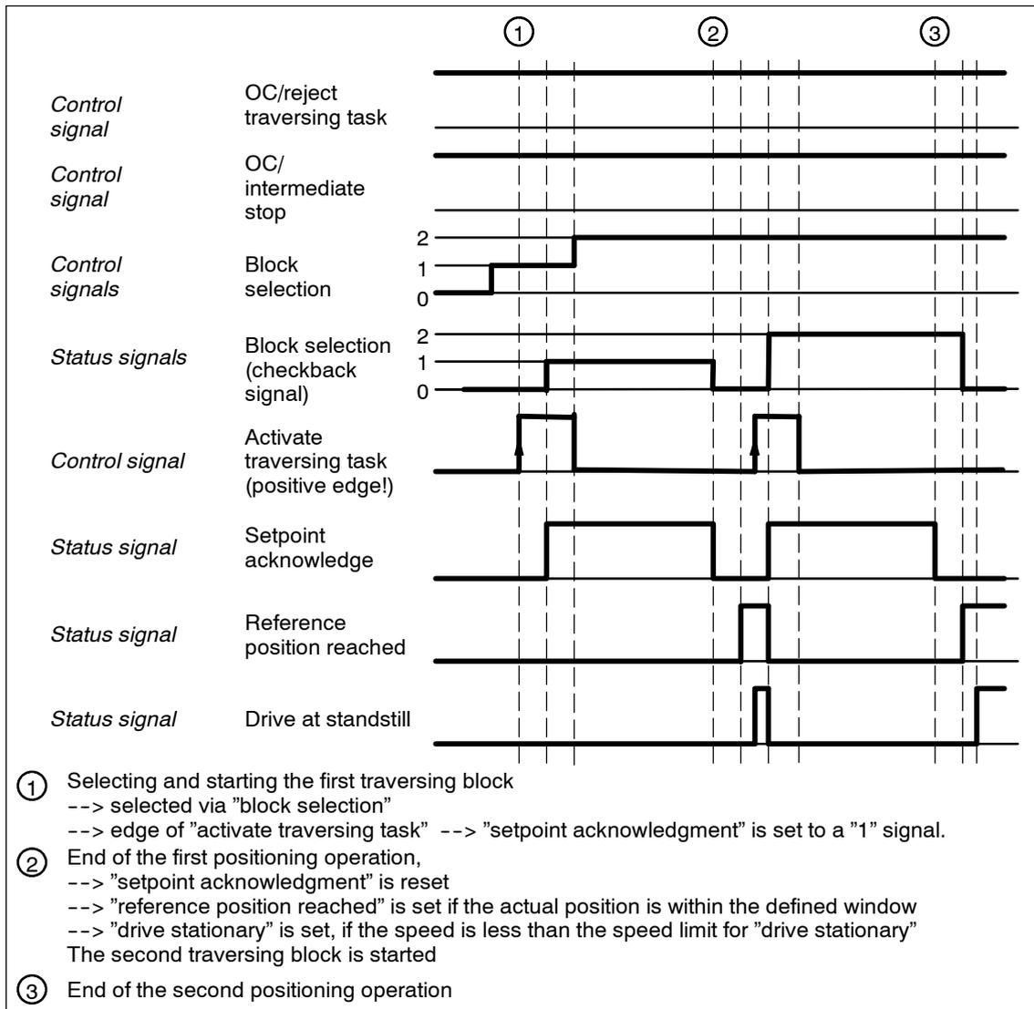
Fig. 6-27 Sequentially starting individual blocks
