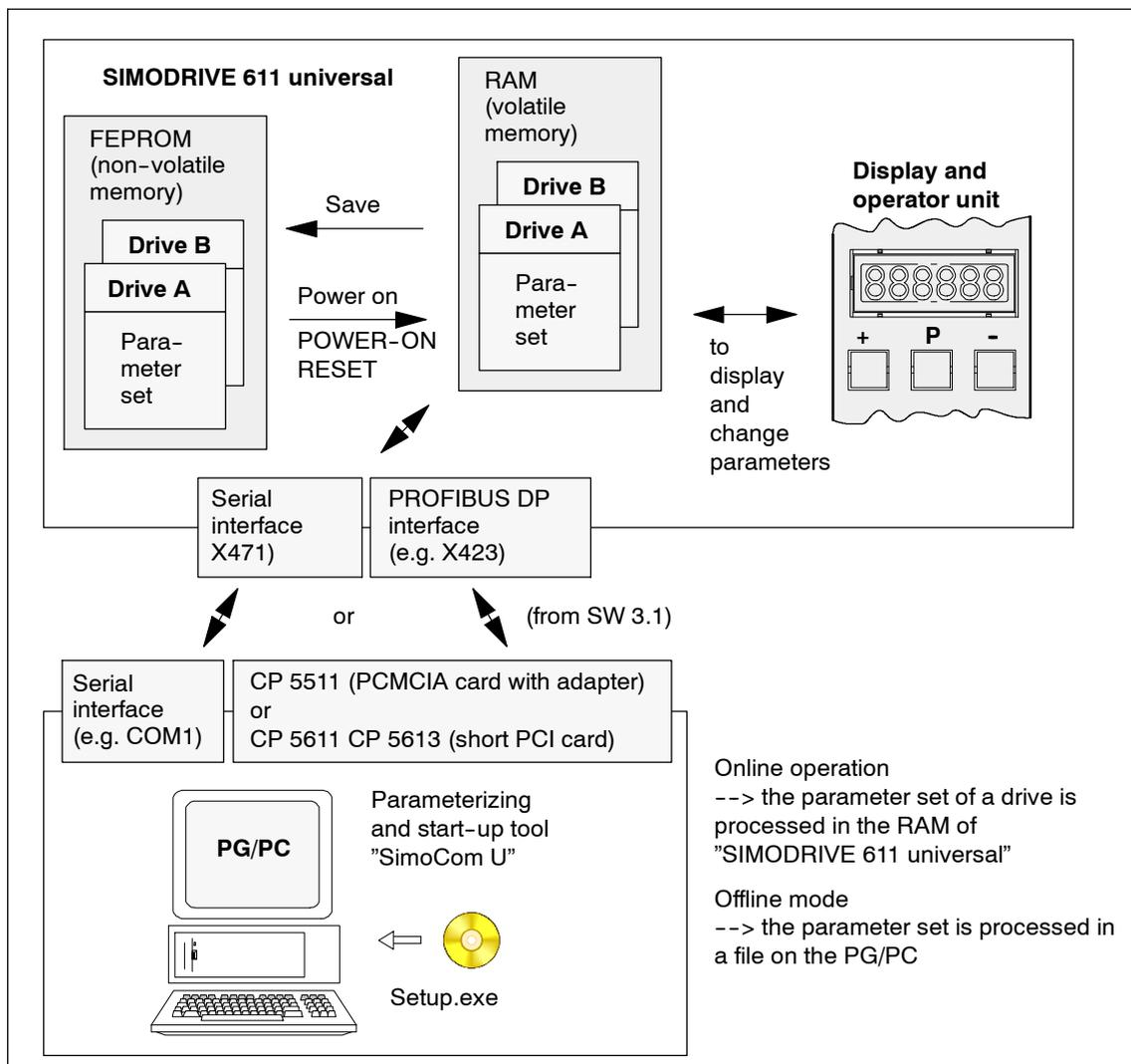
Fig. 3-1 Overview when parameterizing
