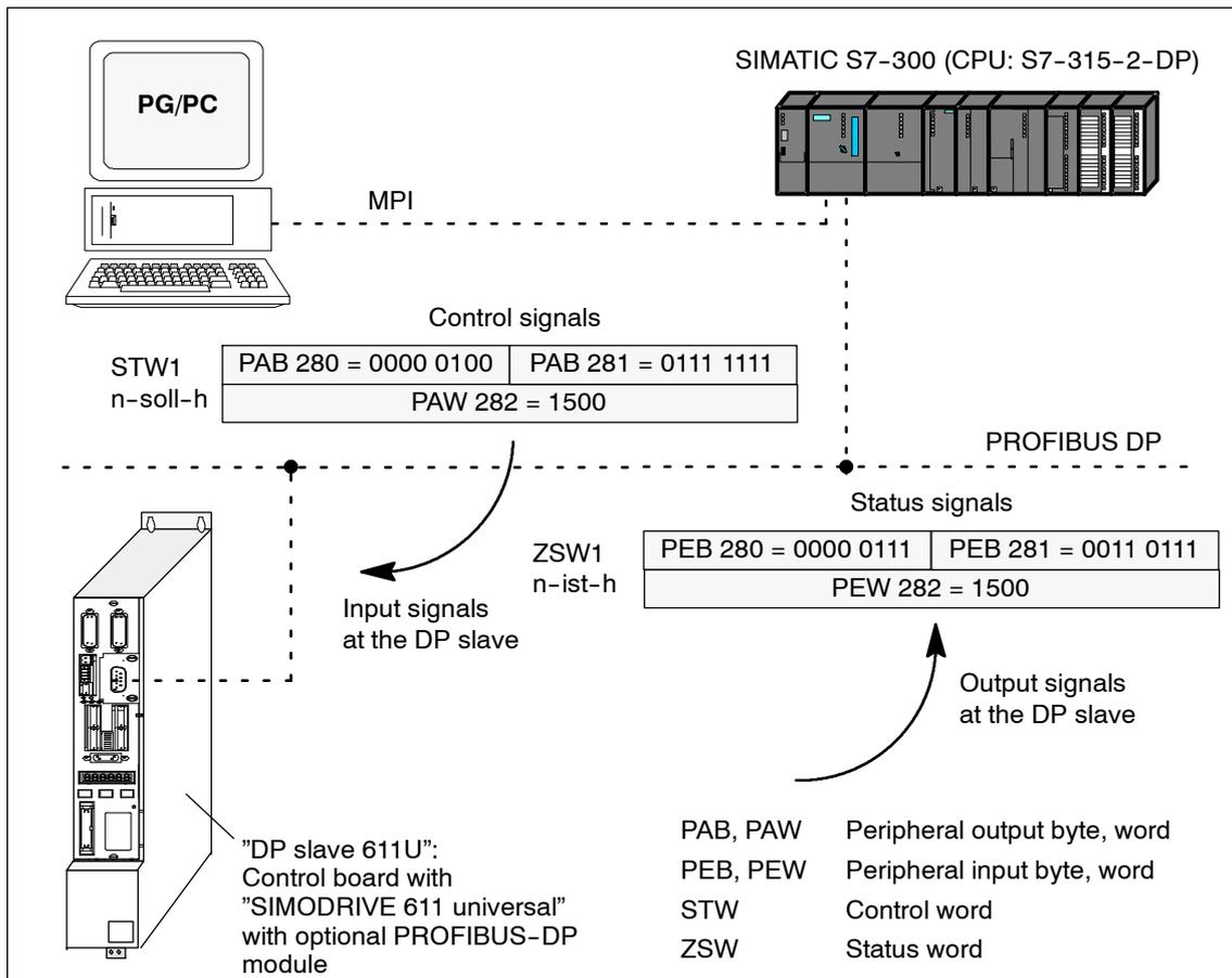
Fig. 5-19 Example: Operate the drive via PROFIBUS
