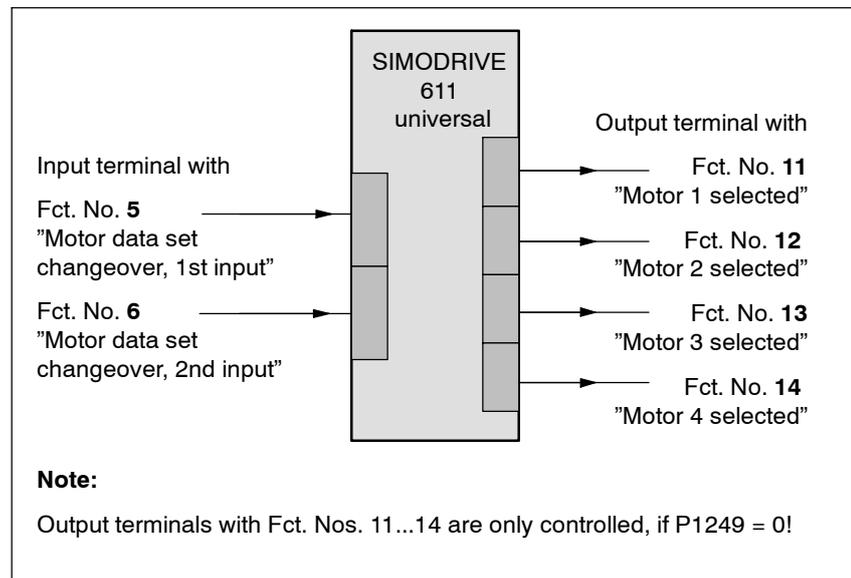
Fig. 6-87 Input/output signals: freely-parameterizable terminals
