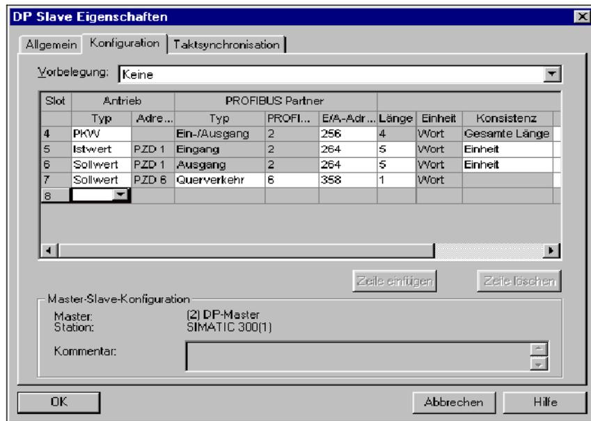
Fig. 6-45 Example, configuring the slave drive for S7
