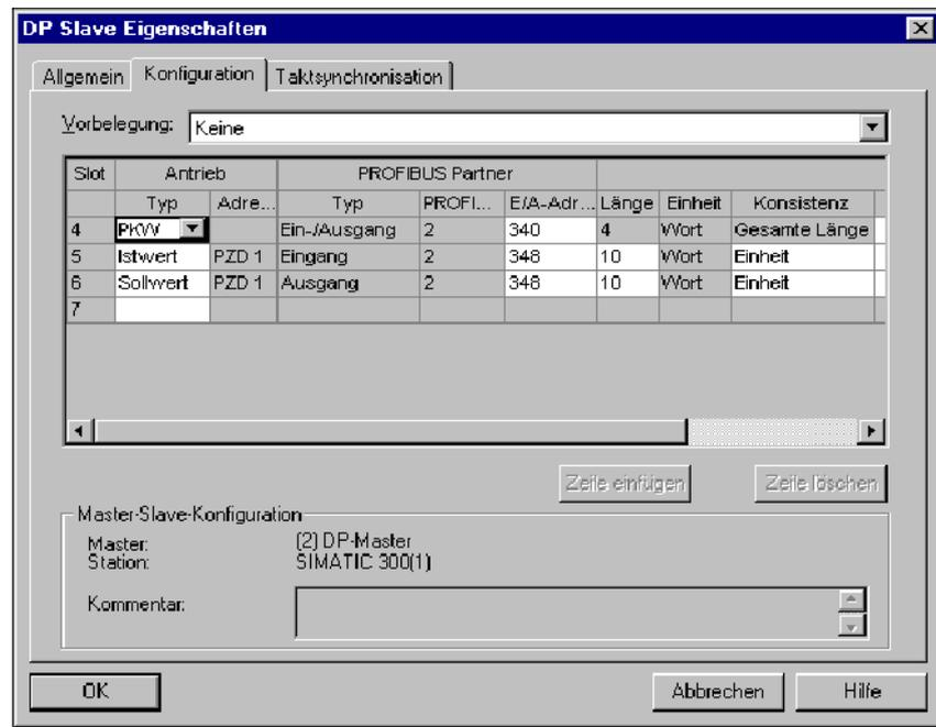
Fig. 5-35 Example, configuring the master drive for S7
