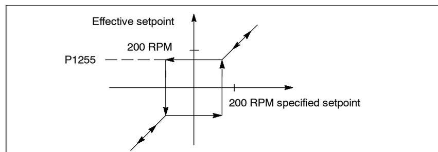
Fig. 6-8 Method of operation of the minimum speed
