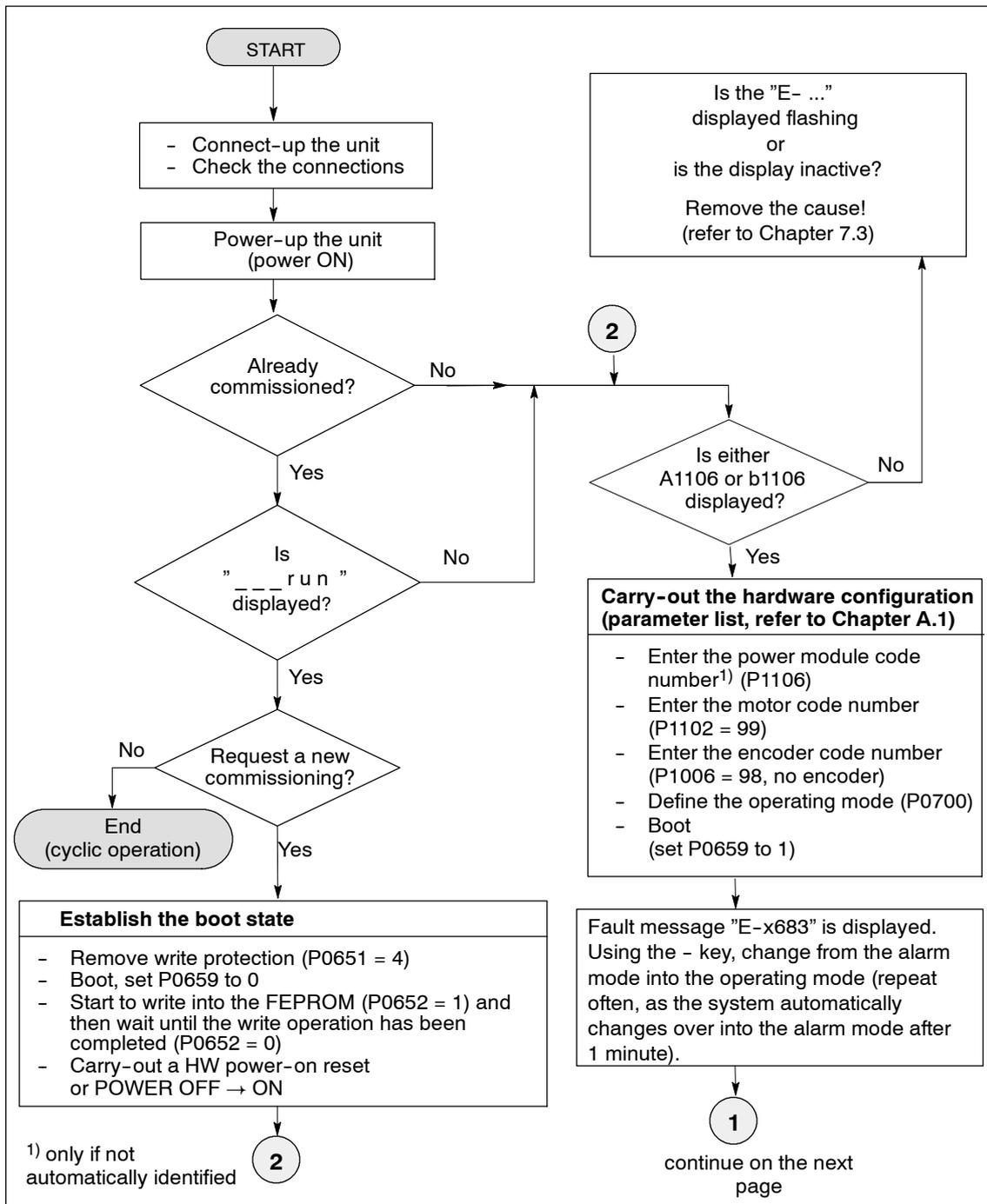
Fig. 4-7 Commissioning induction motors without encoder (Part 1)
