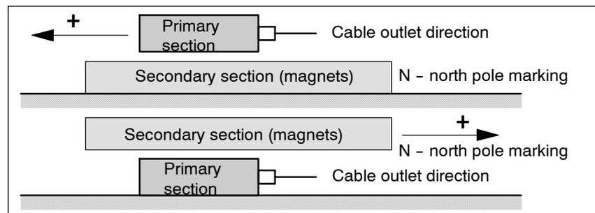
Fig. 4-18 Determining the positive direction of the drive
