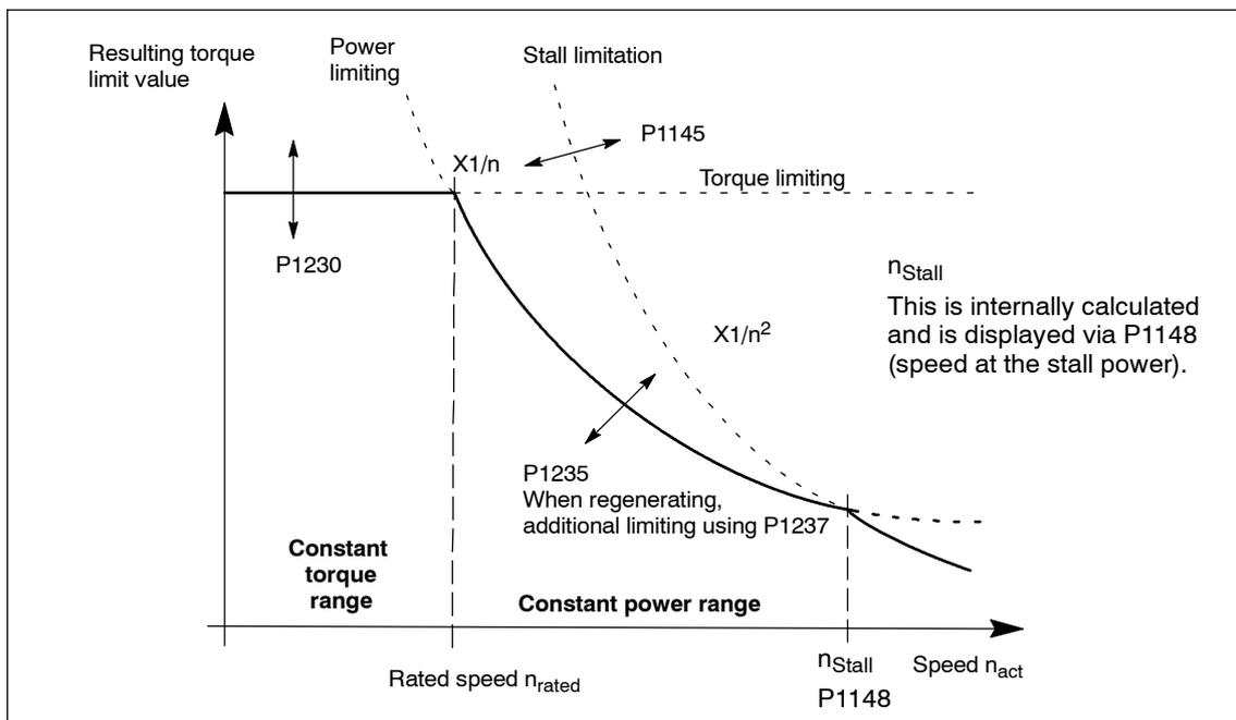
Fig. 6-7 Limiting the torque setpoint
