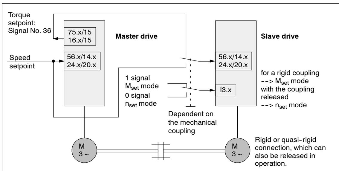
Fig. 6-66 Example: Coupling 2 drives with master/slave with analog I/O
