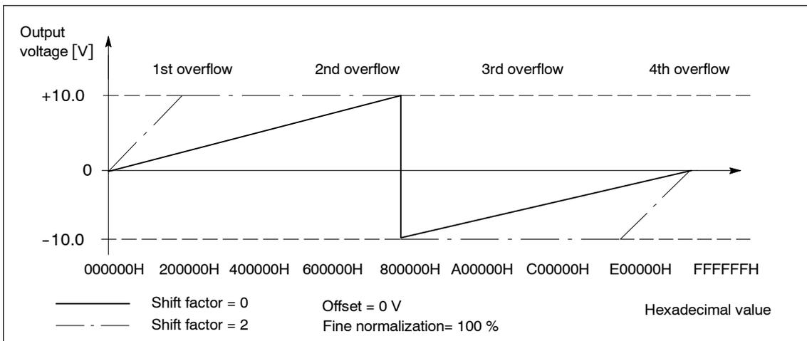
Fig. 6-71 Analog output voltage with overcontrol protection (P0631/P0638 = 1)
