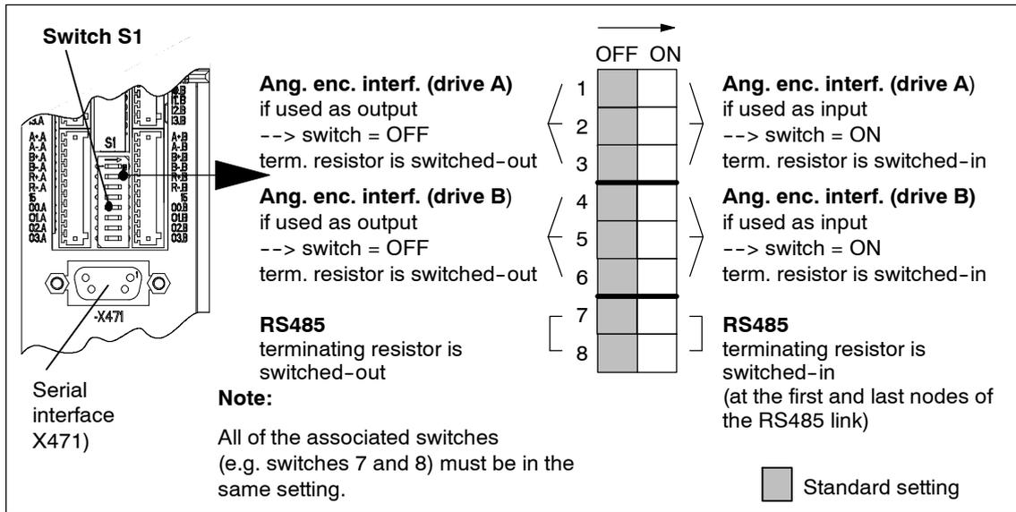
Fig. 1-6 Location and settings of switch S1
