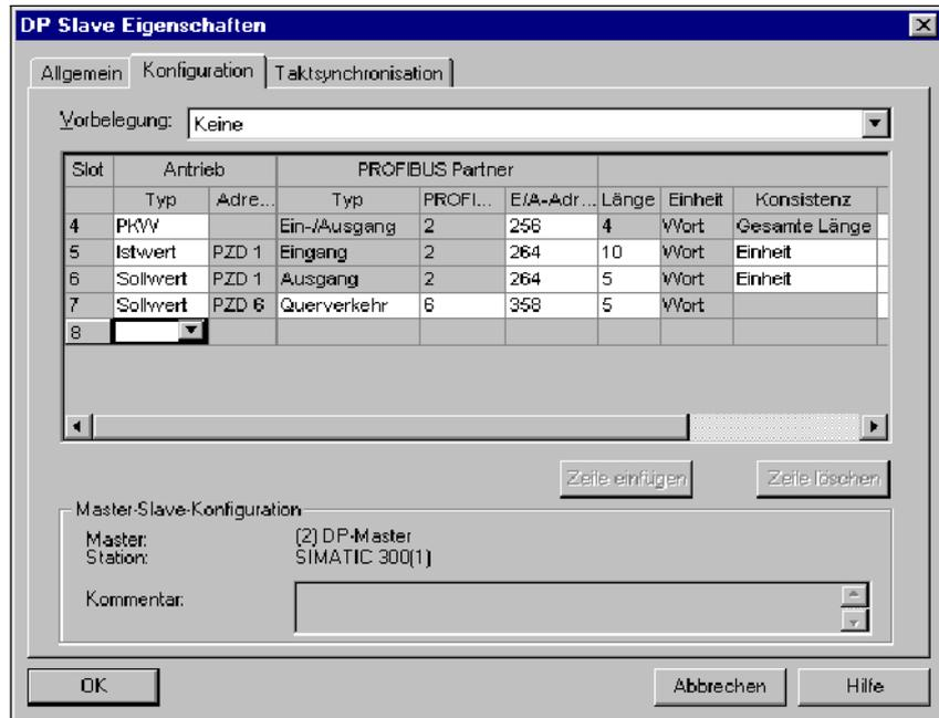
Fig. 5-36 Example, configuring the slave drive for S7
