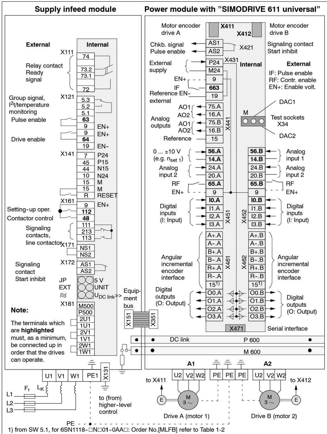
Fig. 2-7 Connection diagram for the control board
