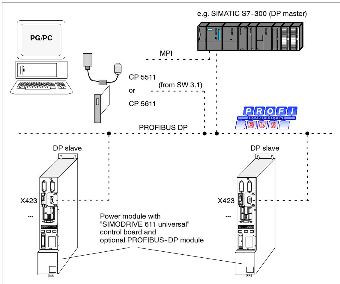
Fig. 2-9 Connection diagram for the optional PROFIBUS-DP module
