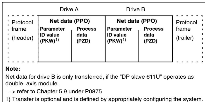
Fig. 5-4 Telegram structure for cyclic data transfer
