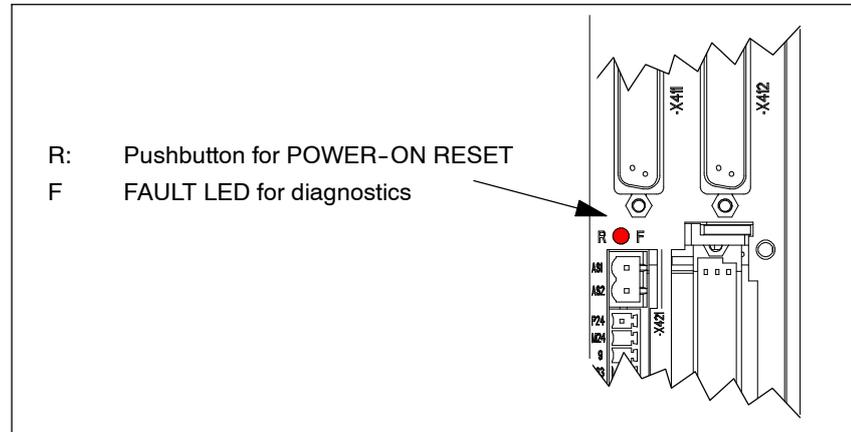
Fig. 7-4 FAULT LED on the front panel of the control board
