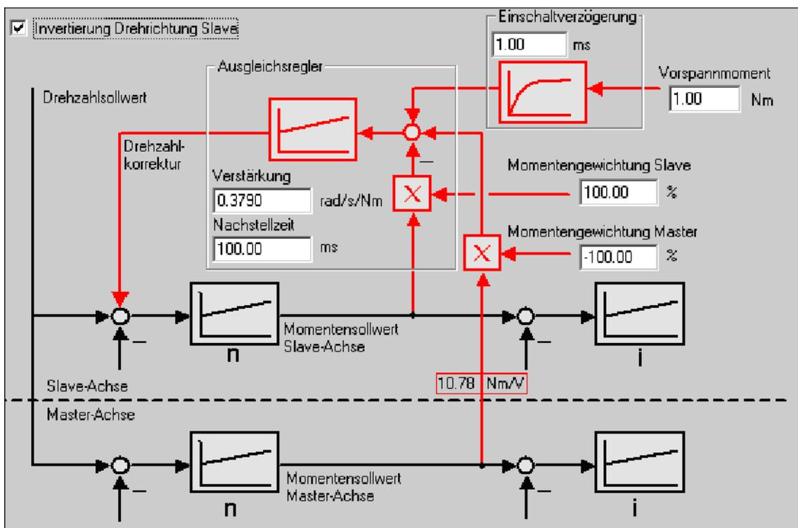
Fig. 6-54 Inverting the direction of rotation, slave axis
