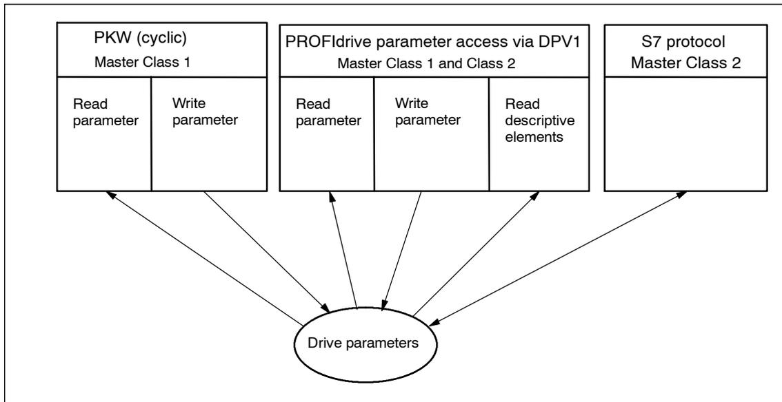
Fig. 5-5 Overview, parameter access operations for PROFIdrive
