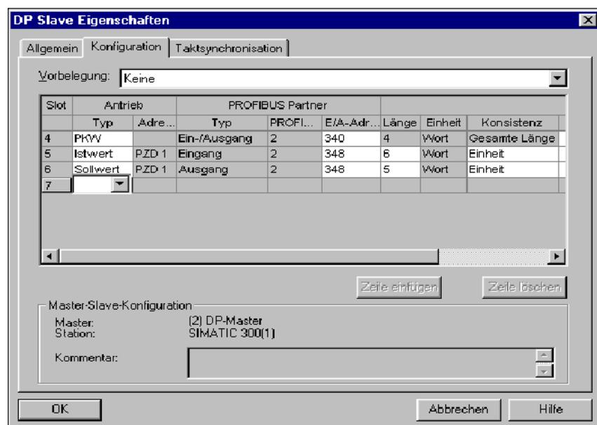
Fig. 6-44 Example, configuring the master drive for S7
