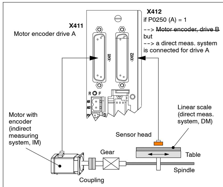
Fig. 4-23 Indirect and direct measuring system for drive A
