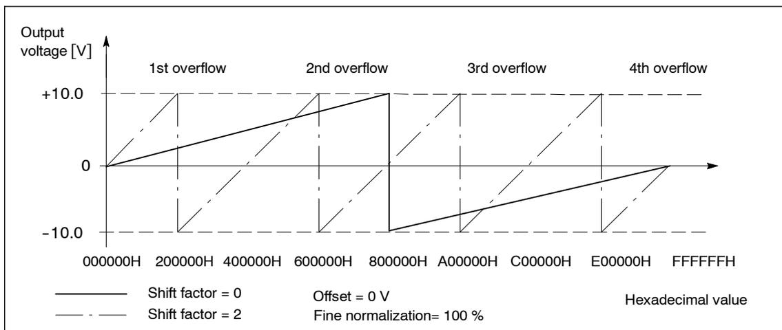
Fig. 6-72 Analog output voltage without overcontrol protection (P0631/P0638 = 0)
