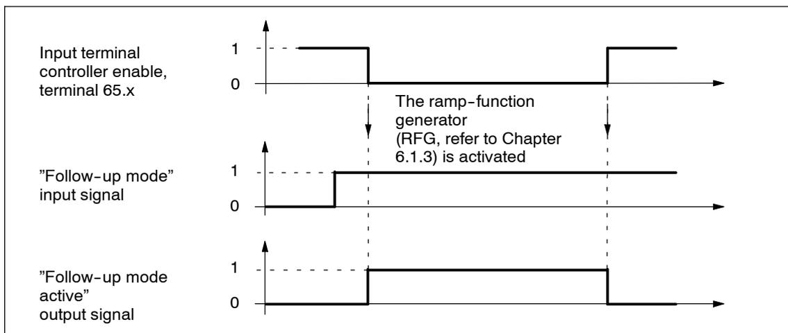
Fig. 6-21 Characteristics (time) in the follow-up mode
