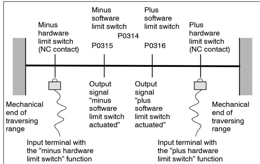
Fig. 6-15 Overview of the limit switch monitoring functions
