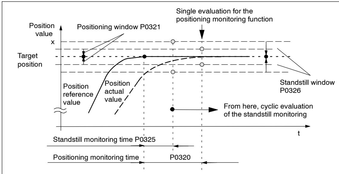
Fig. 6-19 Standstill and positioning monitoring
