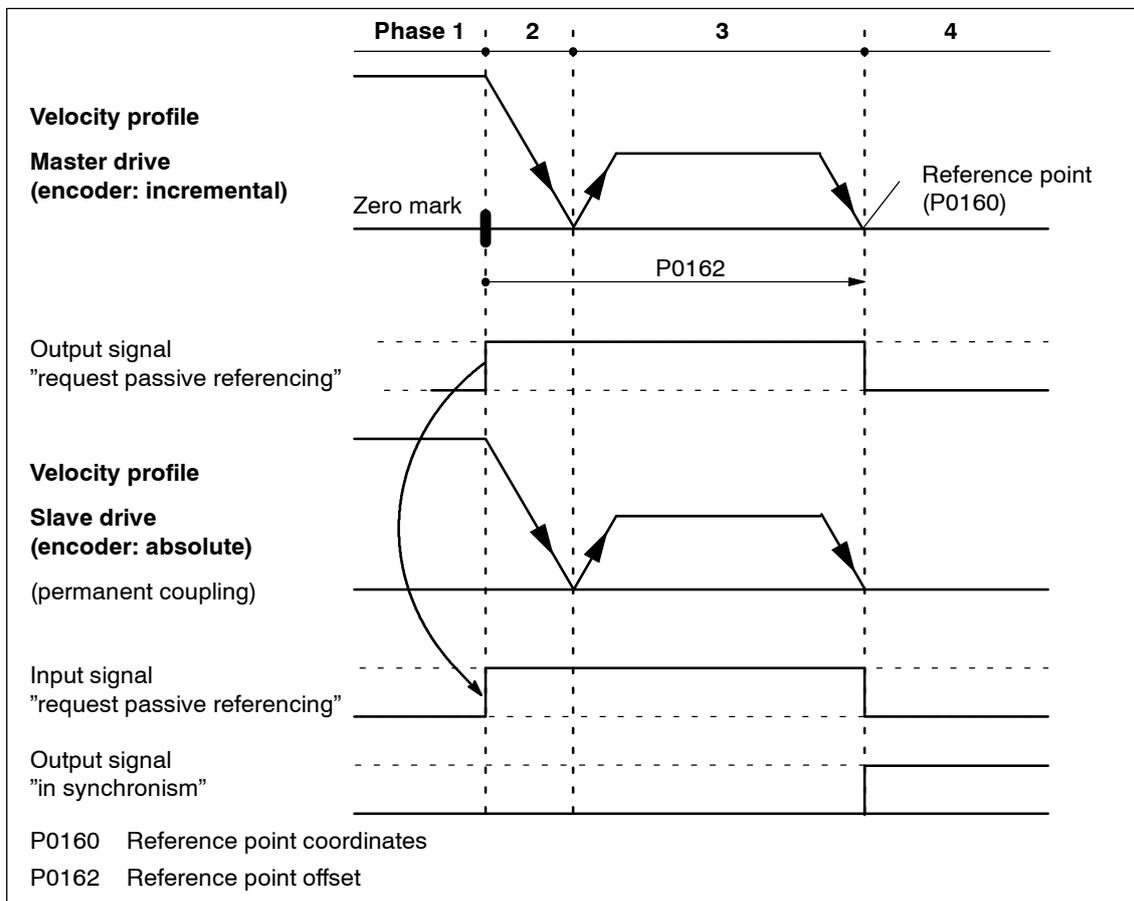
Fig. 6-41 Sequence when passively referencing (master drive with incremental encoder and slave drive with absolute value encoder)
