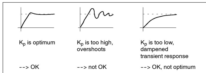
Fig. 4-12 How should the step response be evaluated?
