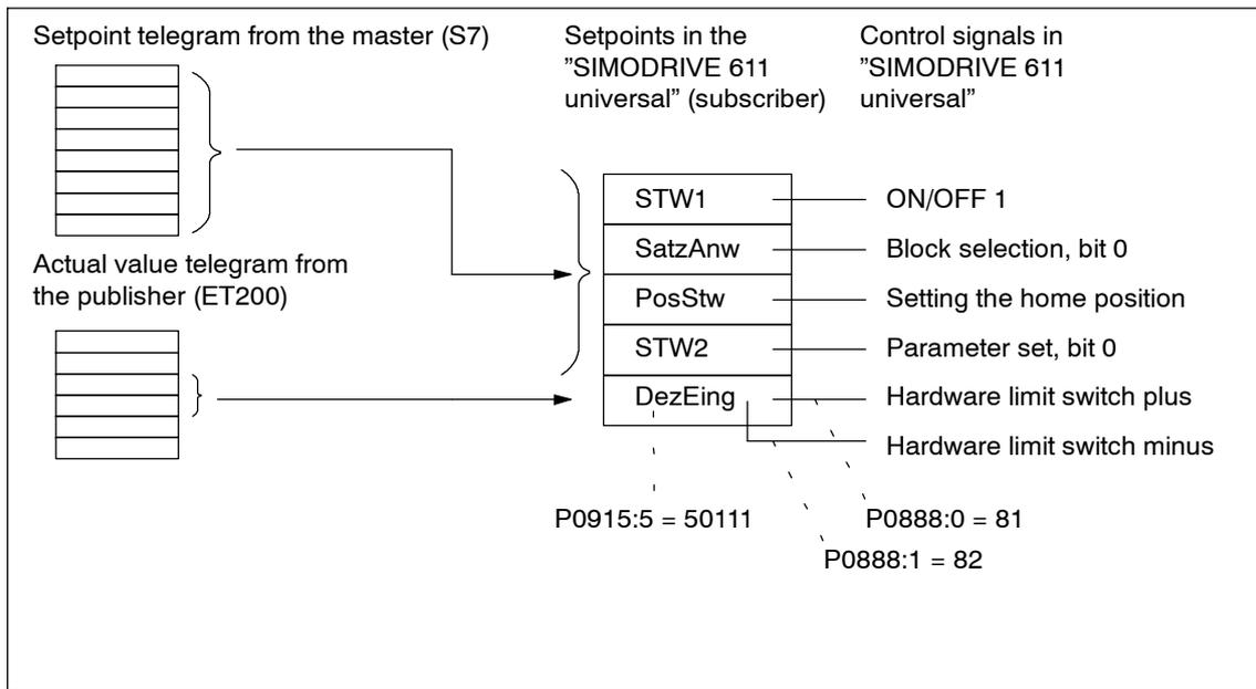
Fig. 5-34 Example, mixed operation for the control signals
