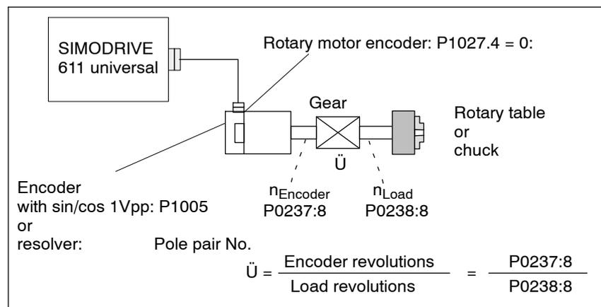
Fig. 6-13 Rotary axis with rotary motor encoder
