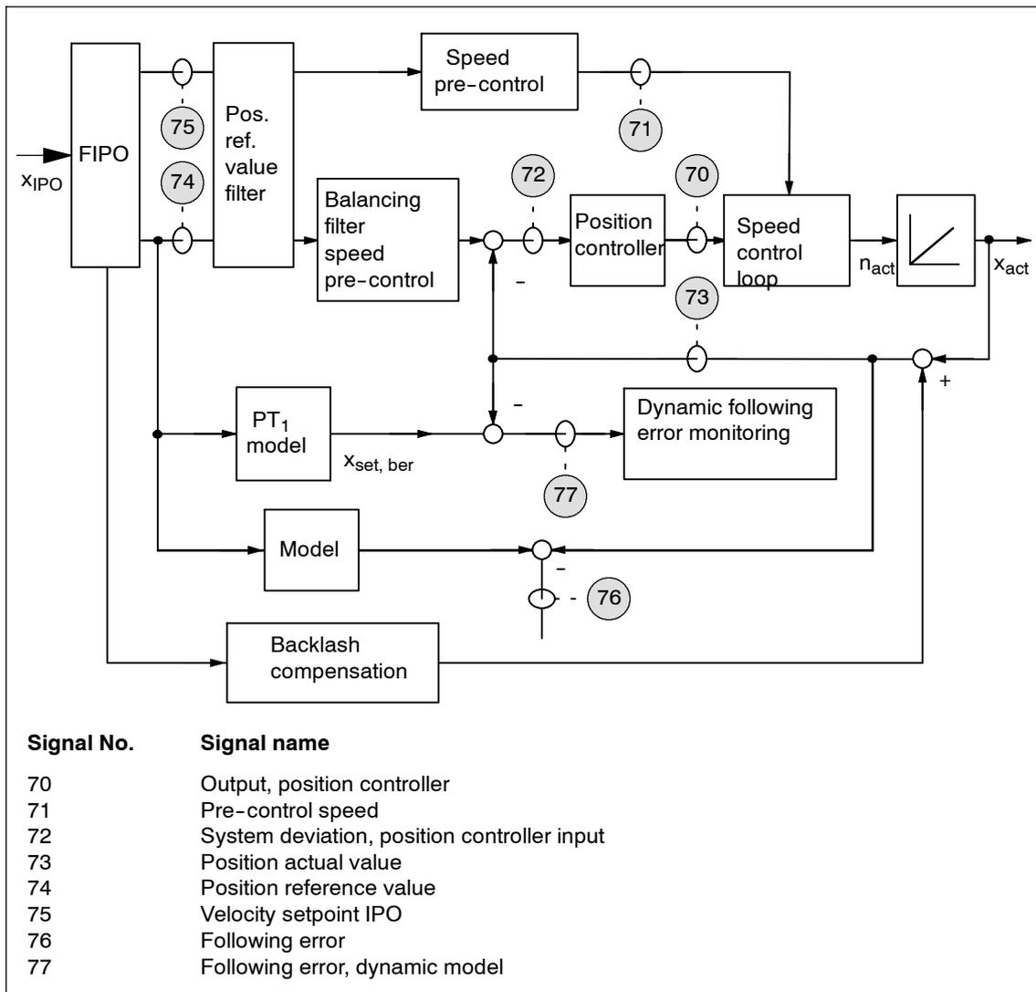
Fig. 6-68 Analog signals for the position control loop
