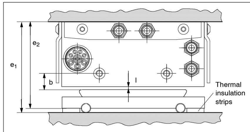
Fig. 4-15 Important dimensions when mounting 1FN1 motors
