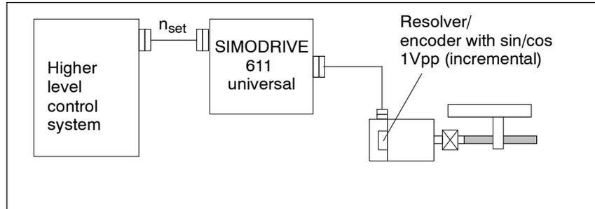
Fig. 6-1 Variable-speed drive
