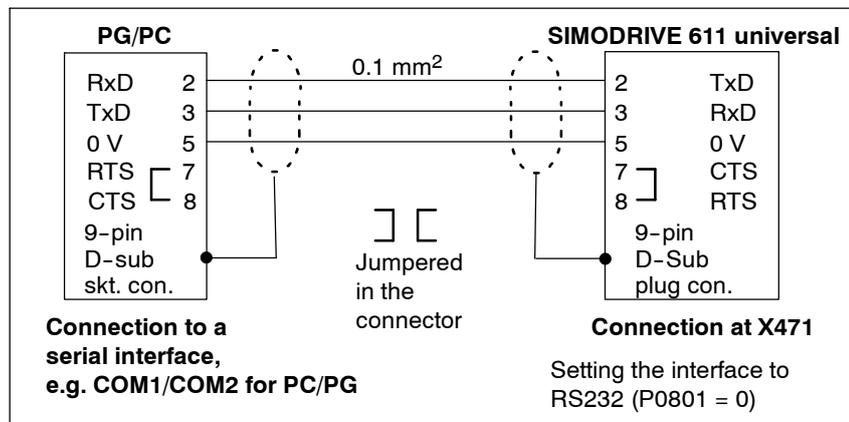
Fig. 2-12 RS232 connecting cable without RTS/CTS lines:
