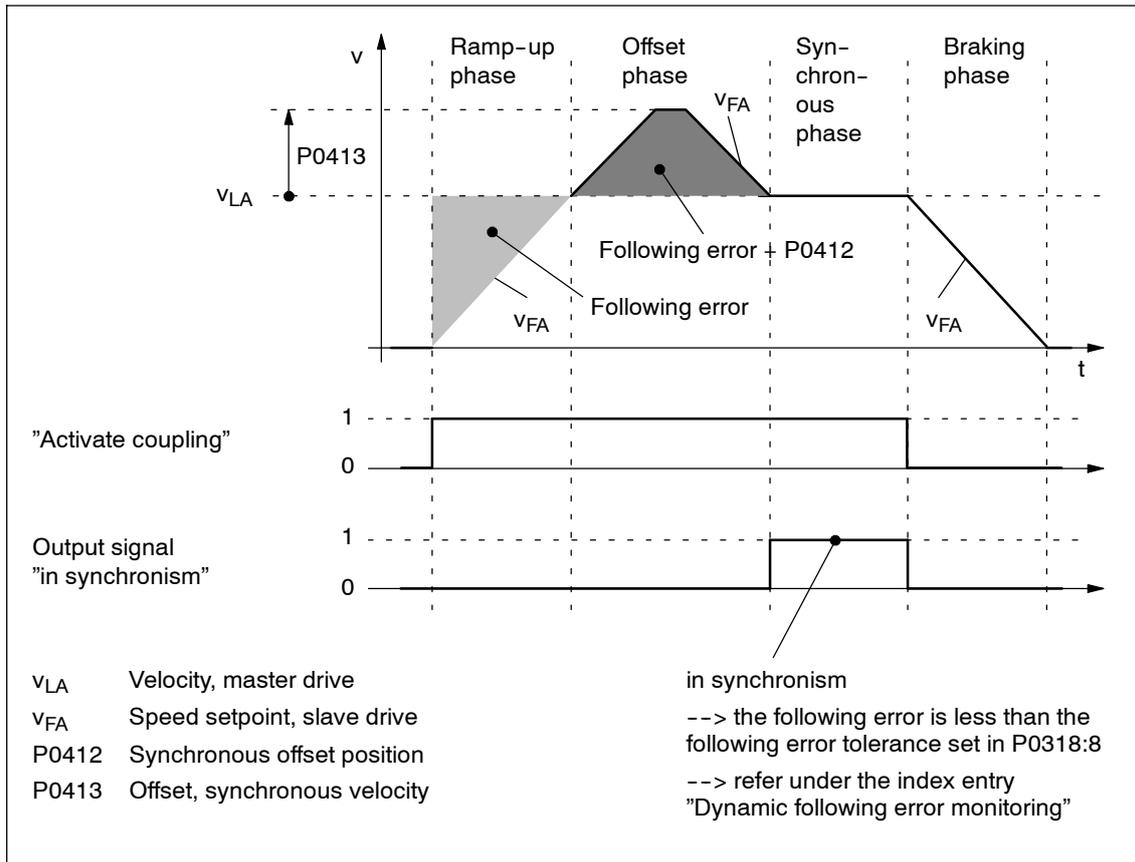
Fig. 6-36 Position synchronism (P0410 = 2 or 4)
