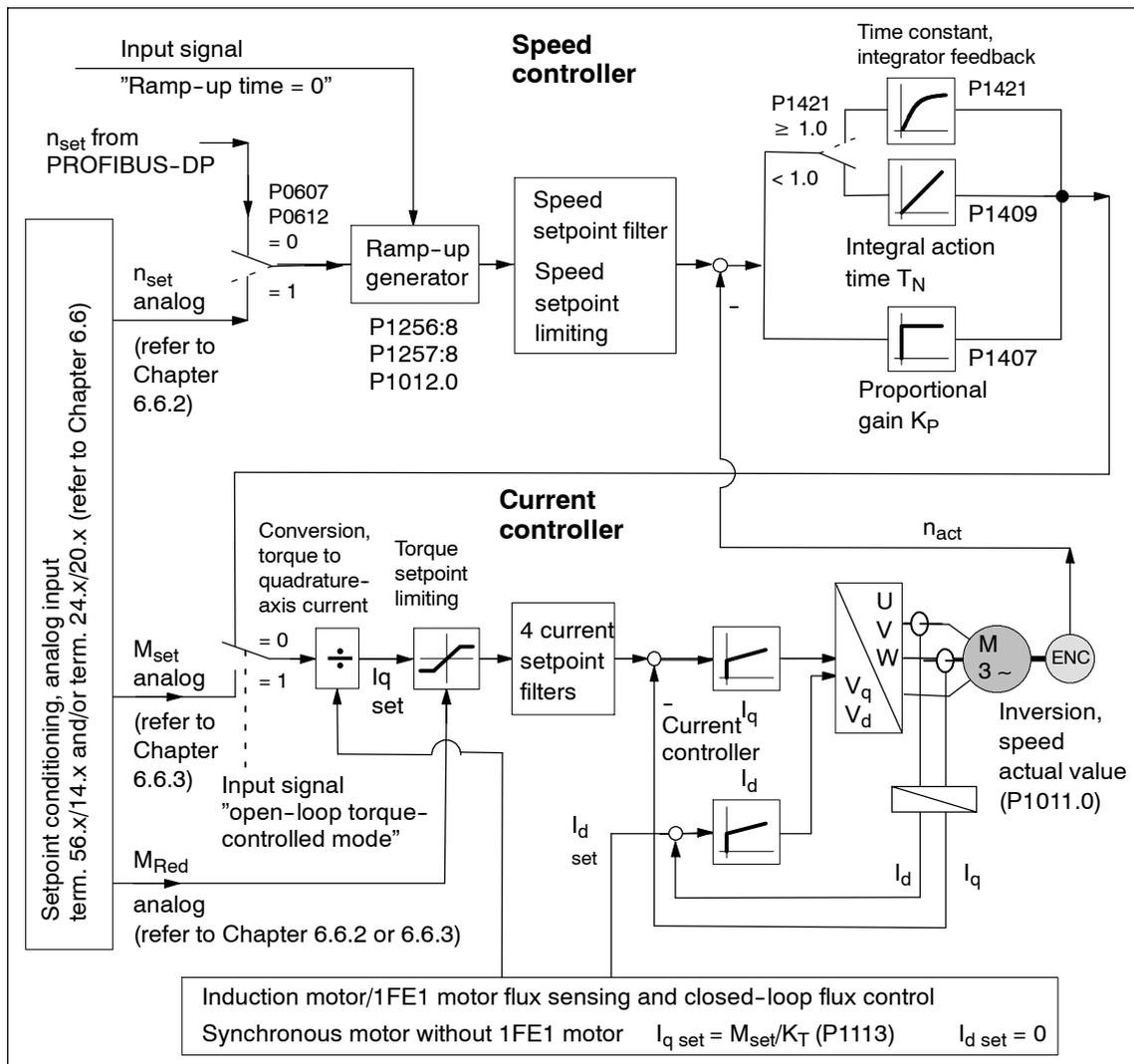
Fig. 6-4 Current and speed control
