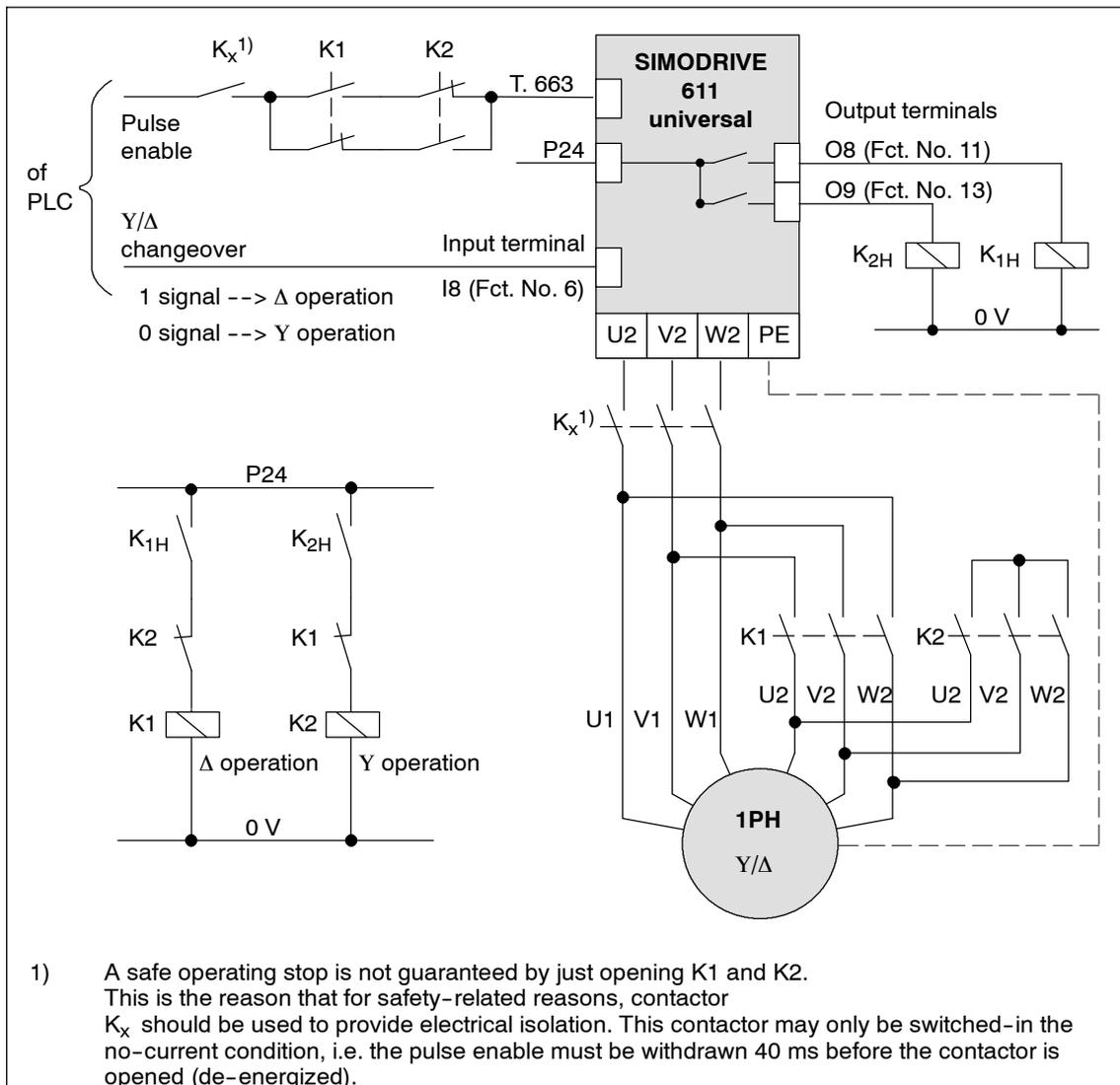
Fig. 6-90 Recommended circuit: Changing over a motor in star/delta operation
