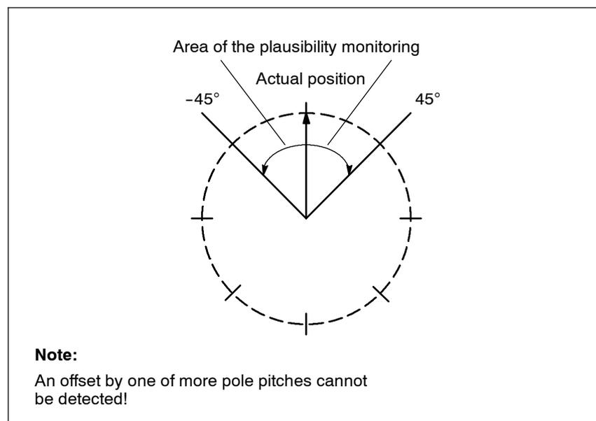
Fig. 6-98 Limits of plausibility monitoring (rotary axis example)
