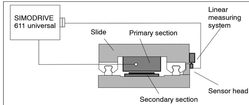
Fig. 6-12 Linear axis with linear motor encoder
