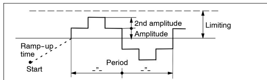
Fig. 7-7 "Staircase" waveform with amplitude > 0 and offset = 0
