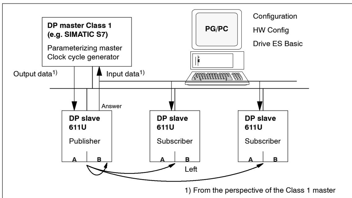
Fig. 5-30 Slave-to-slave communications with the publisher-subscriber module
