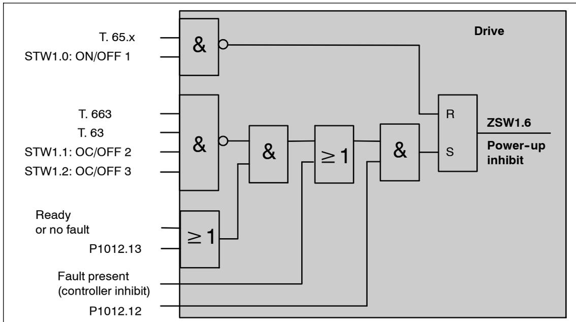
Fig. 5-9 Generating the power-on inhibit
