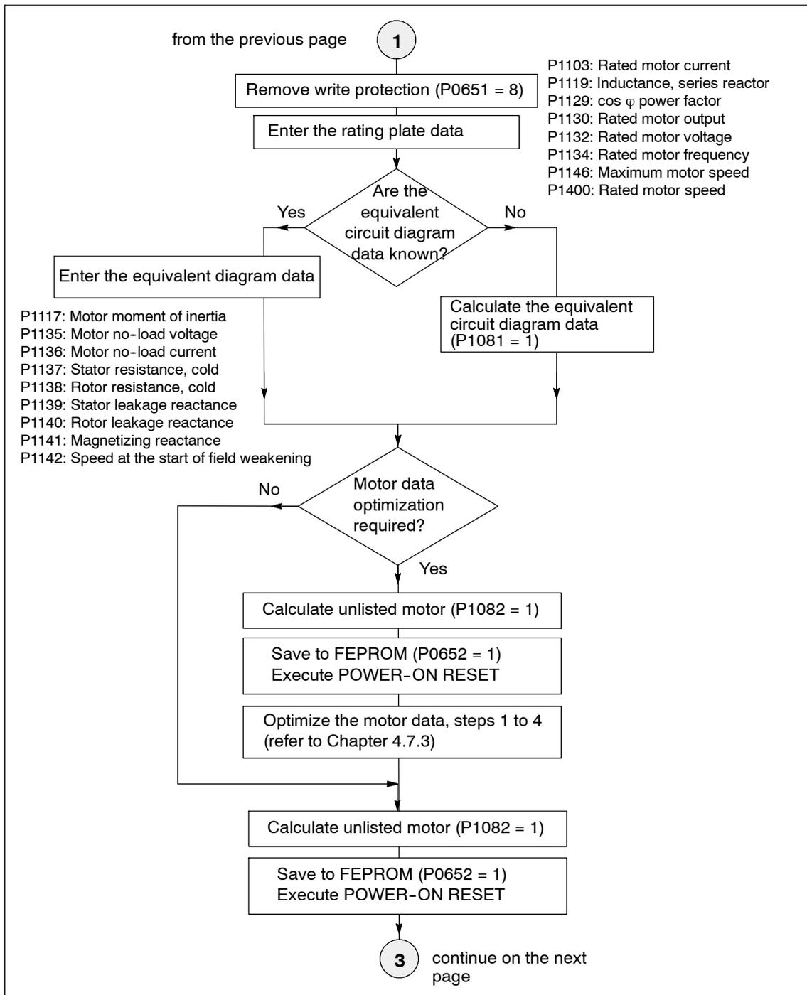
Fig. 4-8 Commissioning induction motors without encoder (Part 2)
