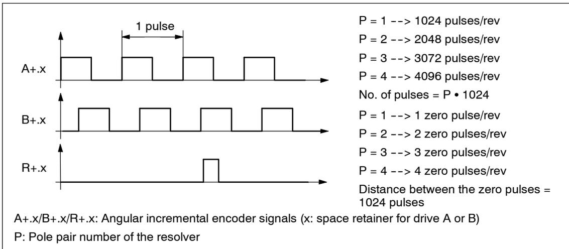
Fig. 6-75 Angular incremental encoder signals for resolvers
