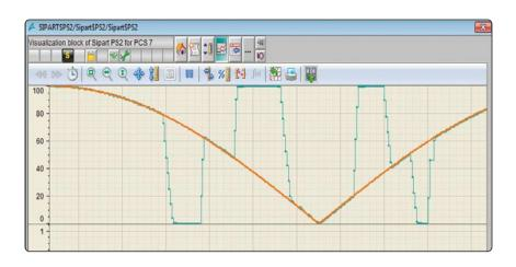
Gain greater transparency about the status of a control valve through display of set point and process value in a single faceplate.
