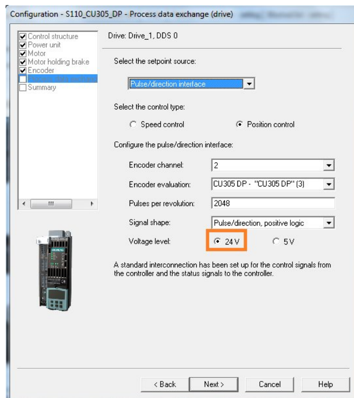
Figure 2. Pulse/direction - interface configuration wizard in Starter
