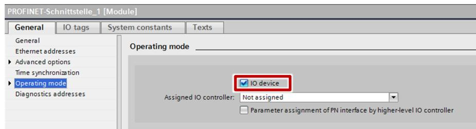
2. You can select the IO controller from the "Assigned IO controller" drop-down list. Then, the networking and the IO system between both devices is displayed in network view.
