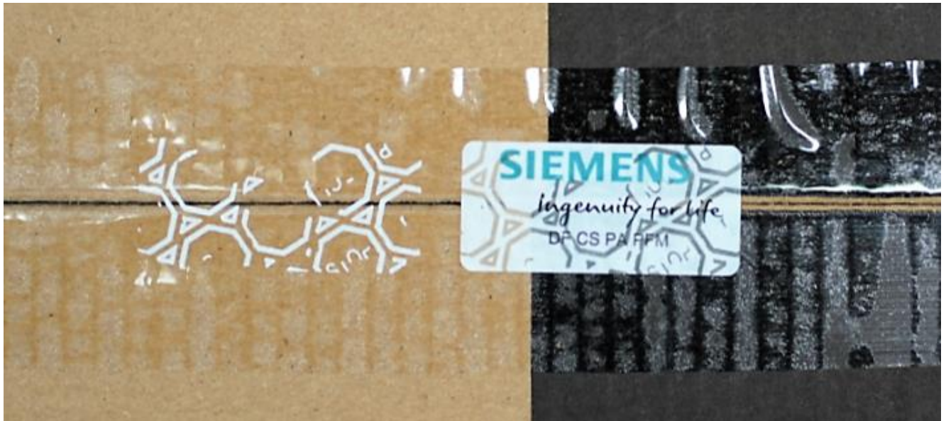
Figure 3: Invalid seal, seal was removed and replaced at a new position
