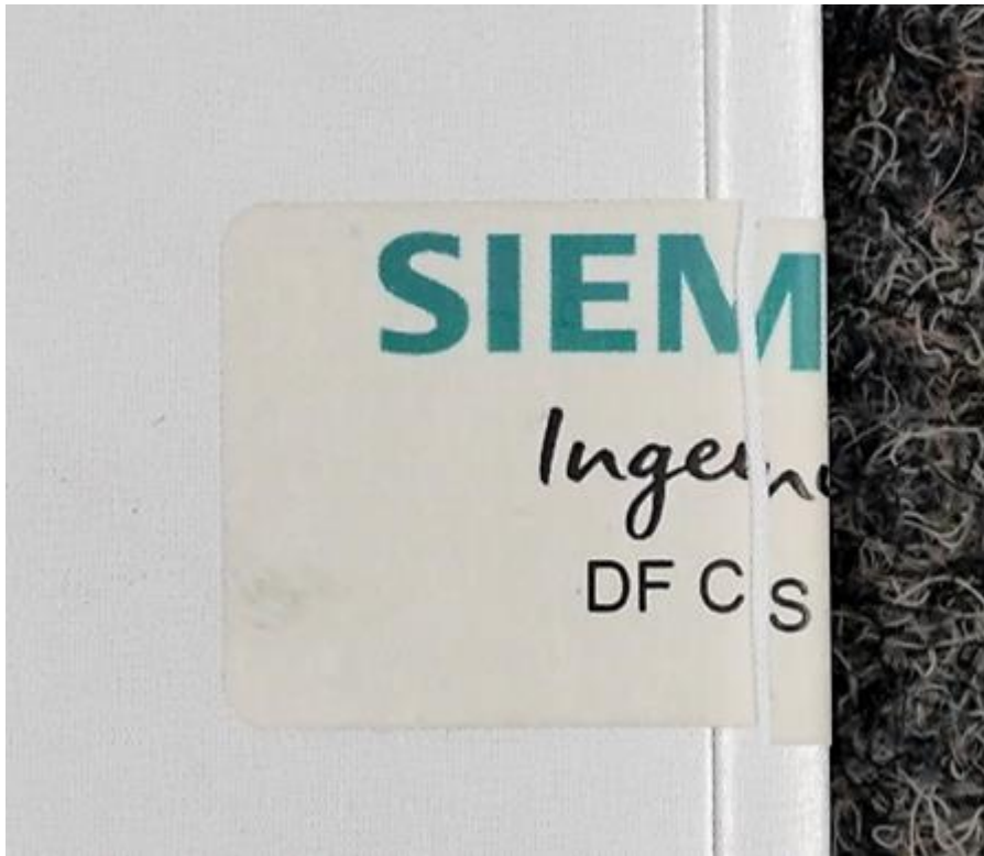
Figure 5: Invalid seal, seal was cut
