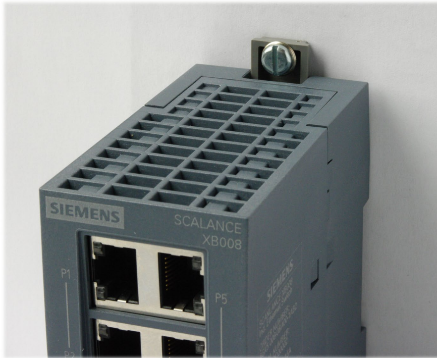
Figure 4-5 Wall mounting of the SCALANCE XB-000
