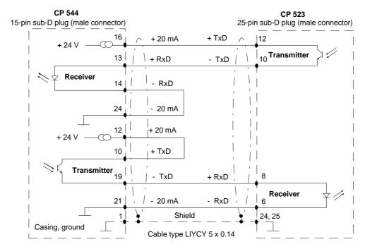
Fig. 10-6 TTY submodule: connecting cable CP 544 - CP 523
