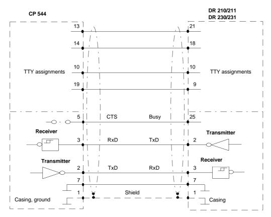
Fig. 10-10 V.24 submodule: connecting cable CP 544 - DR 210/211, DR 230/231
