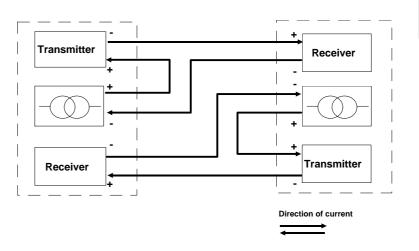
The following Fig. illustrates the typical connections of the current loop signals:
