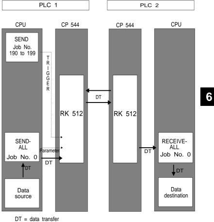
Fig. 6-3 WRITE function of the SEND-DIRECT 190 to 199
