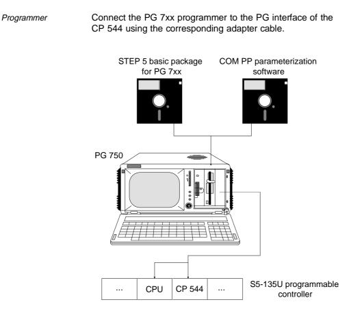
Fig. 9-2 Use of programmer for point-to-point link
