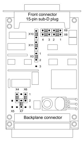
Fig. 10-1 RS422-A/485 submodule: jumper settings when supplied
