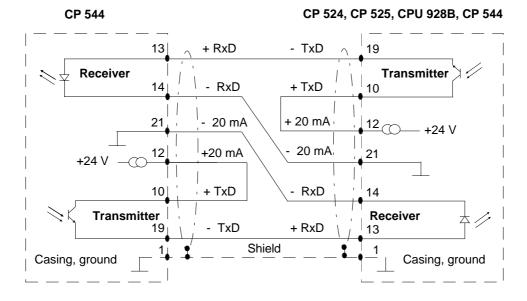
Fig. 10-4 TTY submodule: connecting cable CP 544 - CP 525, CP 524, CPU 928B, CP 544
