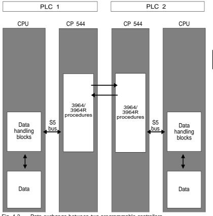
Fig. 4-2 Data exchange between two programmable controllers
