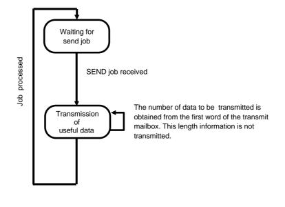
Fig. 5-8 Transmission sequence in mode 3
