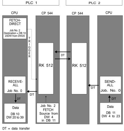
Fig. 9-4 Structure of a FETCH job from DB to DB
