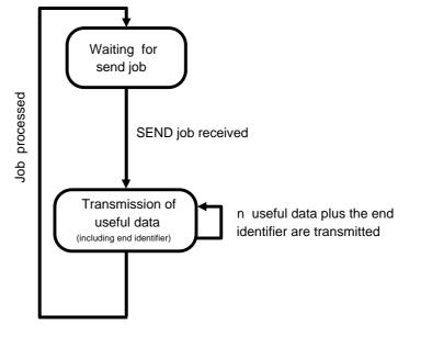
Fig. 5-6 Transmission sequence in mode 2
