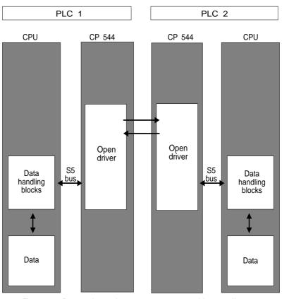
The following Fig. shows the data exchange sequence between two programmable controllers.
