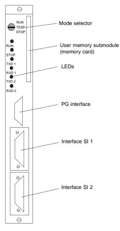
Fig. 1-2 Front panel of CP 544
