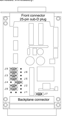
Fig. 10-8 V.24 submodule: jumper settings when supplied
