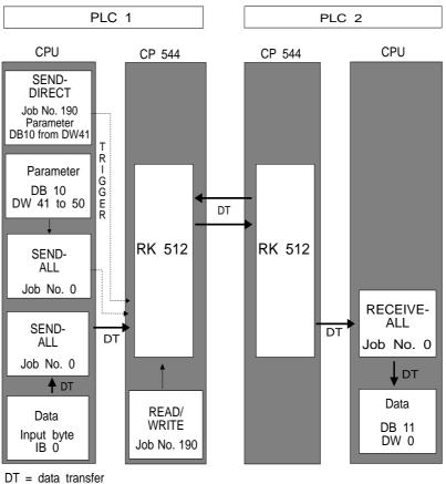
Fig. 9-6 Structure of a PSEUDO-WRITE job
