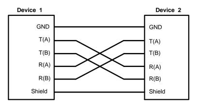
Fig. 1-3 RS422/485 submodule: full-duplex mode
