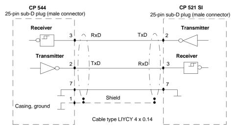
Fig. 10-12 V.24 submodule: connecting cable CP 544 - CP 321 SI
