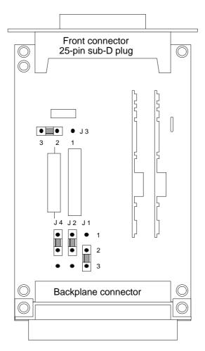
Fig. 10-3 TTY module: jumper settings when supplied
