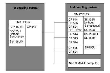
Fig. 3-1 Possible coupling partners with RK 512 data transmission
