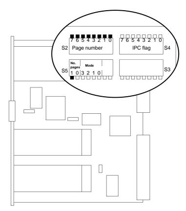
Fig. 2-2 Positions of switches on the module, and delivered state
