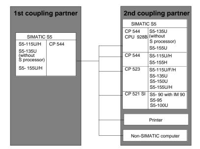
Fig. 5-1 Possible coupling partners for data transmission with open driver
