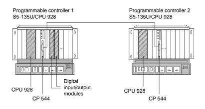
Fig. 9-1 System configuration in application example
