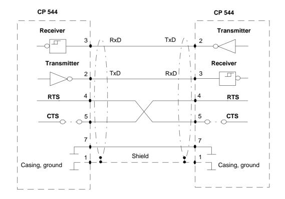
Fig. 10-13 Example of a connecting cable CP 544 - CP 544 for RTS/CTS flow control
