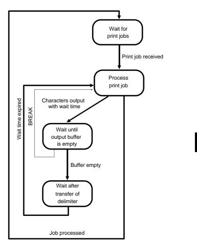
Fig. 5-10 Transmission sequence in mode 4
