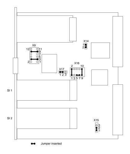
Fig. 2-4 Jumper settings on the CP 544 when delivered
