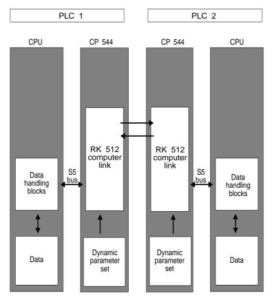
Fig. 3-2 Data exchange between two programmable controllers
