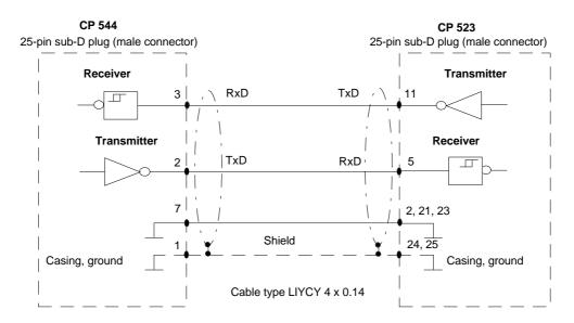
Fig. 10-11 V.24 submodule: connecting cable CP 544 - CP 523
