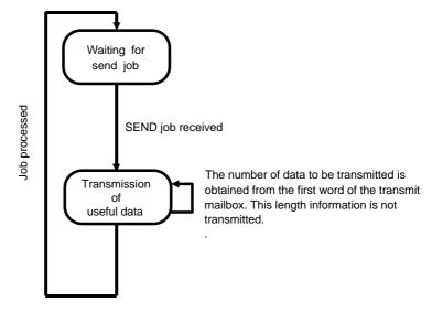
Fig. 5-4 Transmission sequence in mode 1
