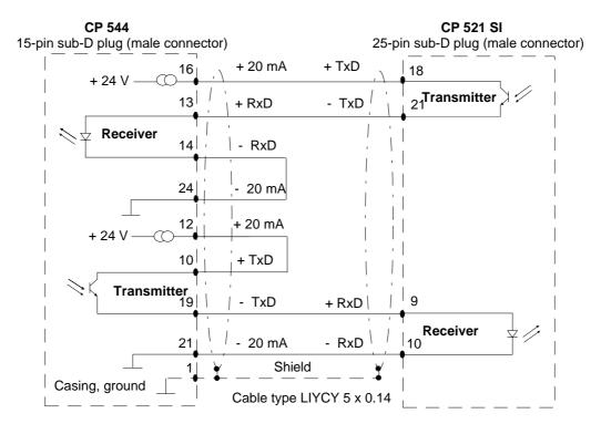
Fig. 10-7 TTY submodule: connecting cable CP 544 - CP 521 SI
