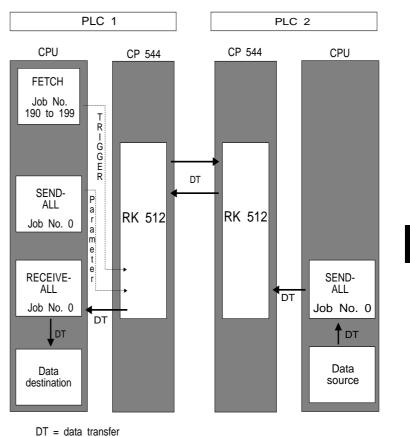
Fig. 6-2 READ function of the SEND-DIRECT 190 to 199
