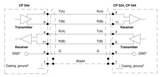
Fig. 10-2 RS422-A/485 submodule: connecting cable CP 544 - CP 524, CP 544
