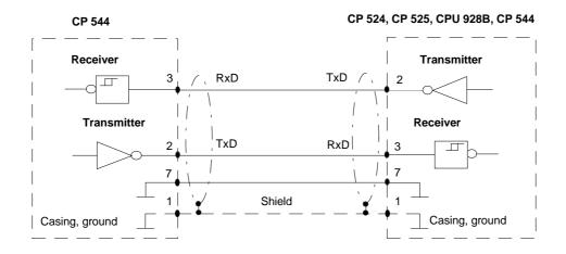
Fig. 10-9 V.24 submodule: connecting cable CP 544 - CP 525, CP 524, CPU 928B, CP 544
