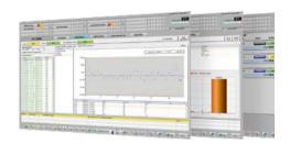
Operator control and monitoring system for optimizing the analyzer landscape in new and existing plants. PC-based system for monitoring, testing and management of gas analyzers in subsystems or complete plants.
